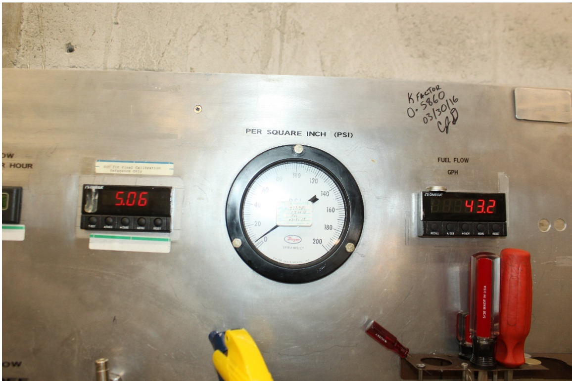
Figure 4: View Depicting the Test Bench Values during the Low Boost Flow Test.
