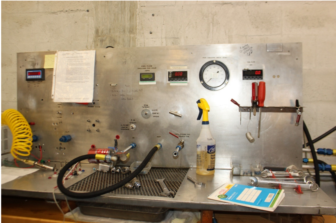
Figure 3: View of the Auxiliary Pump Installed on the Test Bench
