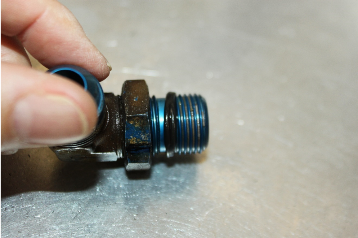
Figure 5: View of the Damaged Packing or O-Ring on the Outlet Fitting.
