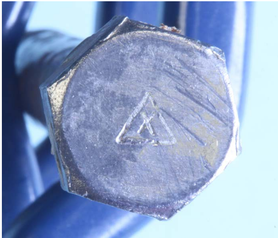
Figure 2: Bolt head with triangle and "X" inscription.
