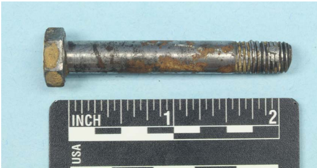
Figure 1: Torque link bolt as received.
