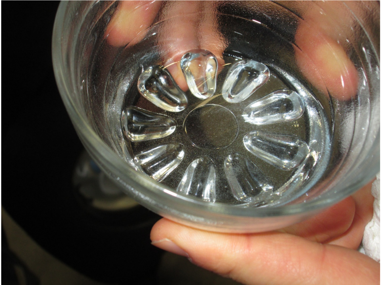
Figure 4: Fuel Sample from Left Engine
