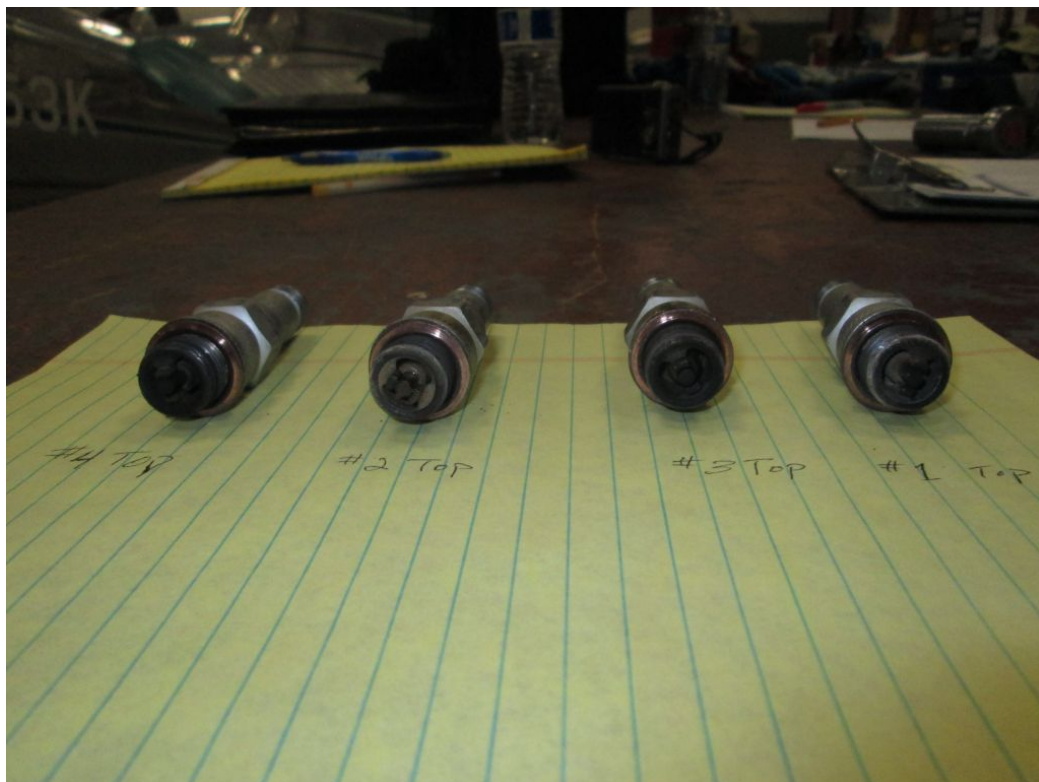
Figure 6: Right Engine Top Spark Plugs
