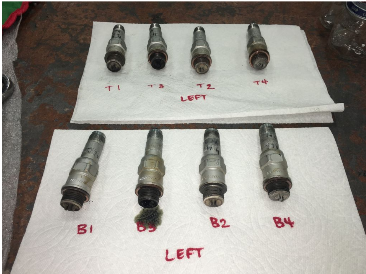
Figure 2: Spark Plugs from Left Engine
