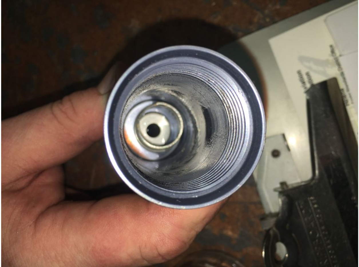
Figure 3: Fuel Filter from Left Engine
