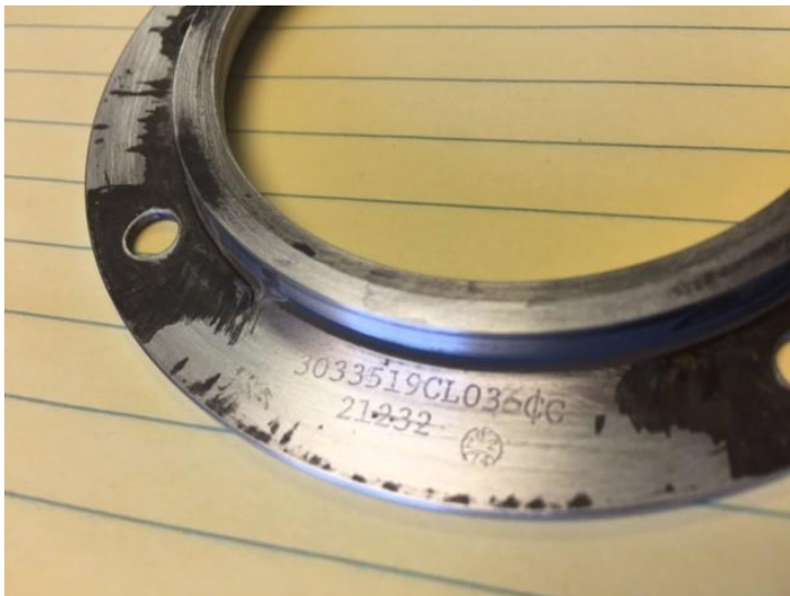
Photo 8: Image of Valve Seat Submitted to Investigation Team by Prime Turbines
