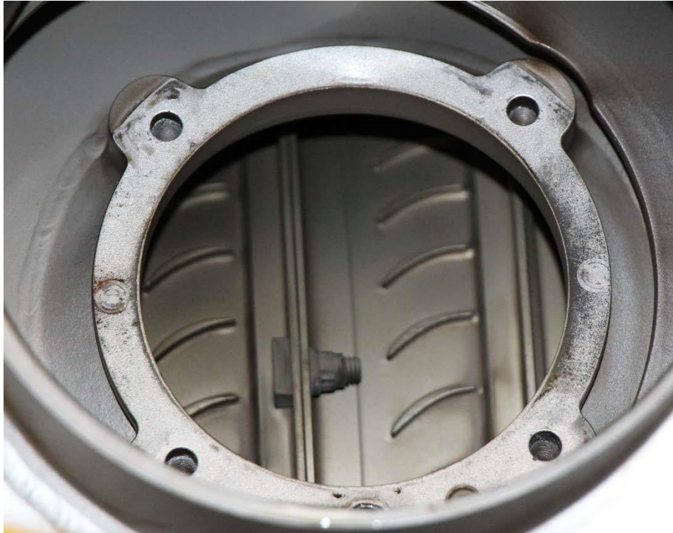
Photo 7: Black Residue at Valve Mating Surface
