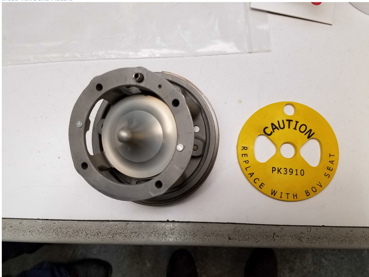
Photo 3: Bleed Valve and Placard
