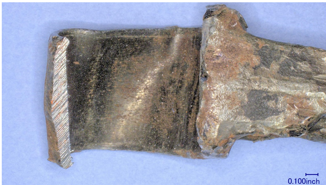
Figure 7 – The pin side of #5 connecting rod, after sectioning the fractured bore half away.
