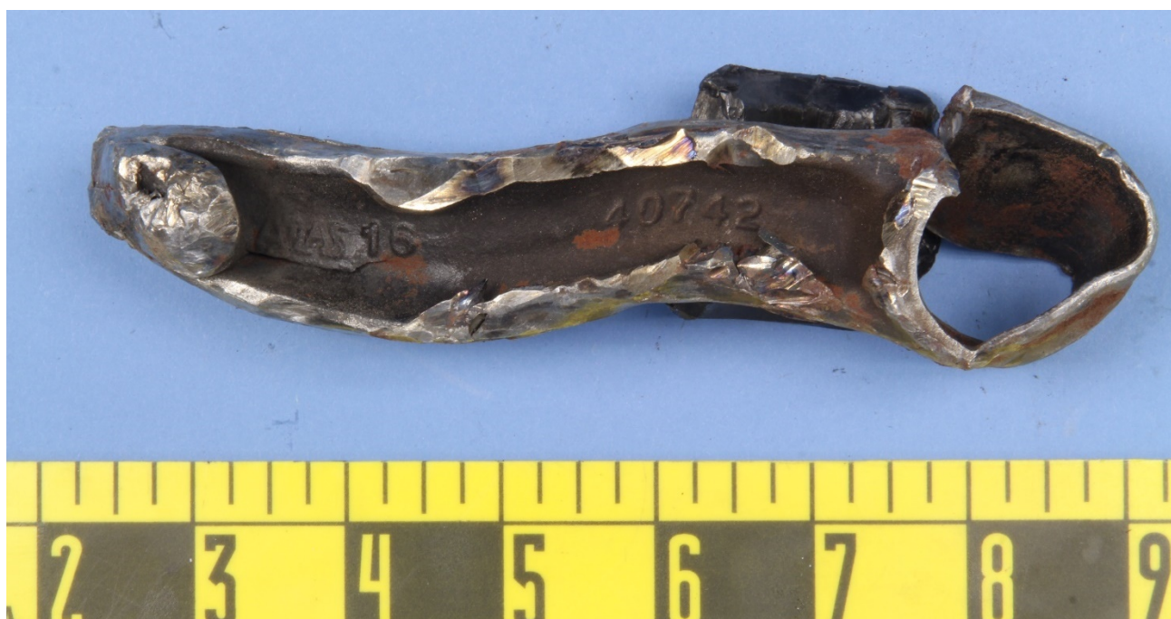
Figure 4 – The web and camshaft bearing of the #5 connecting rod, as received.
