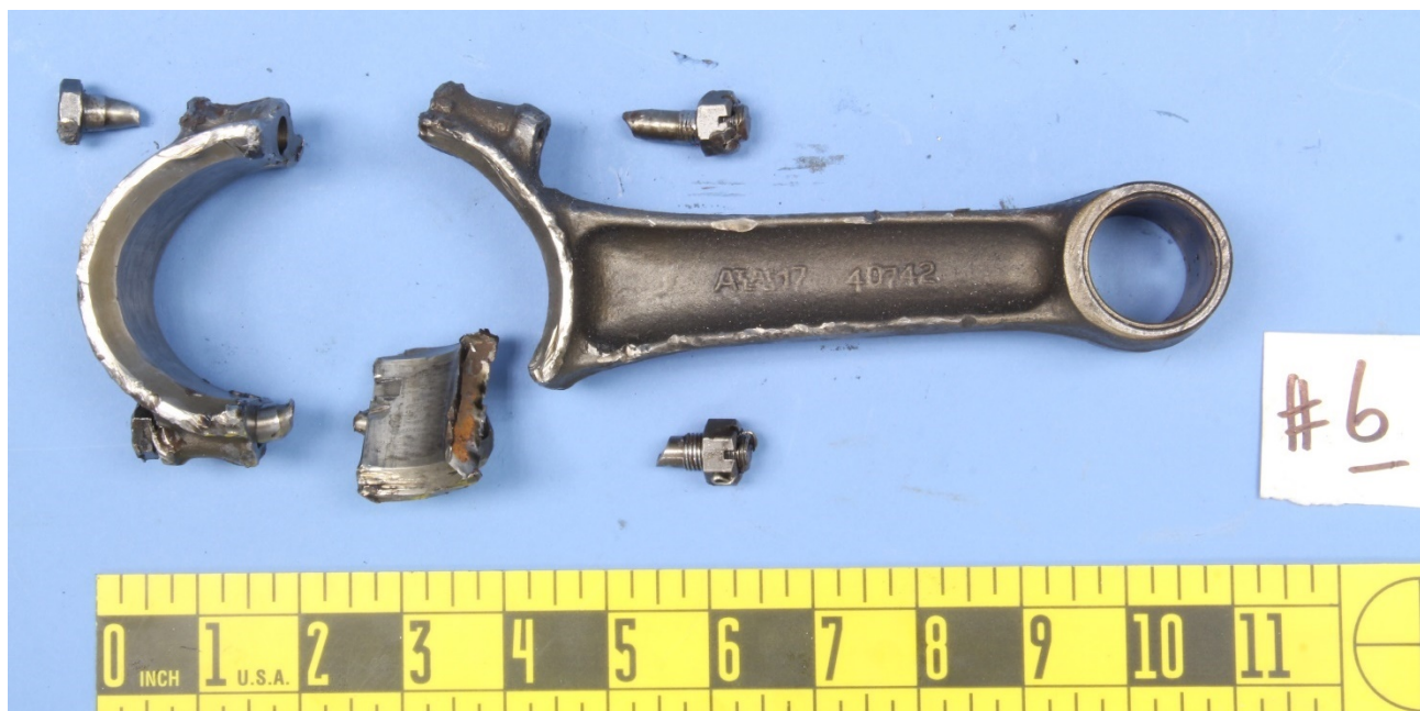
Figure 17 – The received pieces of the #6 connecting rod, cap, and bolts.
