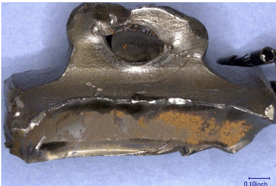
Figure 23 – The fracture surface of the #5 connecting rod pin bore near the yoke neck, which mated with the fracture surface in Figure 22.
