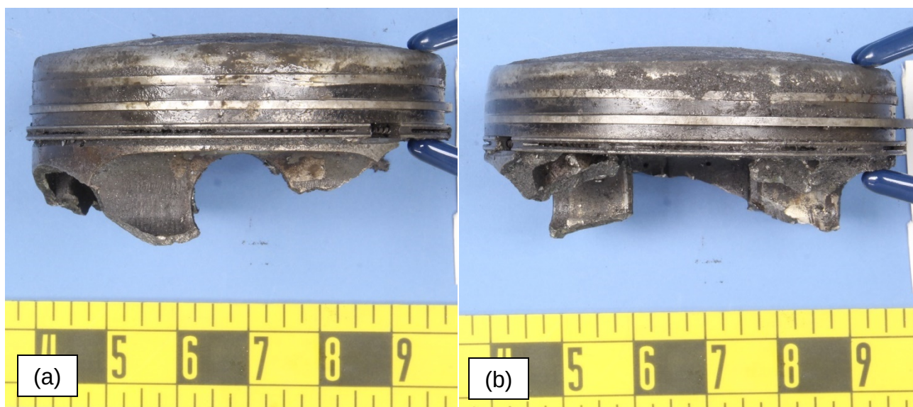
Figure 14 – The sides of the #5 piston, showing the damage about the pin boss from (a) the pin boss side and (b) rotated 90° from Figure 14a.
