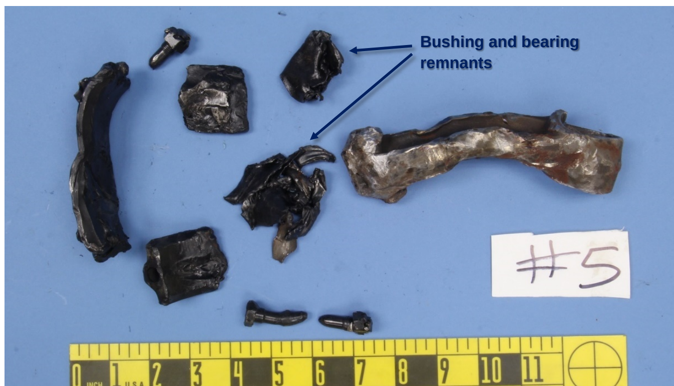
Figure 2 – The received pieces of the #5 connecting rod, cap, and bolts.
