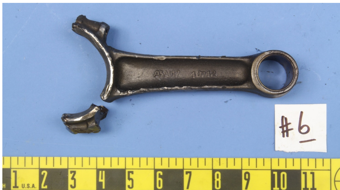
Figure 21 – The pieces of the #6 connecting rod.
