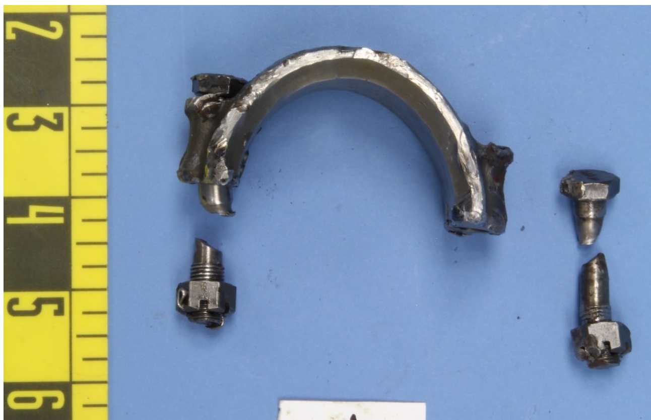
Figure 18 – Closer view of the bolts and cap from the #6 connecting rod, as received.
