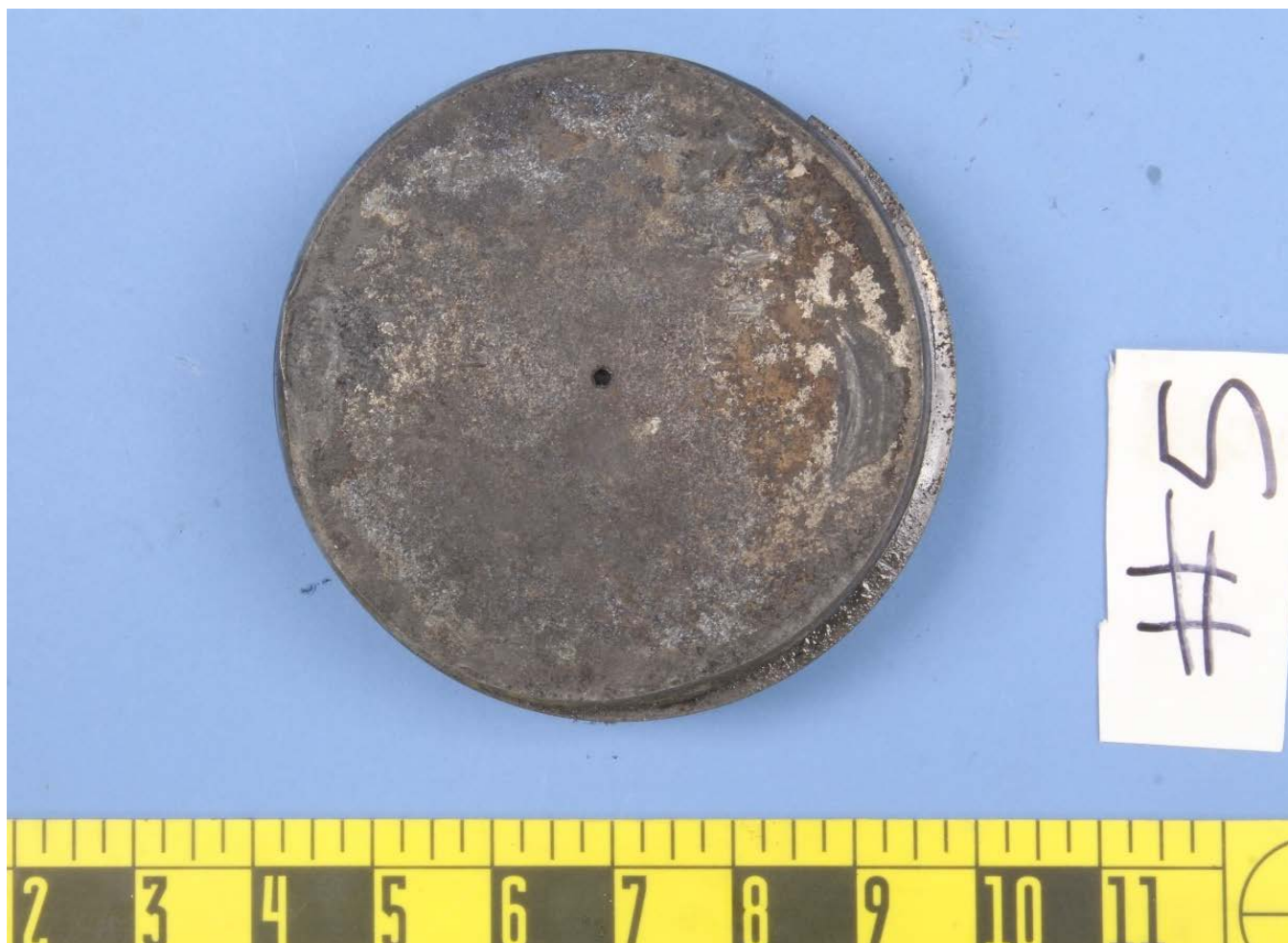
Figure 13 – The top of the #5 piston, which had faced the interior of the #5 cylinder.
