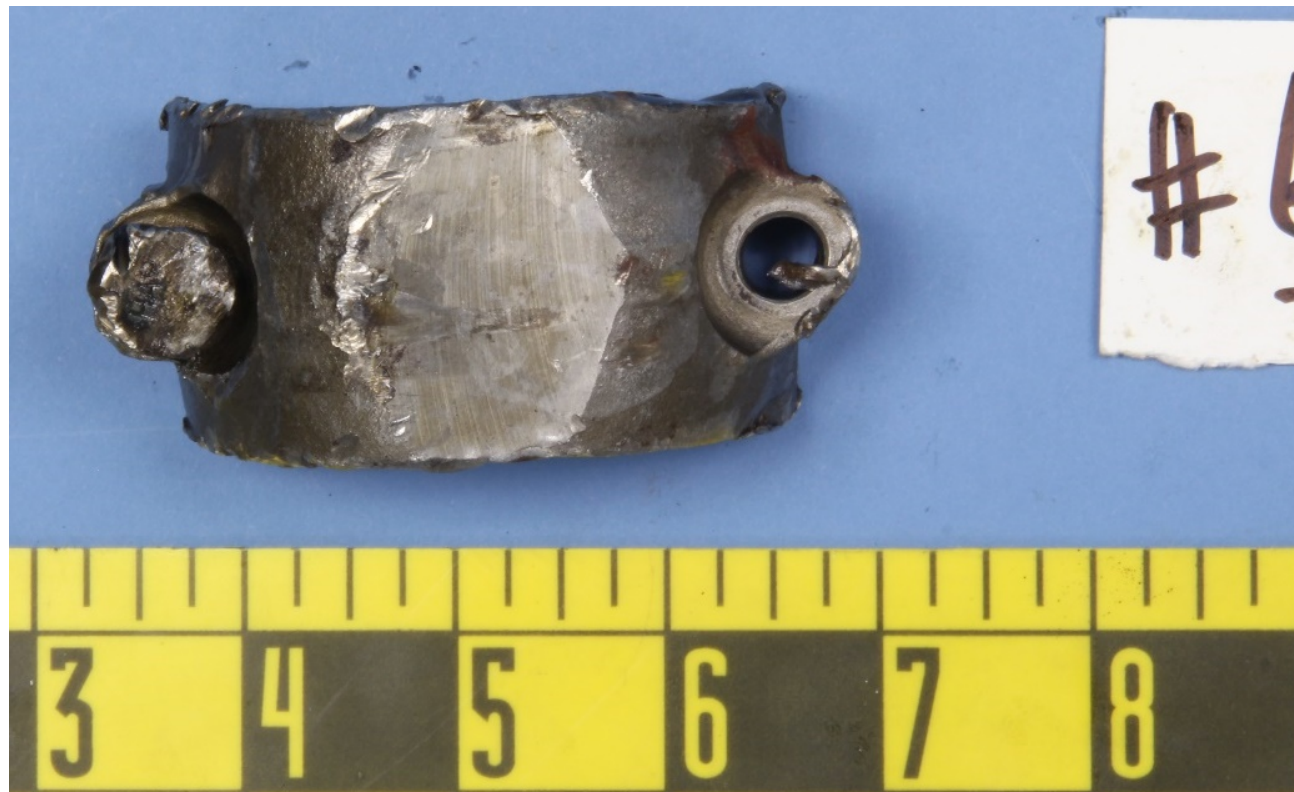
Figure 20 – The outside of the #6 connecting rod cap, showing batter.
