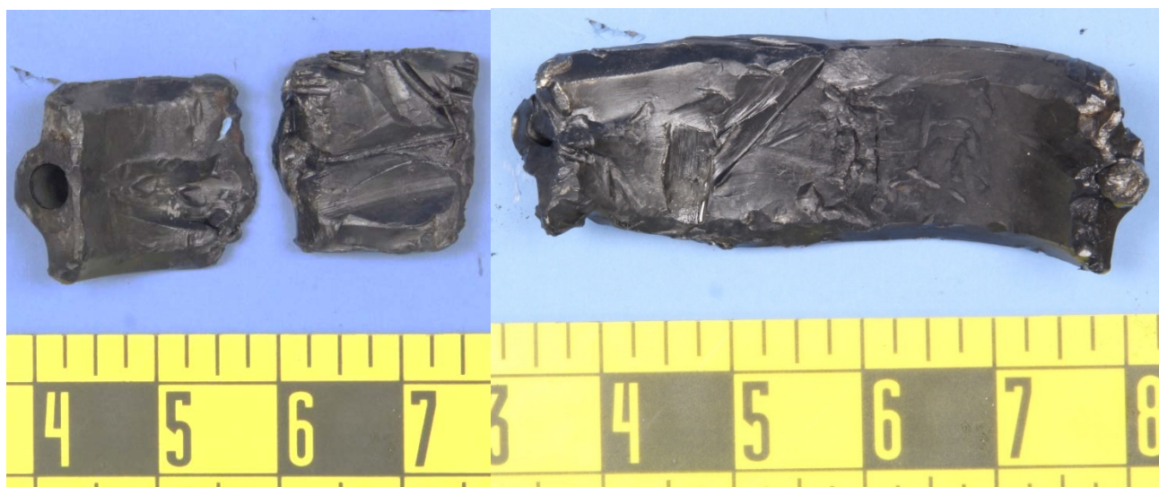
Figure 9 – The inside bearing surfaces of the #5 connecting rod cap.
