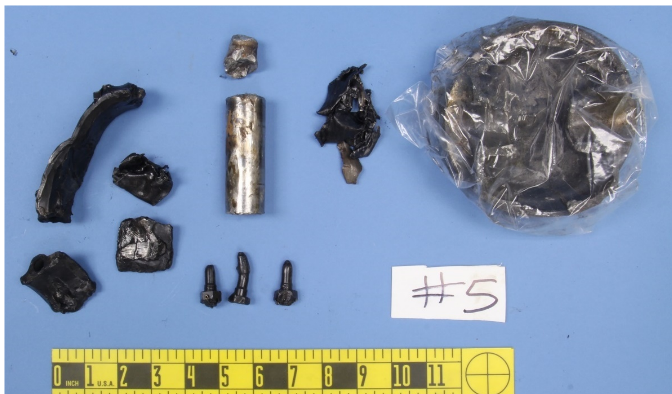
Figure 1 – The components of the #5 engine position (less the connecting rod shaft), as received.
