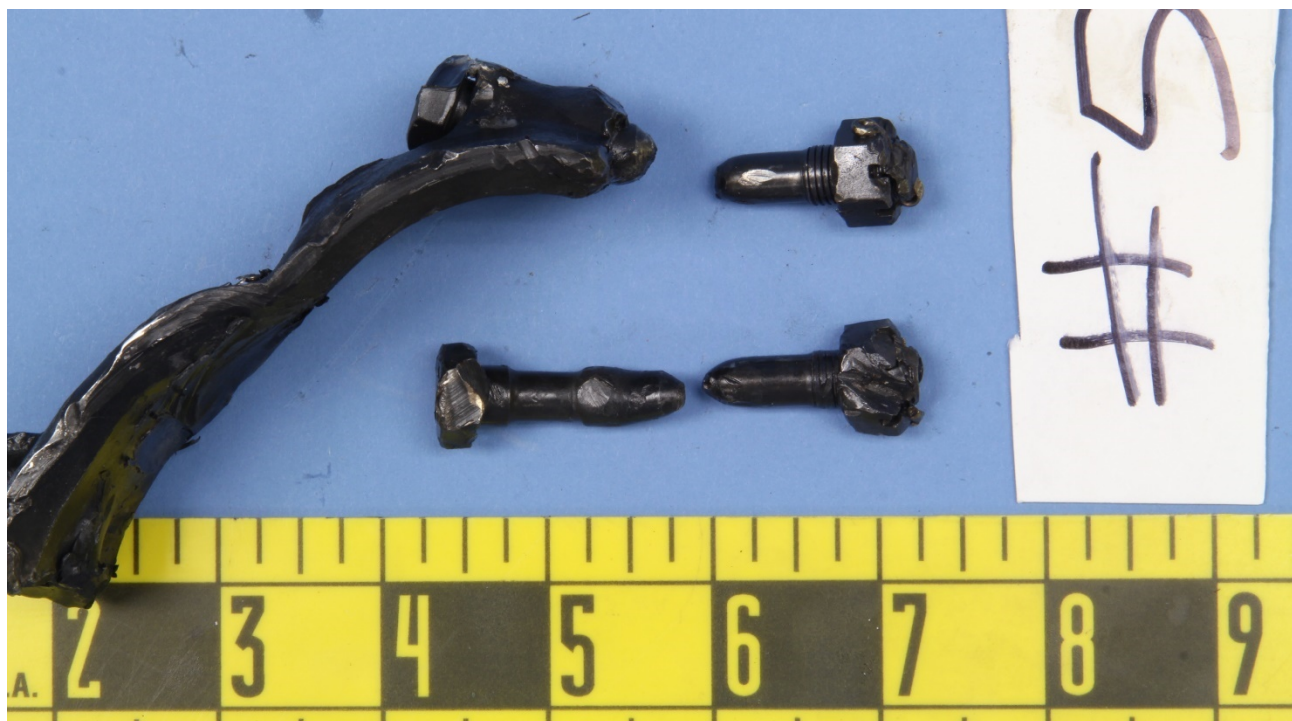
Figure 3 – Closer view of the bolts from the #5 connecting rod, as received.
