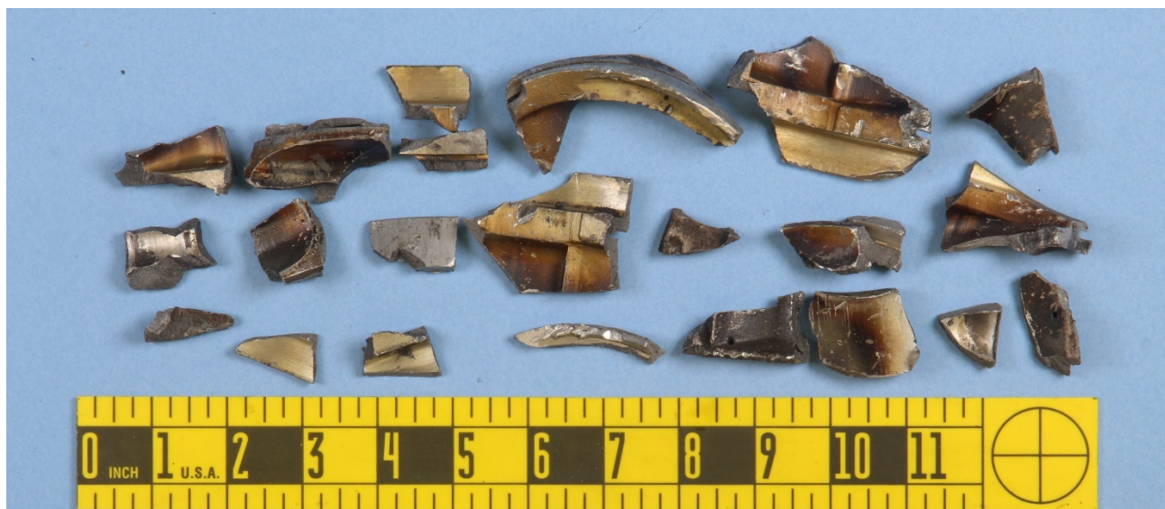
Figure 15 – The miscellaneous piston pieces from the #5 piston.
