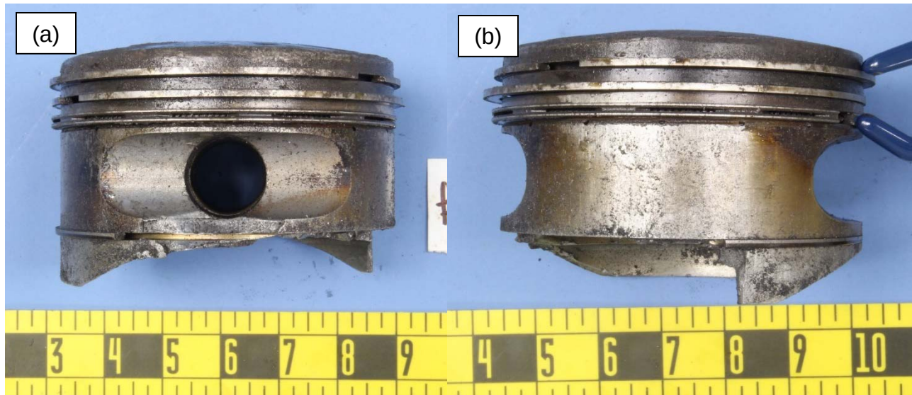
Figure 27 – The #6 piston viewed from (a) the pin boss side and (b) rotated 90° from Figure 27a.
