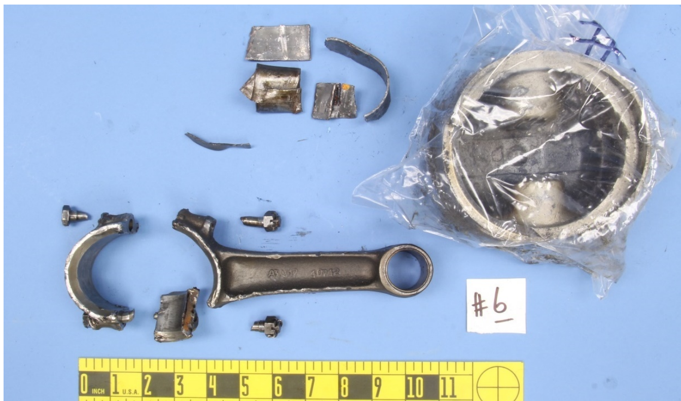
Figure 16 – The components of the #6 engine position, as received.
