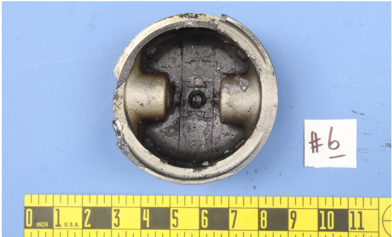
Figure 25 – The underside of the #6 piston.
