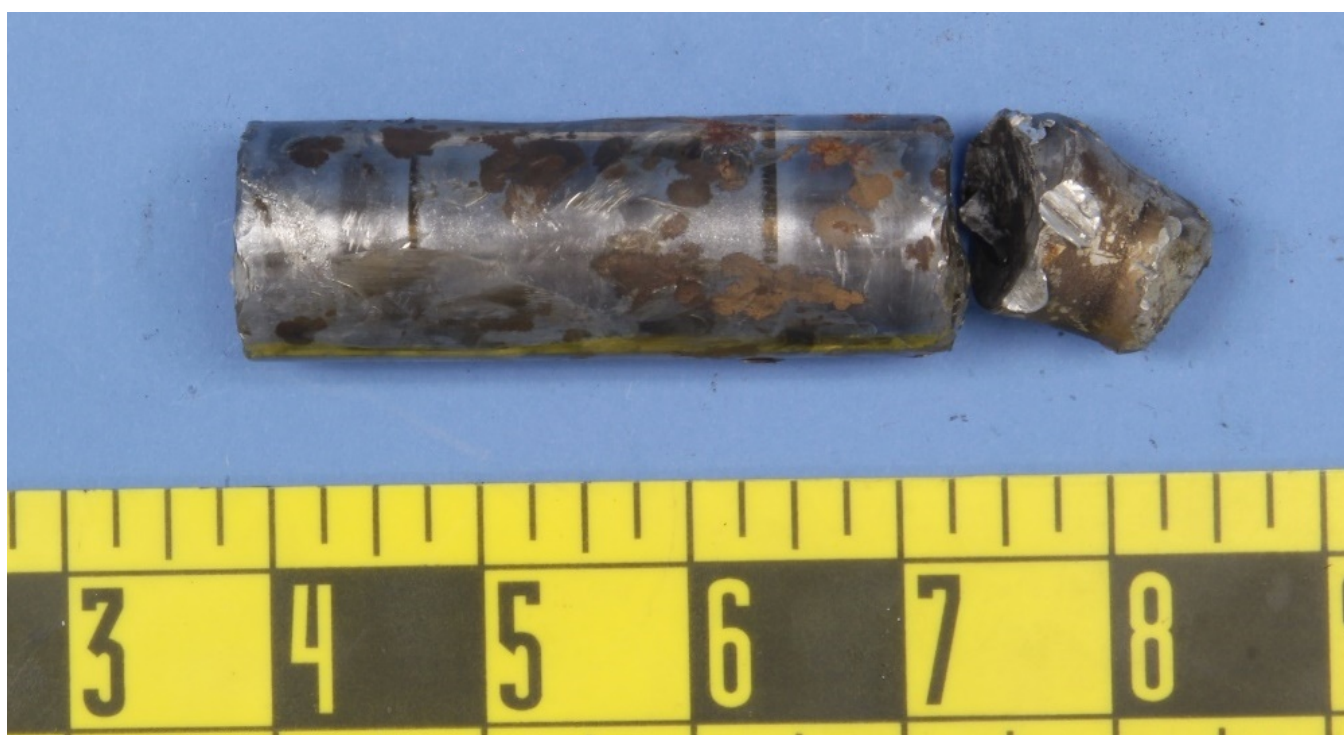
Figure 10 – The pieces of the piston pin from the #5 piston.
