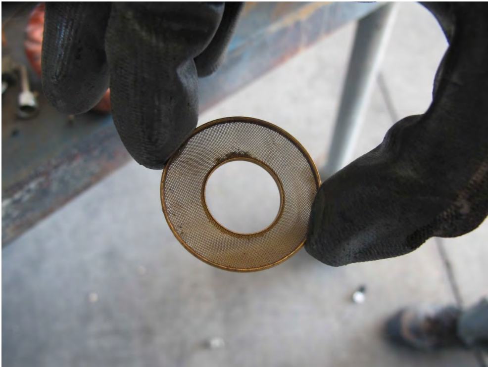
Photo 14 Fuel Manifold Valve Screen
