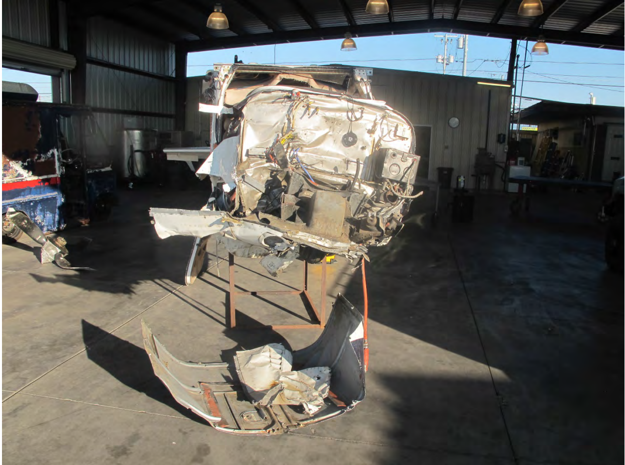
Photo 1 Front of Airplane with Engine Removed
