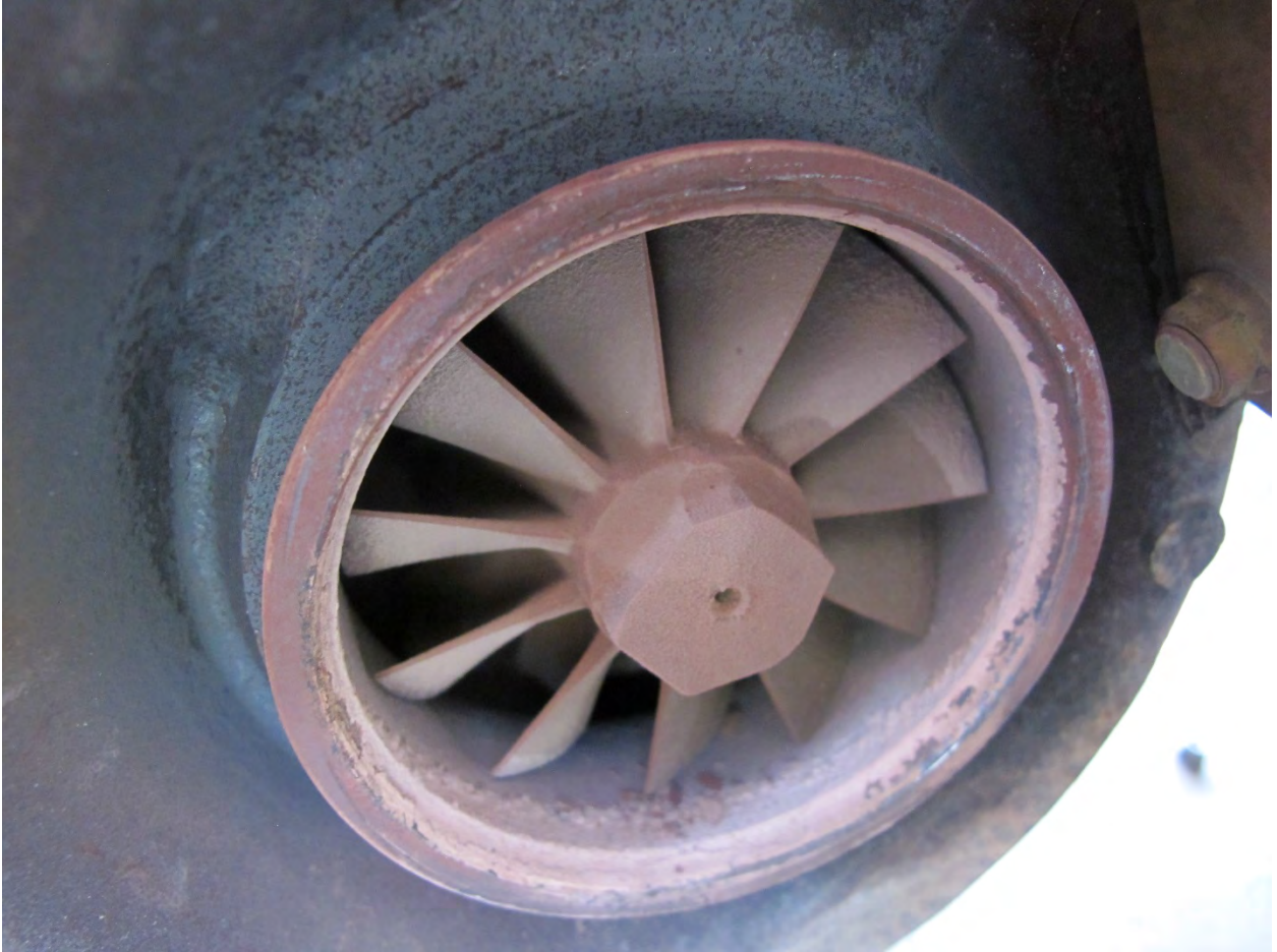
Photo 16 Turbocharger Turbine Blades
