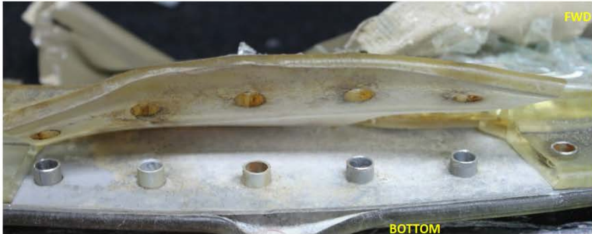
Figure E: LH Windshield Corroded Insert
