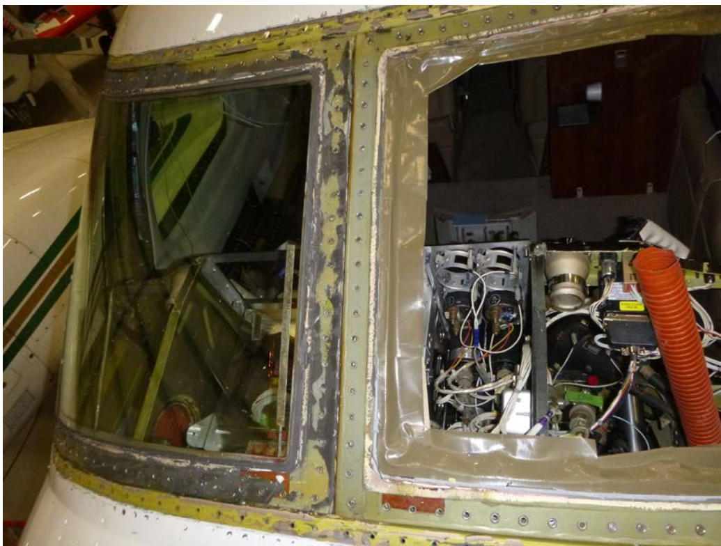
Figure 3 – Left and right windshields after frame removal, N909PW
