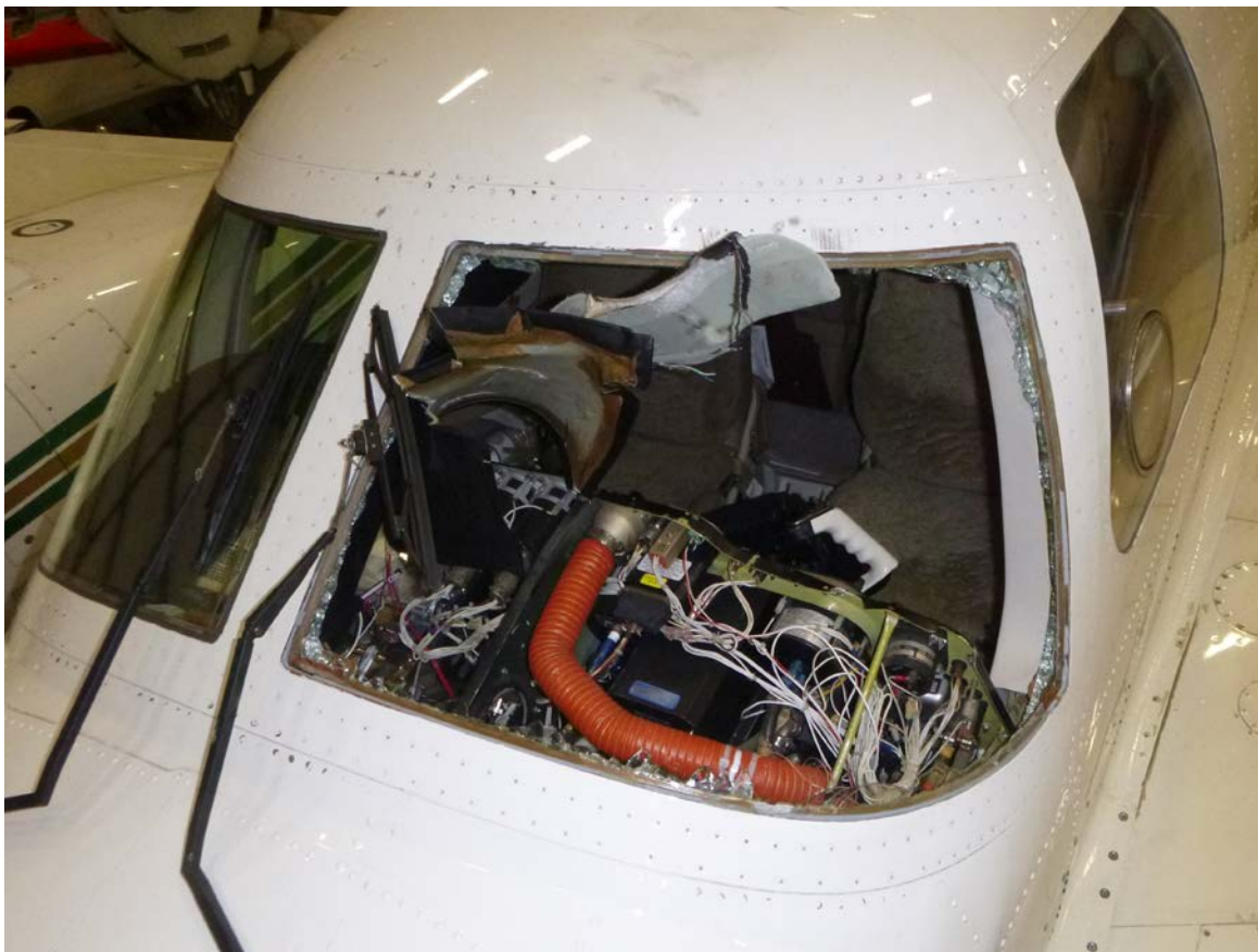
Figure 2 – Fractured left windshield, N909PW
