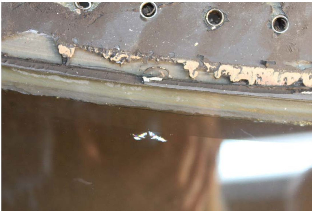
Figure 8 – Peel chip fracture on right windshield
