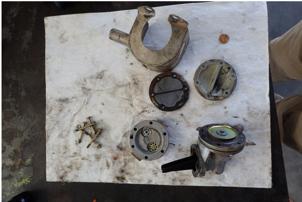
Photo 9 – Engine Driven Fuel Pump
