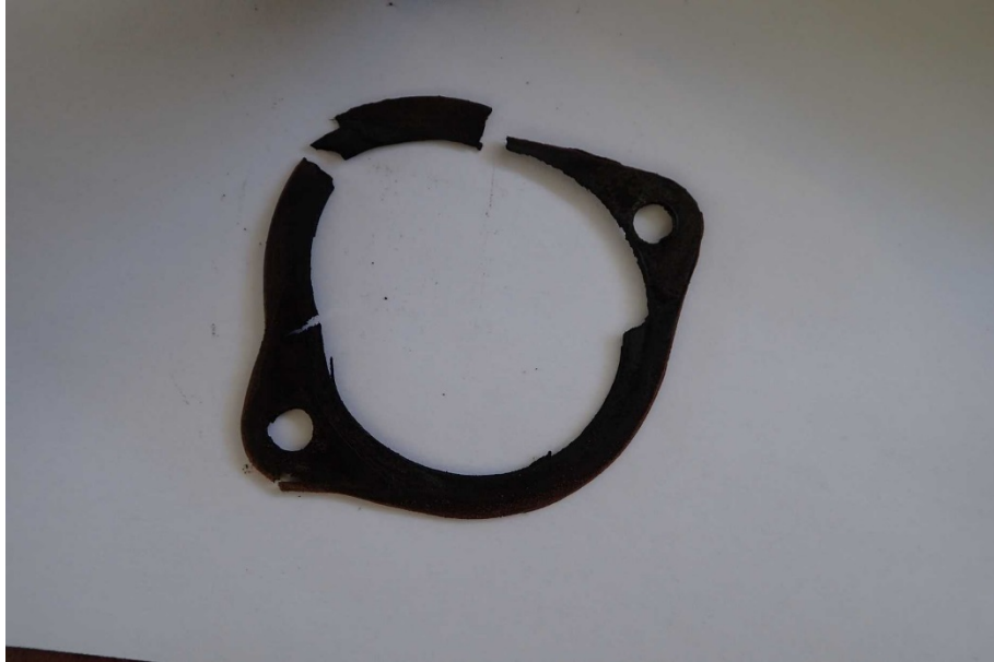
Photo 4 – Number 3 Intake Manifold Gasket
