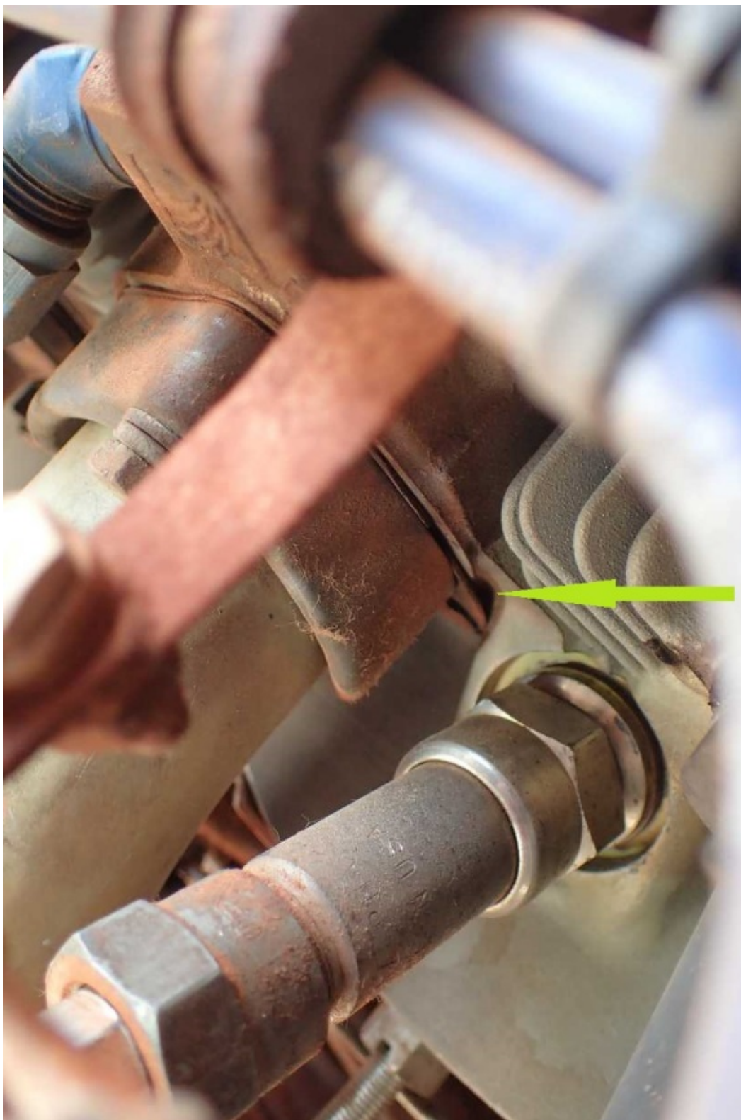
Photo 3 – Number 3 Cylinder Intake Manifold Gasket
