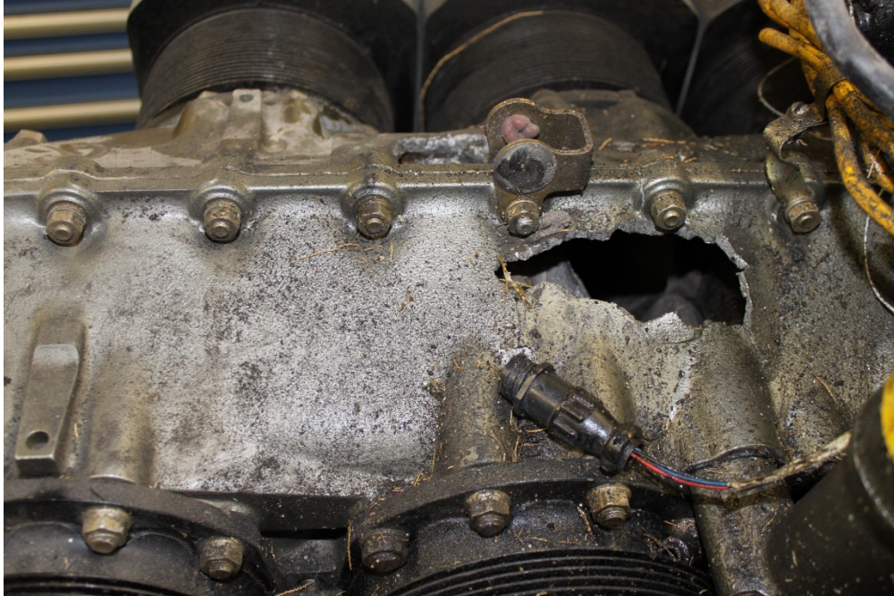
Figure 4 Upper crank case damage
