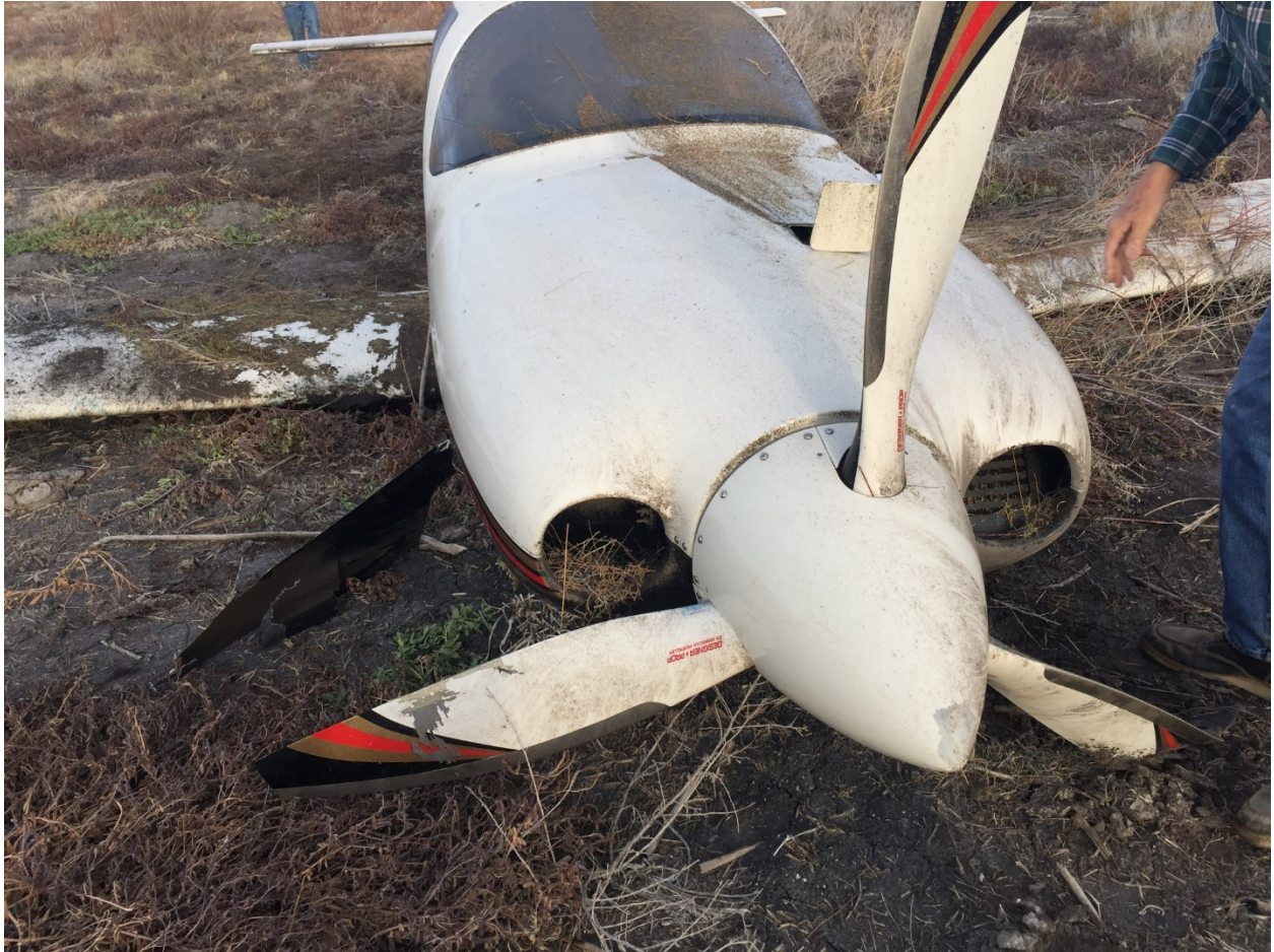
Figure 2 Damage to fuselage and wings
