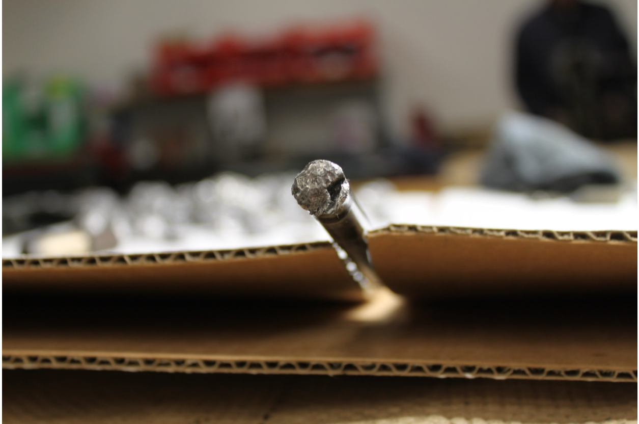
Figure 7 Alternative view of cylinder 3 valve stem and guide
