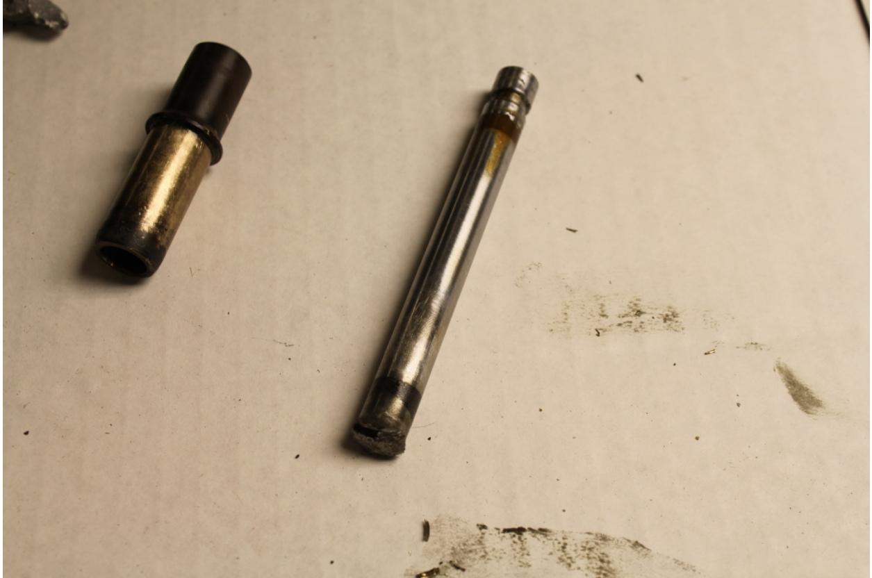
Figure 6 Cylinder 3 valve stem and guide
