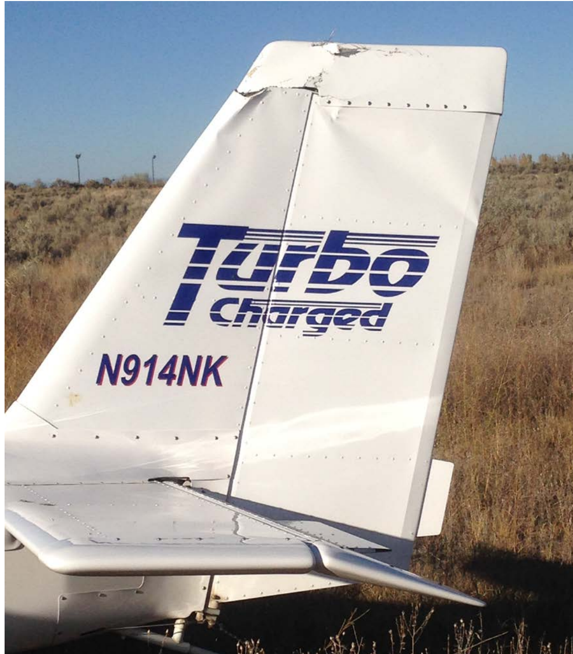
Photo 1 – View of Vertical Stabilizer and Rudder at Accident Site (Courtesy of Federal Aviation Administration)
