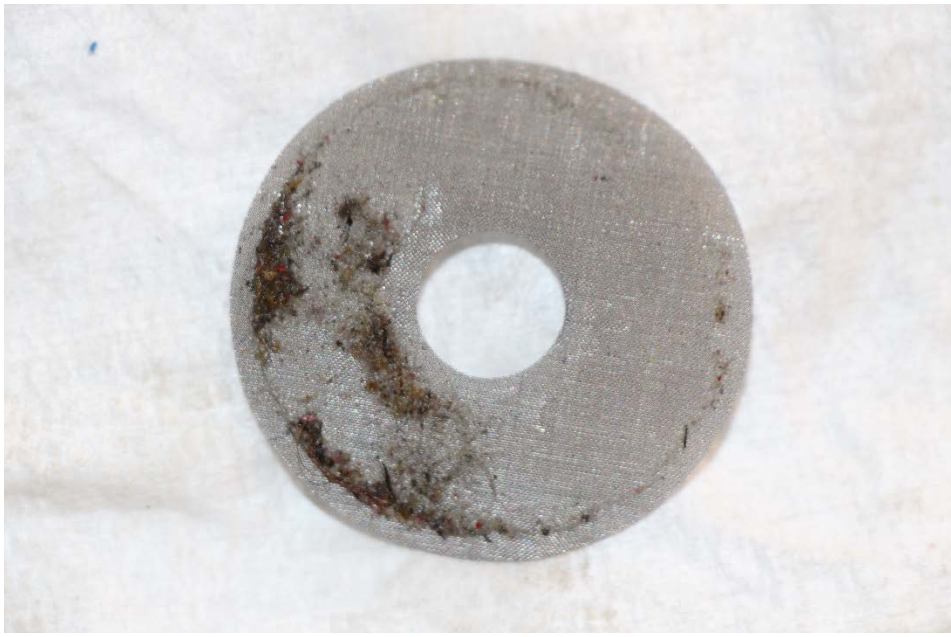
Photo 6: Gascolator Fuel Filter Screen
