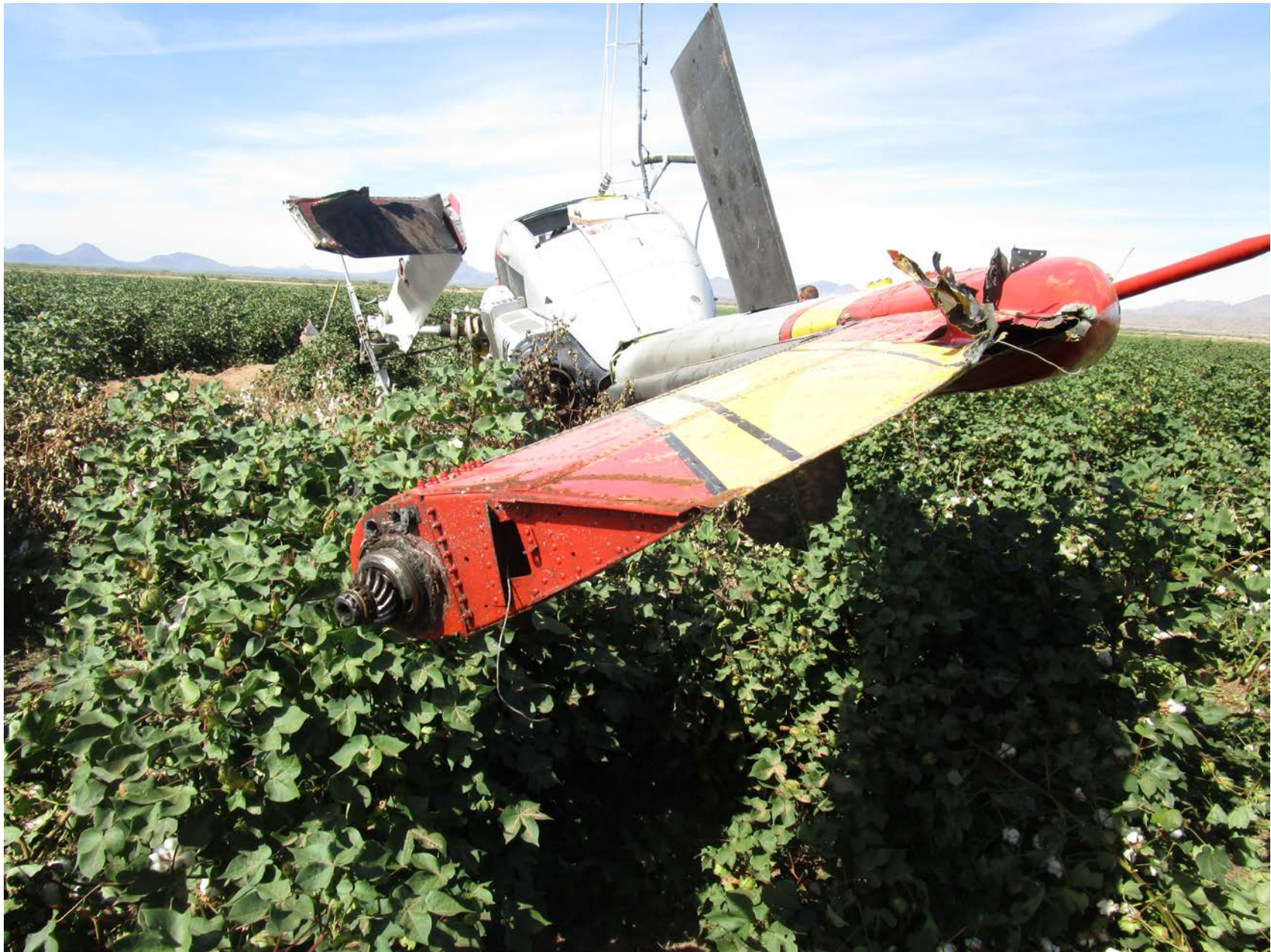
Photo 2 – Vertical Fin at Accident Site
