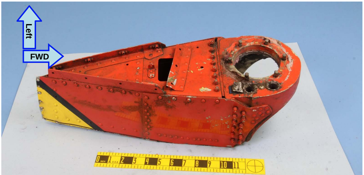
Figure 1. Overall views of the as-received components. Tail rotor gearbox with separated input quill at top and the upper portion of the vertical fin with gearbox mounting studs below.
