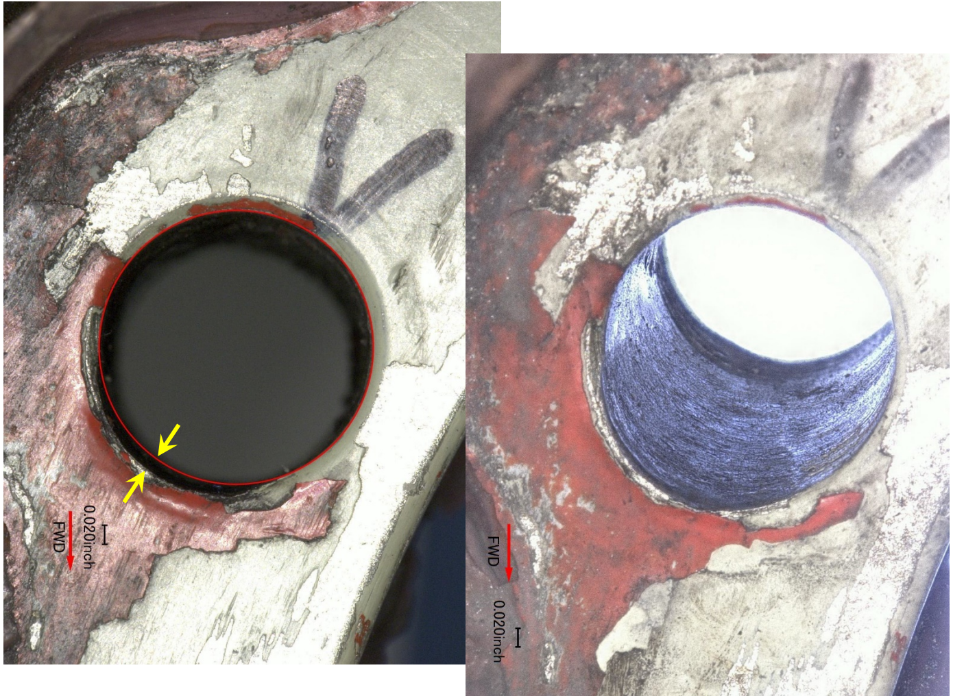
Figure 5. Two views of the #3 stud hole. Left view shows a plan view with the wear between the yellow arrows. Right image shows the wear on the interior of the hole corresponding to the fretting wear on the stud.
