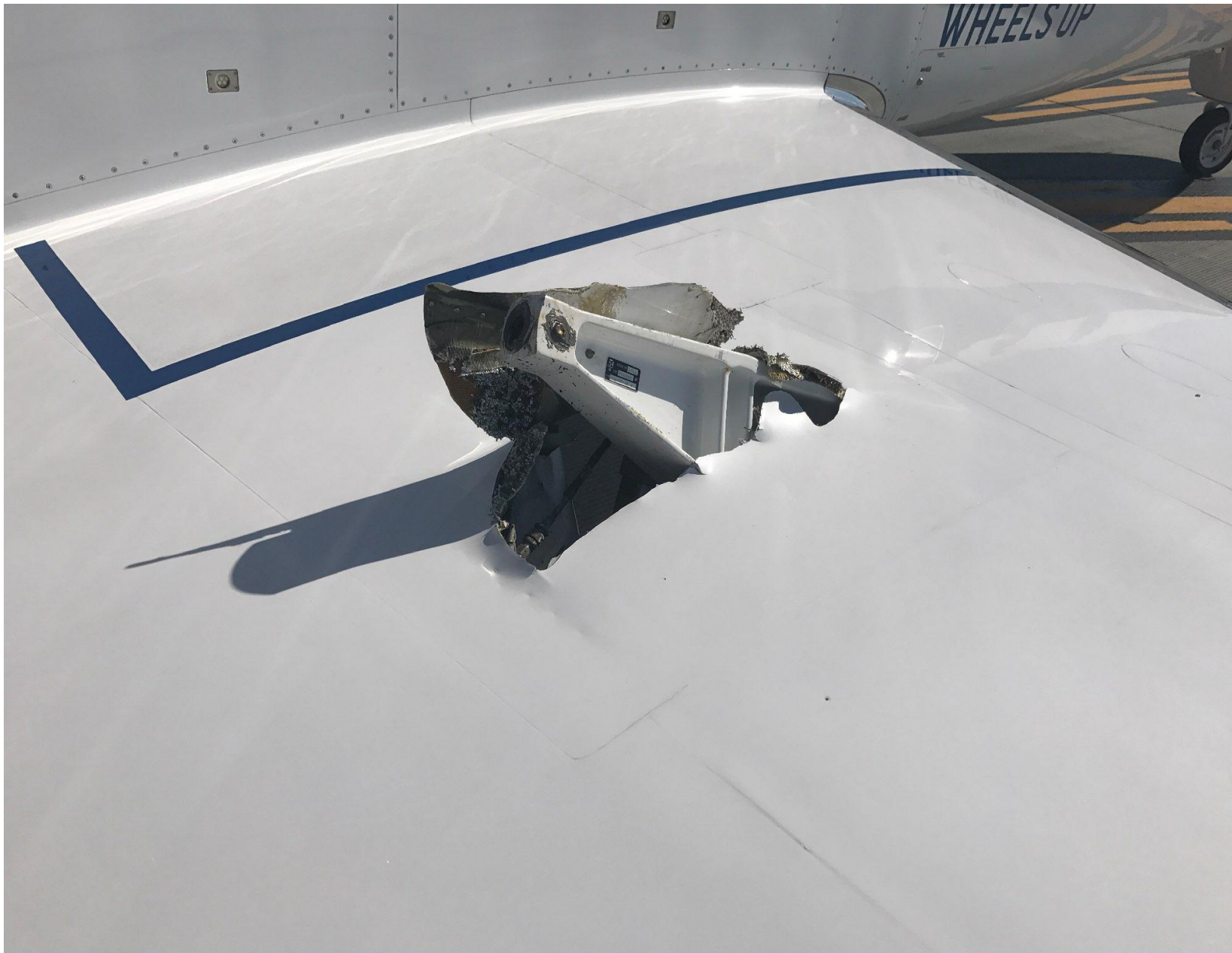
Photo 4 - Accident site, top surface of right wing and right landing gear trunnion.
