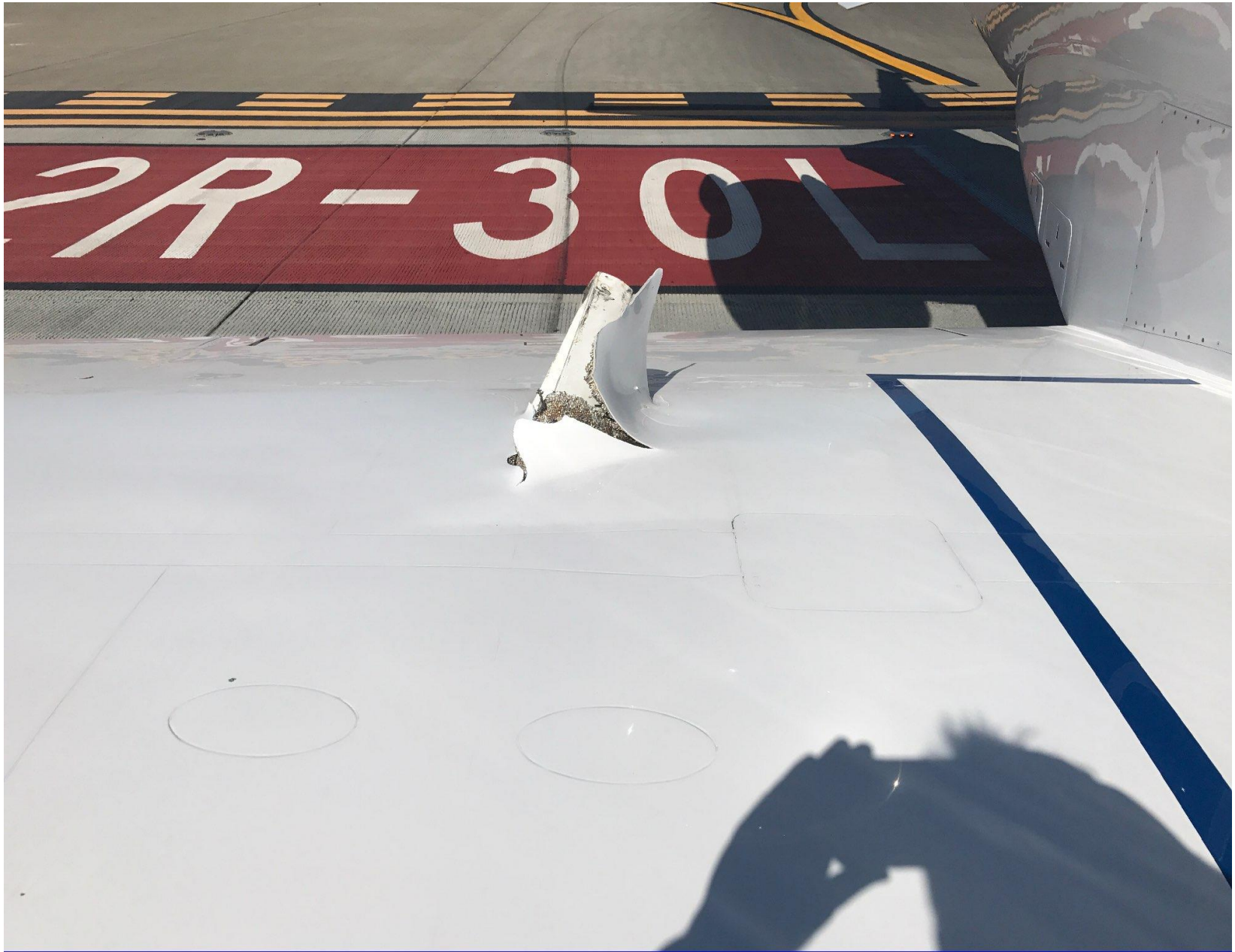
Photo 2 – Accident site, top surface of right wing and right landing gear trunnion.
