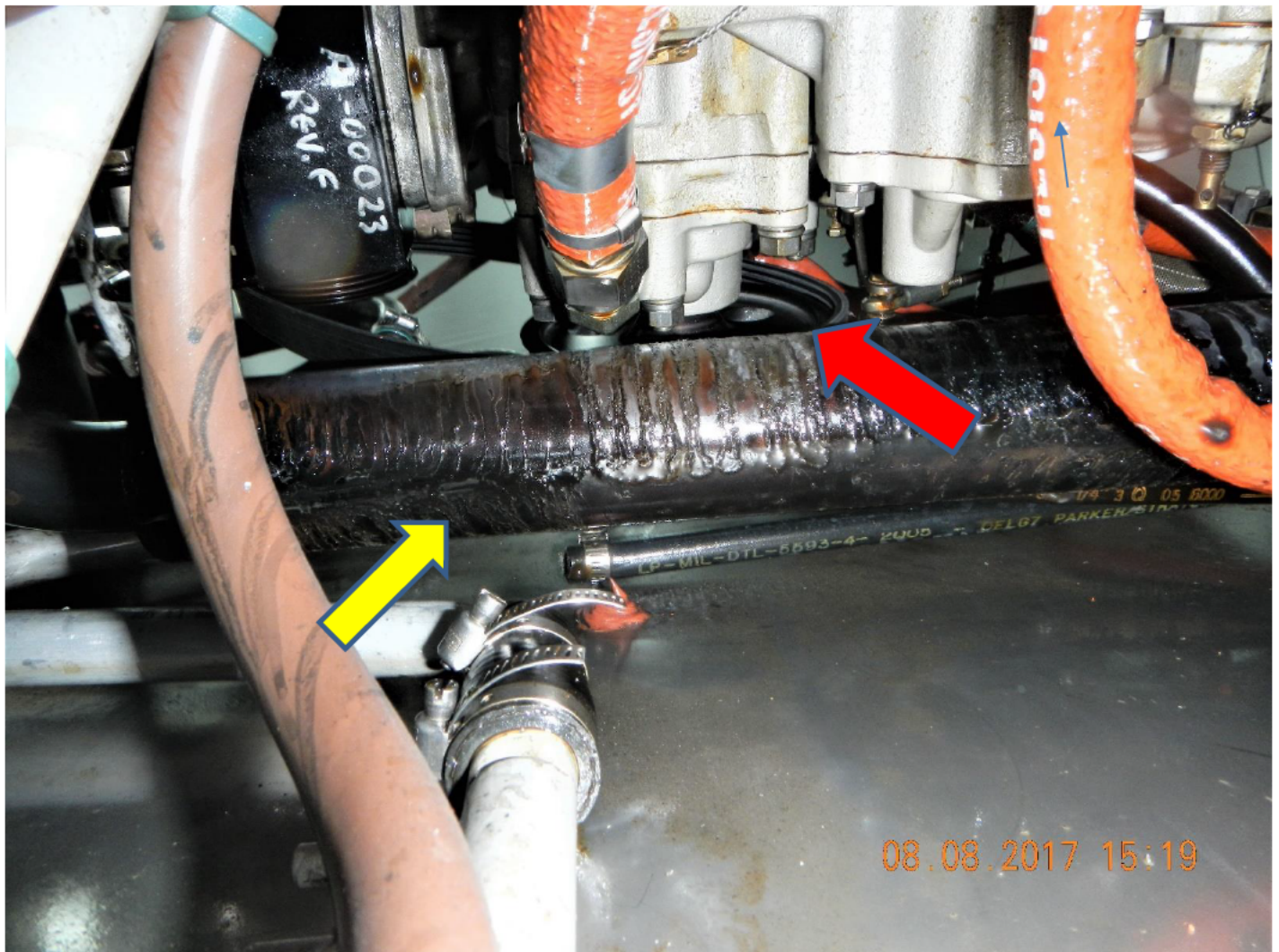
View looking up from beneath the engine near the firewall. The red arrow points to the starter adapter and aftermarket pulley used to power the optional third alternator. NOTE the baked-on oil on the outer surface of the exhaust cross-over tube located directly under the starter adapter pulley (yellow arrow).
