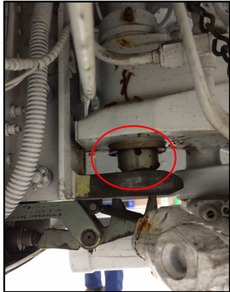
Figure 2: View of an exemplar airplane's nose gear down-lock actuator piston (note chrome color) as provided by the operator.
