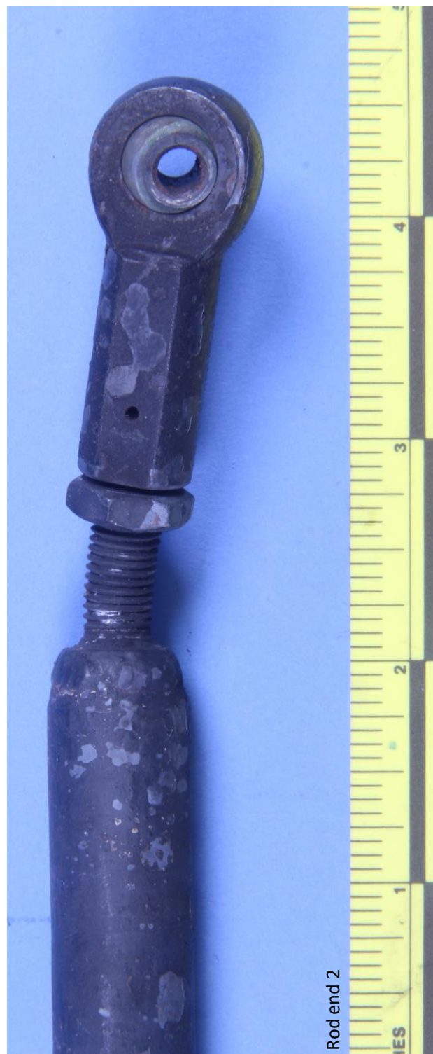
Figure 4 Closer view of rod end bearing 2
