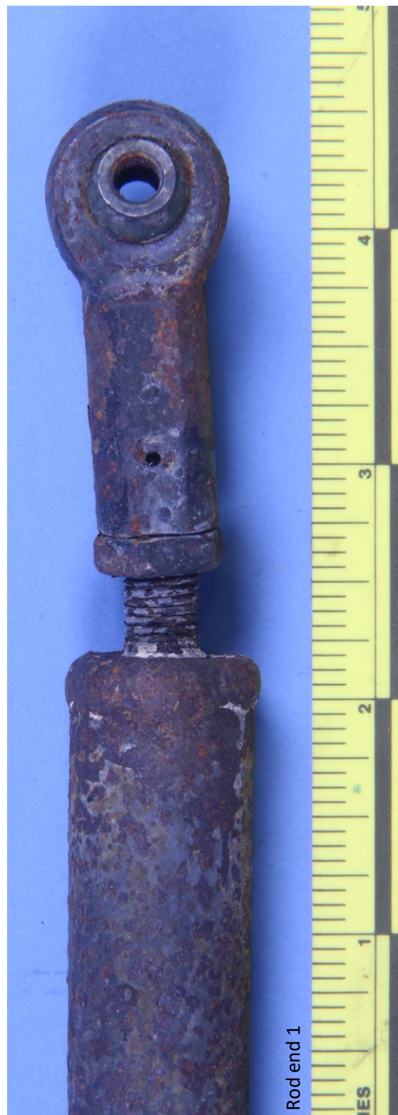
Figure 3 Closer view of rod end bearing 1.
