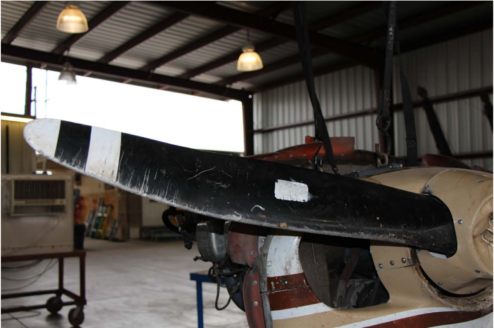
Photo 6 – Propeller Blade with Forward Bending
