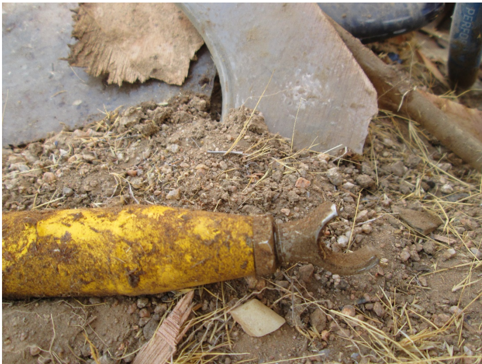
Figure 8: Fractured Left Aileron Control
