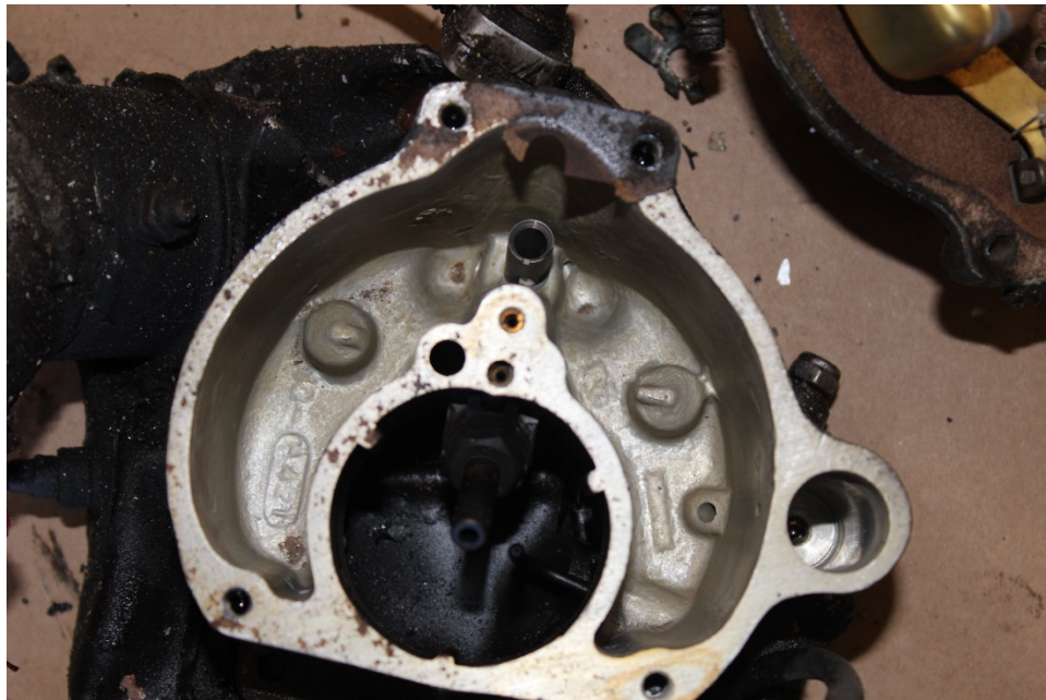
Figure 4: Carburetor Bowl and Accelerator Pump Well
