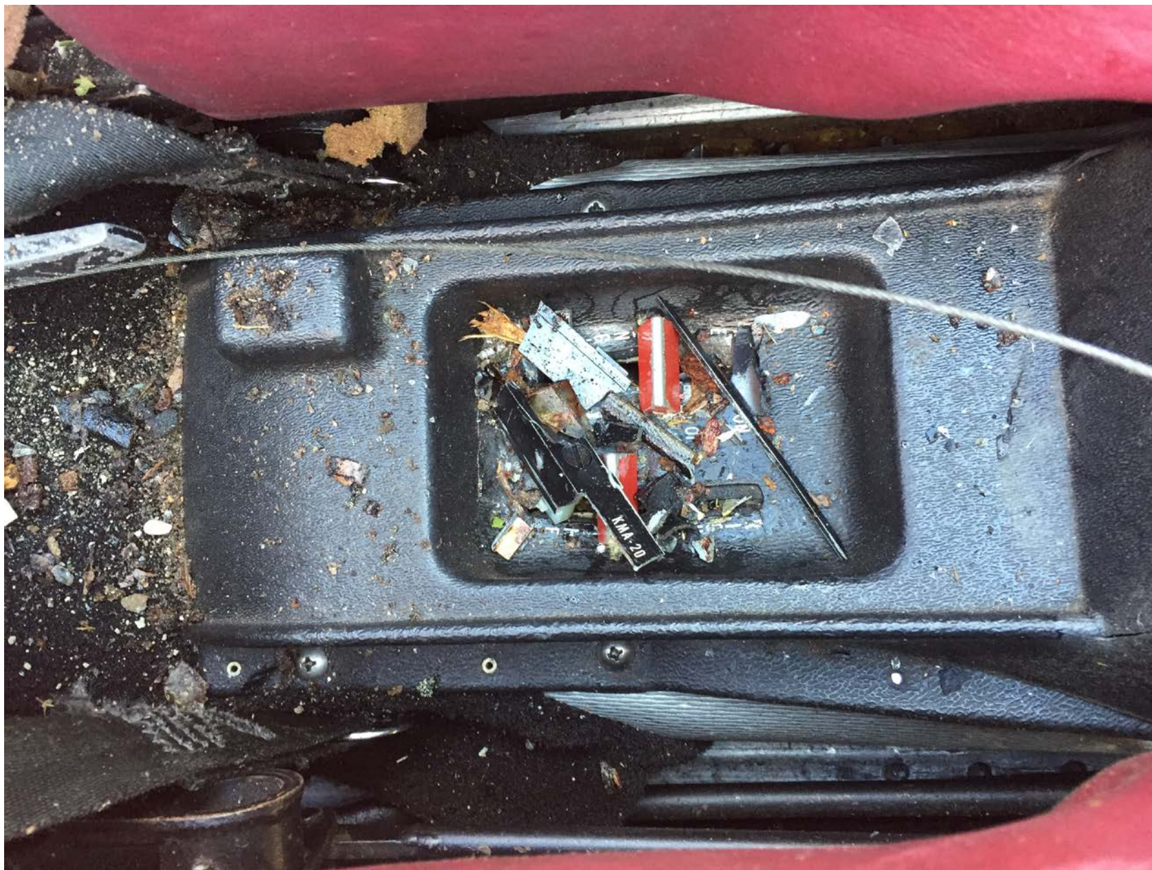
Photo 5 – Fuel Selector Handles
