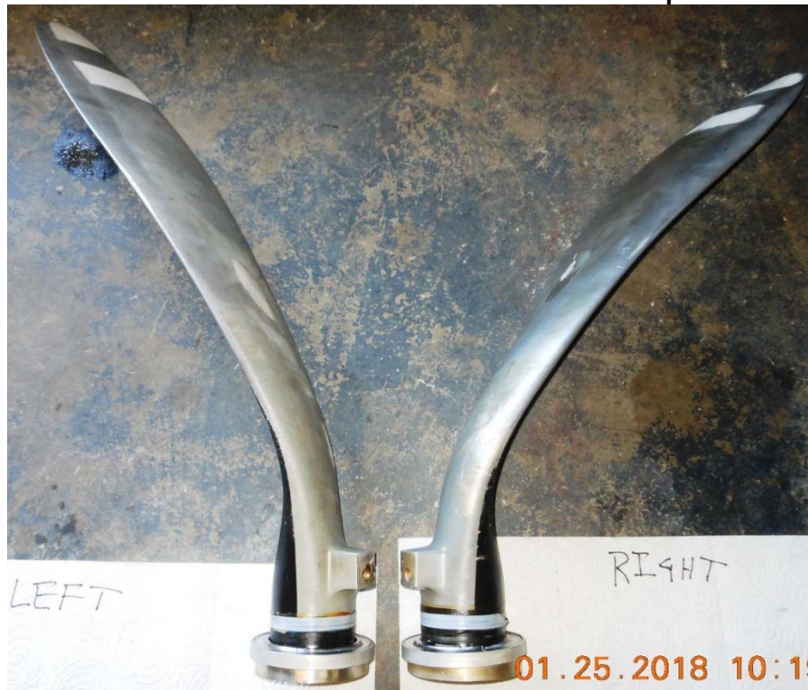
Photo #2 – Blades R1 and L1 bend and twist comparison
