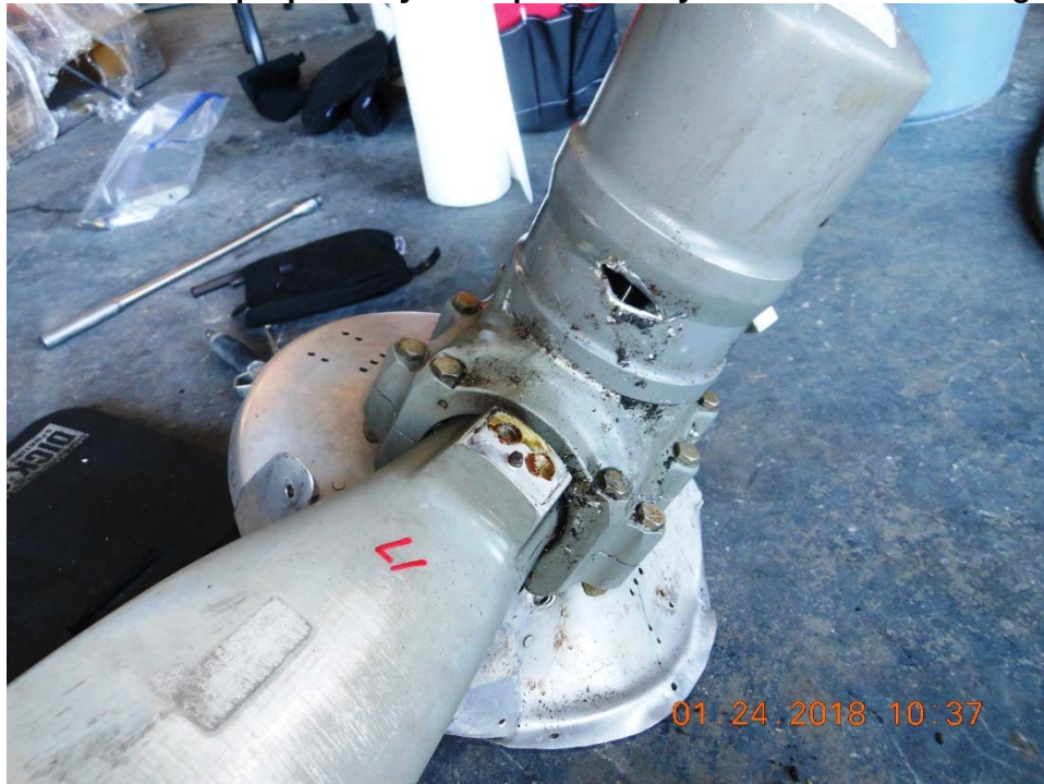
Photo #7 – Left propeller cylinder puncture by blade L1 counterweight
