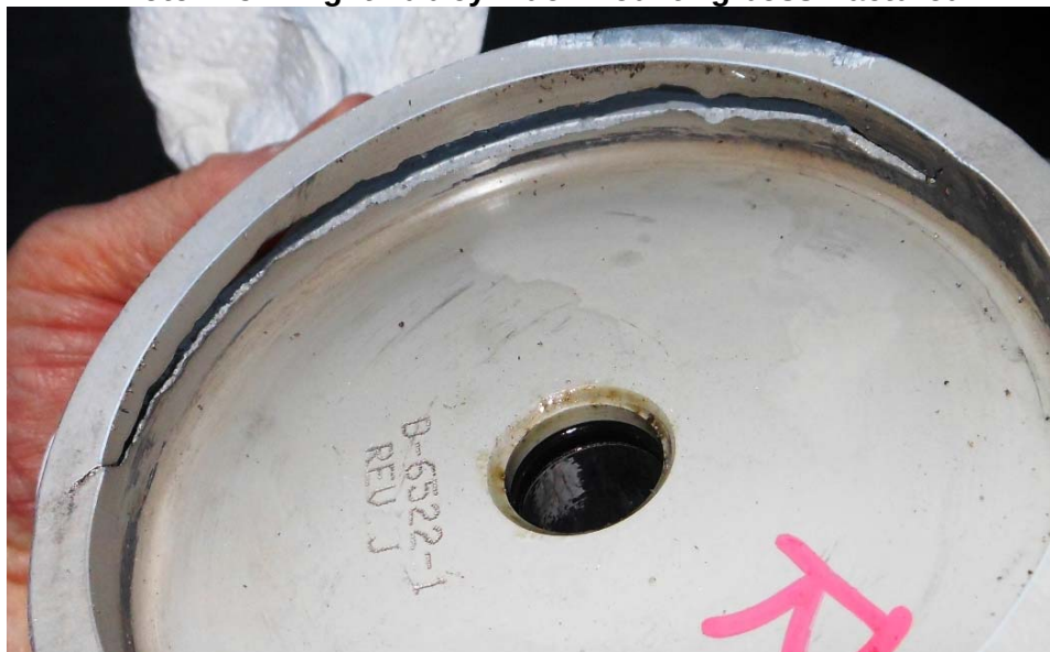
Photo #25 – Right hub cylinder mounting boss fractured
