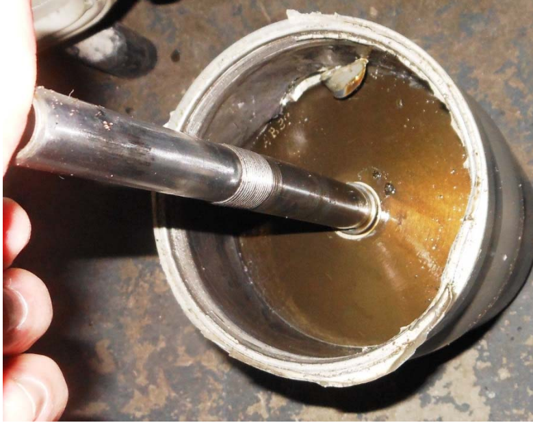
Photo #8 – Left piston bottom and pitch change rod trapped in cylinder
