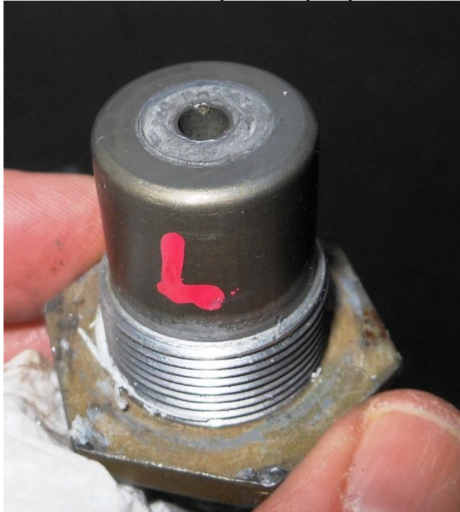
Photo #9 – Left low pitch stop impact mark
