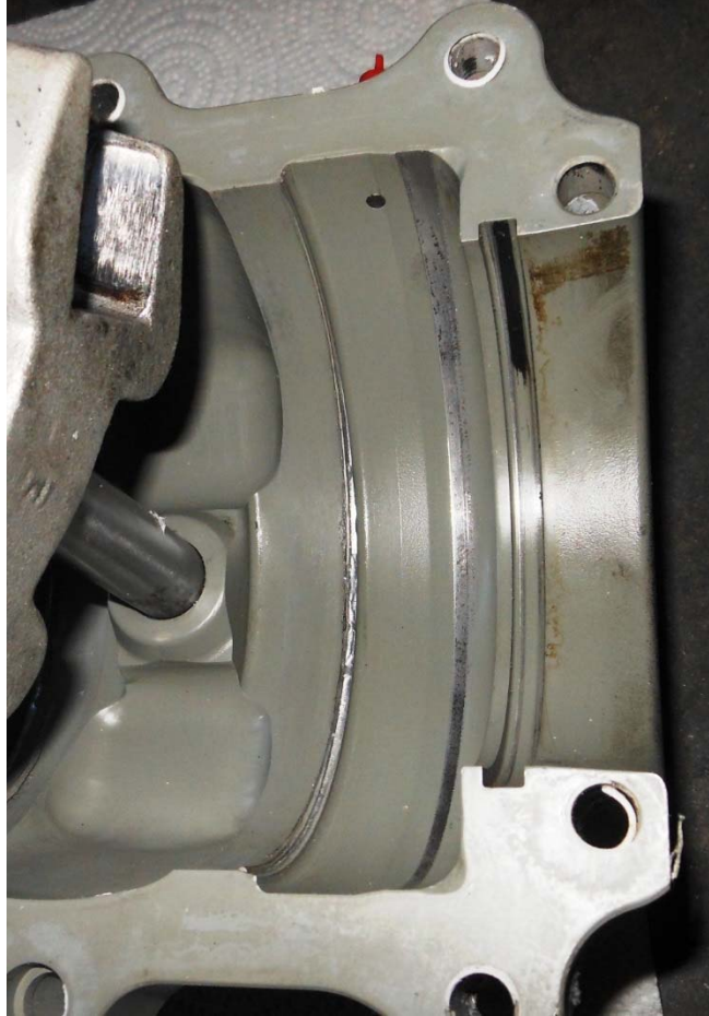
Photo #24 – Right aft hub half blade pocket R2
