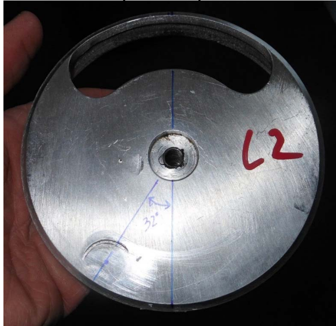
Photo #12 – Preload plate L2 impact mark measurement
