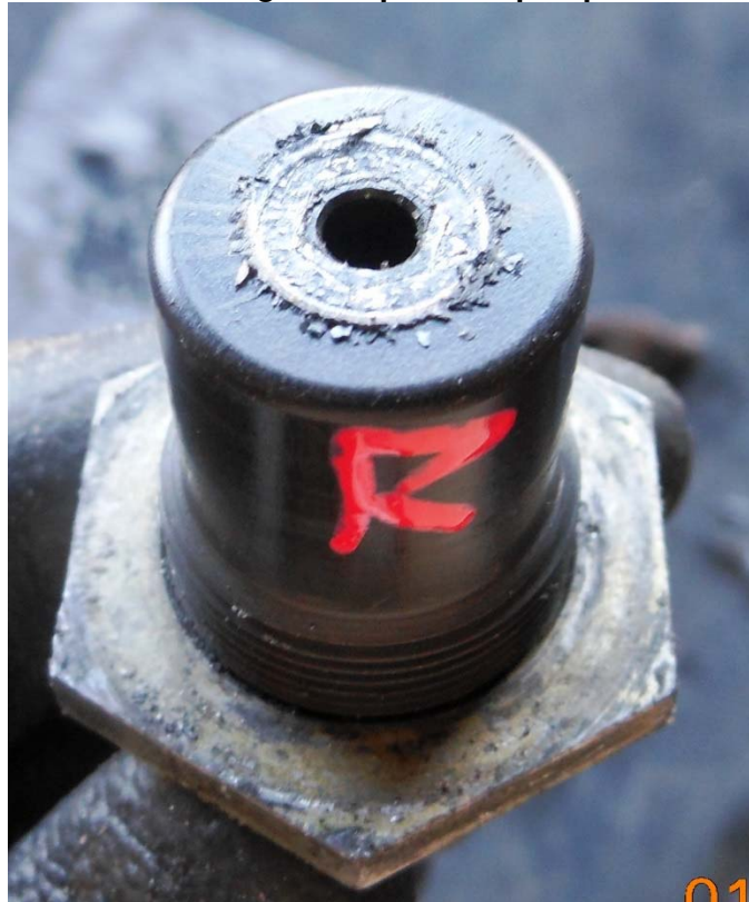
Photo #21 – Right low pitch stop impact mark
