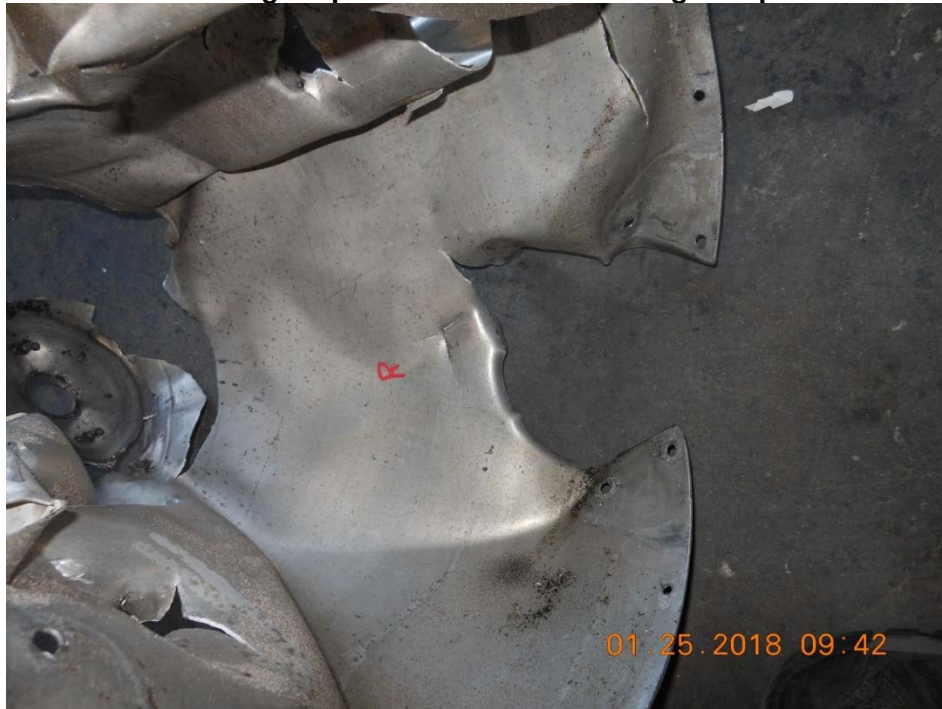
Photo #18 – Right spinner dome counterweight impact mark
