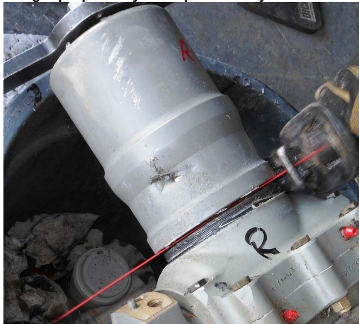
Photo #19 – Right propeller cylinder puncture by blade R1 counterweight
