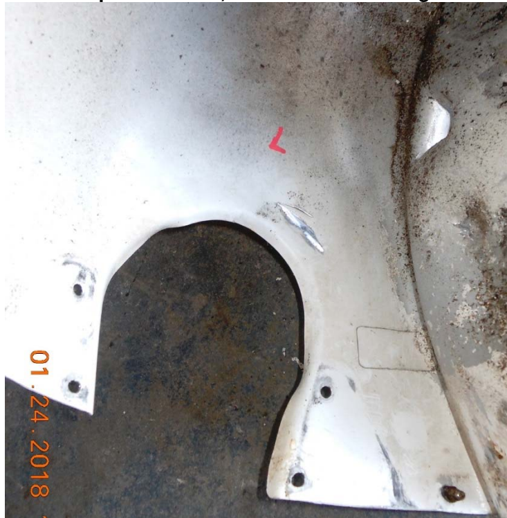
Photo #5 – Left spinner dome, internal counterweight contact mark
