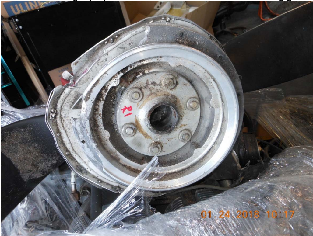
Photo #17 – Right propeller fractured crankshaft and starter ring gear
