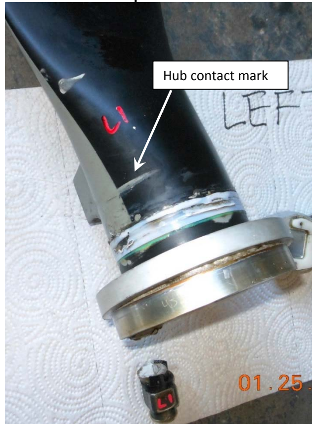
Photo #13 – Blade L1 hub impact mark and seal rub strip damage
