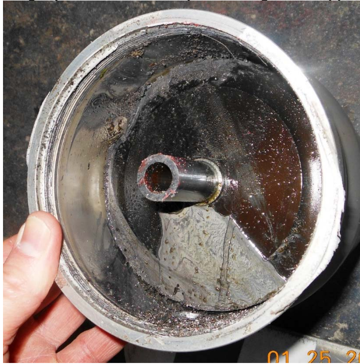
Photo #21 – Right low pitch stop impact mark
