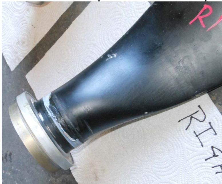
Photo #27 – Blade R1 hub impact mark and seal rub strip damage
