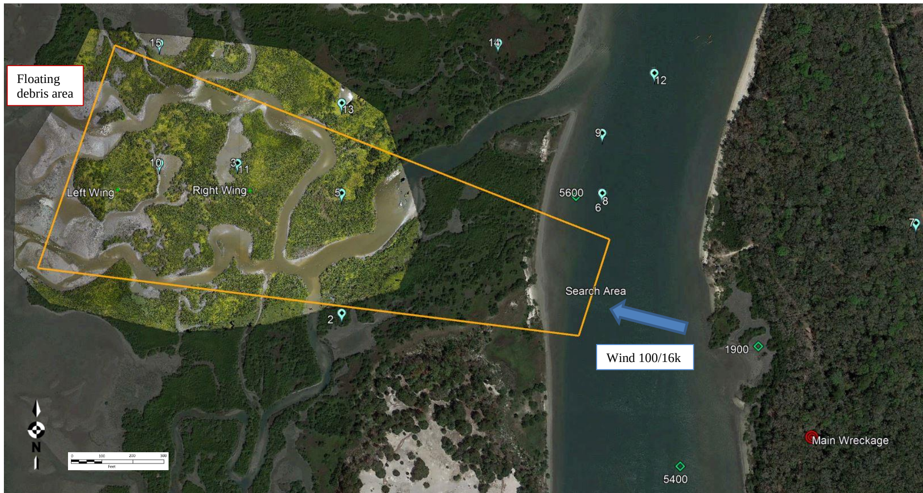
Figure 3 – Orthomosaic including wings, main wreckage, miscellaneous wreckage, radar targets, and search area.
