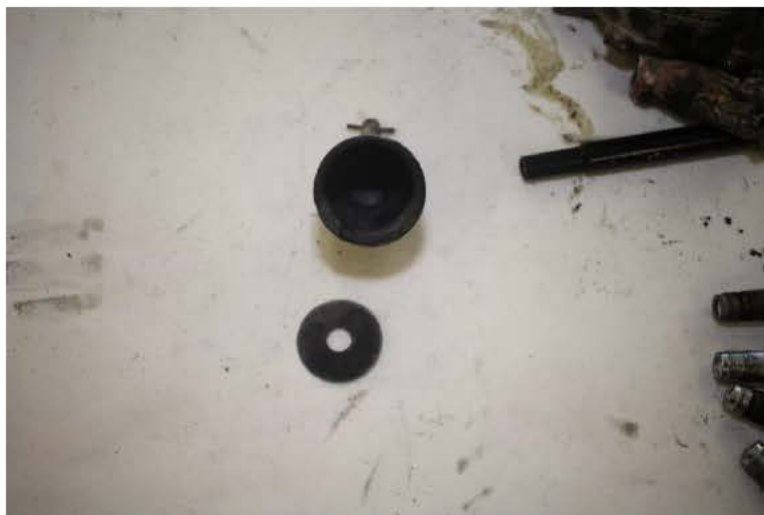
Figure 4: View of extensive thermal damage to the gascolator screen and bowl.
