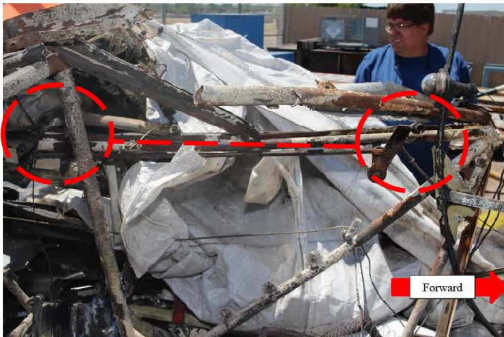
Figure 2: View of forward throttle quadrant still connected to aft throttle.
