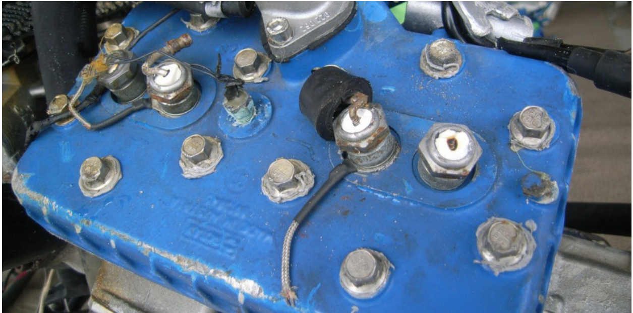
Figure 22 - Fractured Spark Plugs (PTO side to right)
