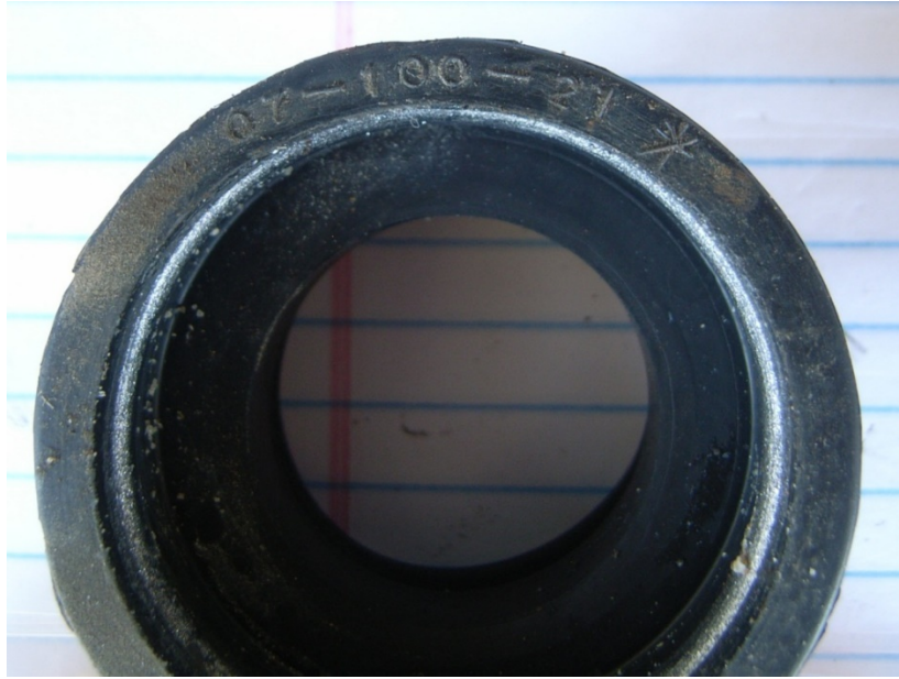
Figure 42 - MAG End Socket (incorrect PN)
