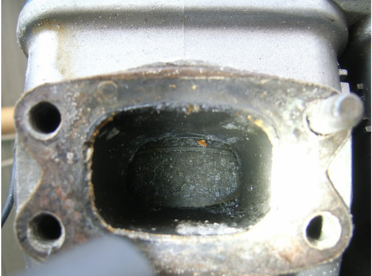
Figure 44 – MAG End Piston (via exhaust port; note lack of scoring, typical)
