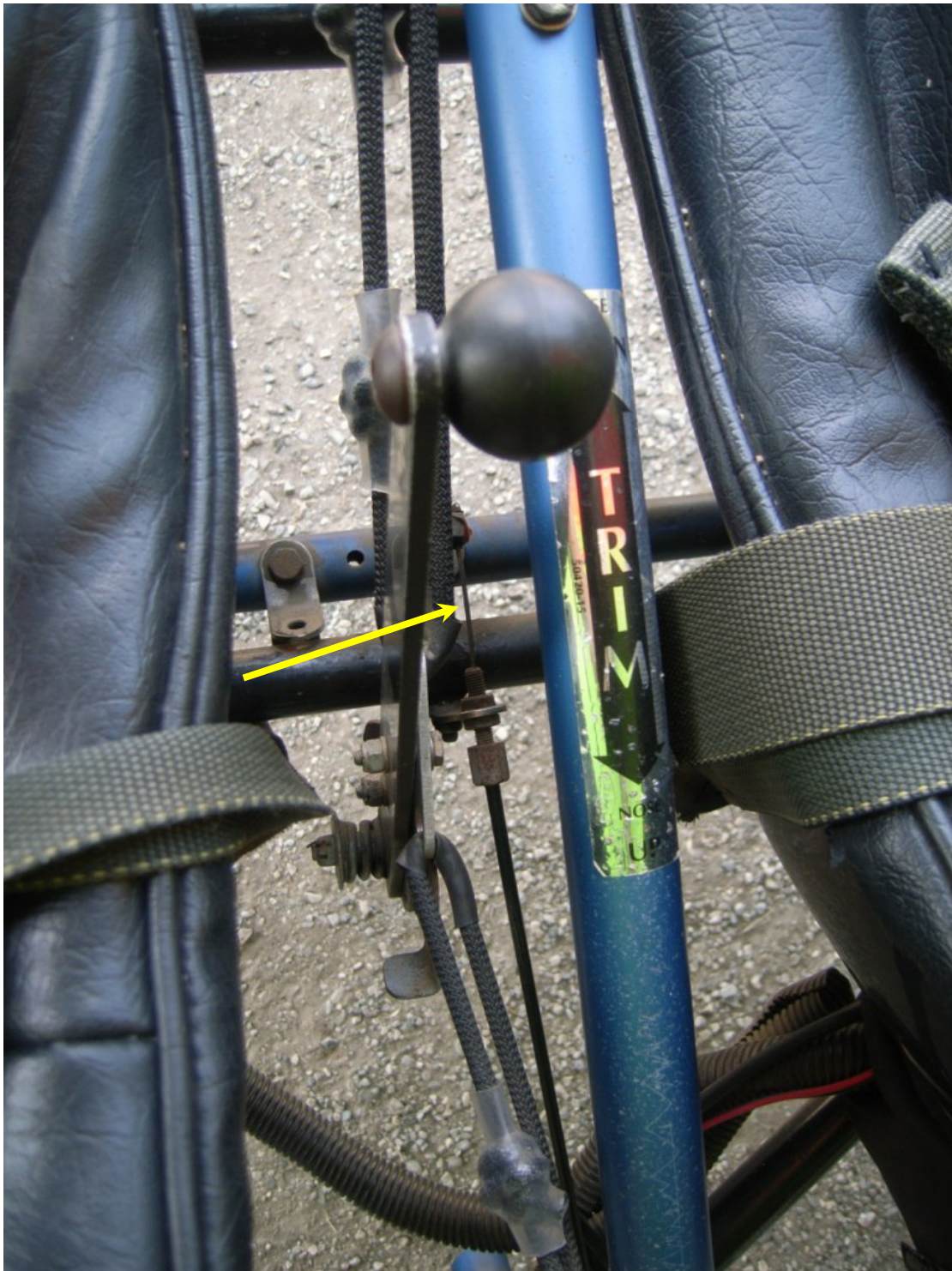
Figure 13 - Exemplar Central Throttle Linkage (looking down)
