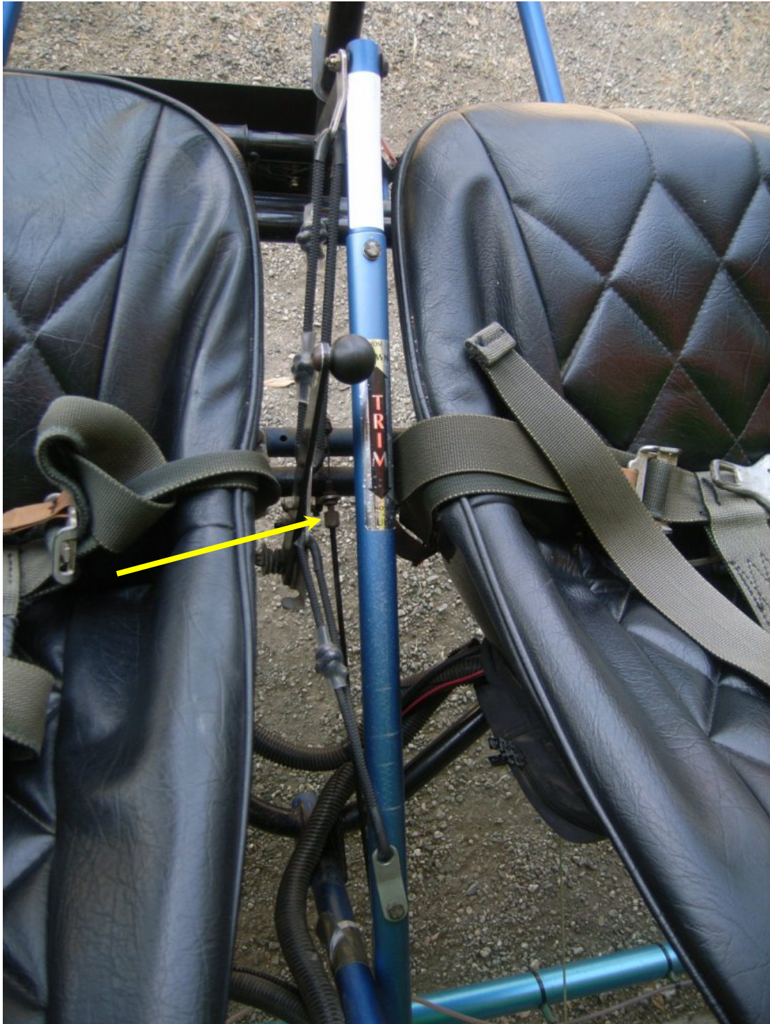
Figure 12 - Exemplar Central Throttle Linkage (looking down)
