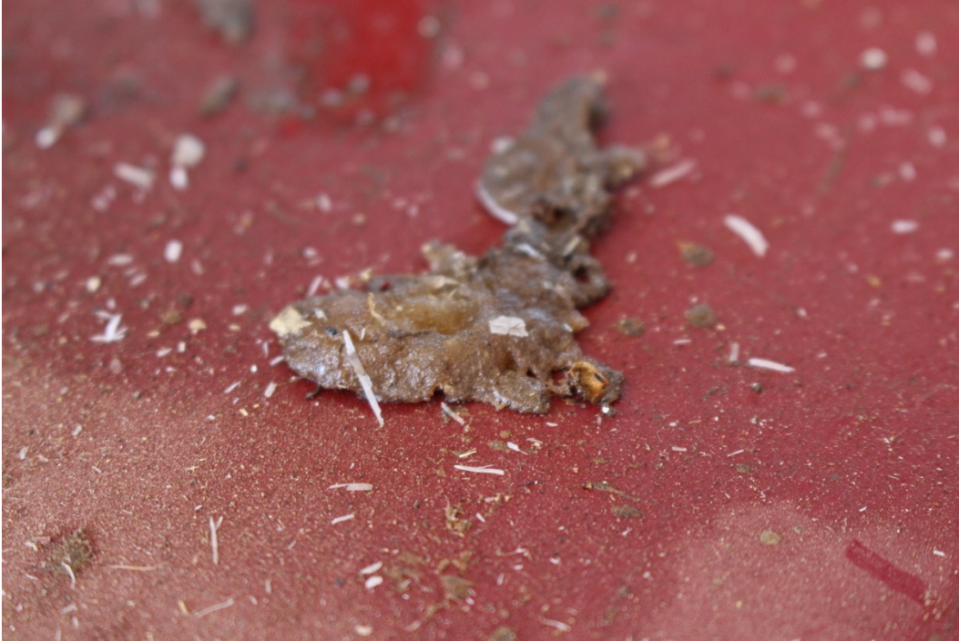
Figure 2: View of Snarge Found on Horizontal Stabilizer.
