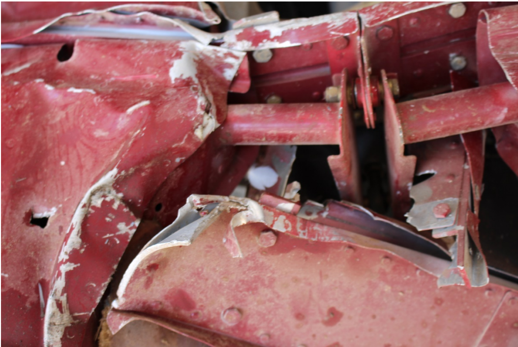
Figure 3: View of Feather Found in Empennage.
