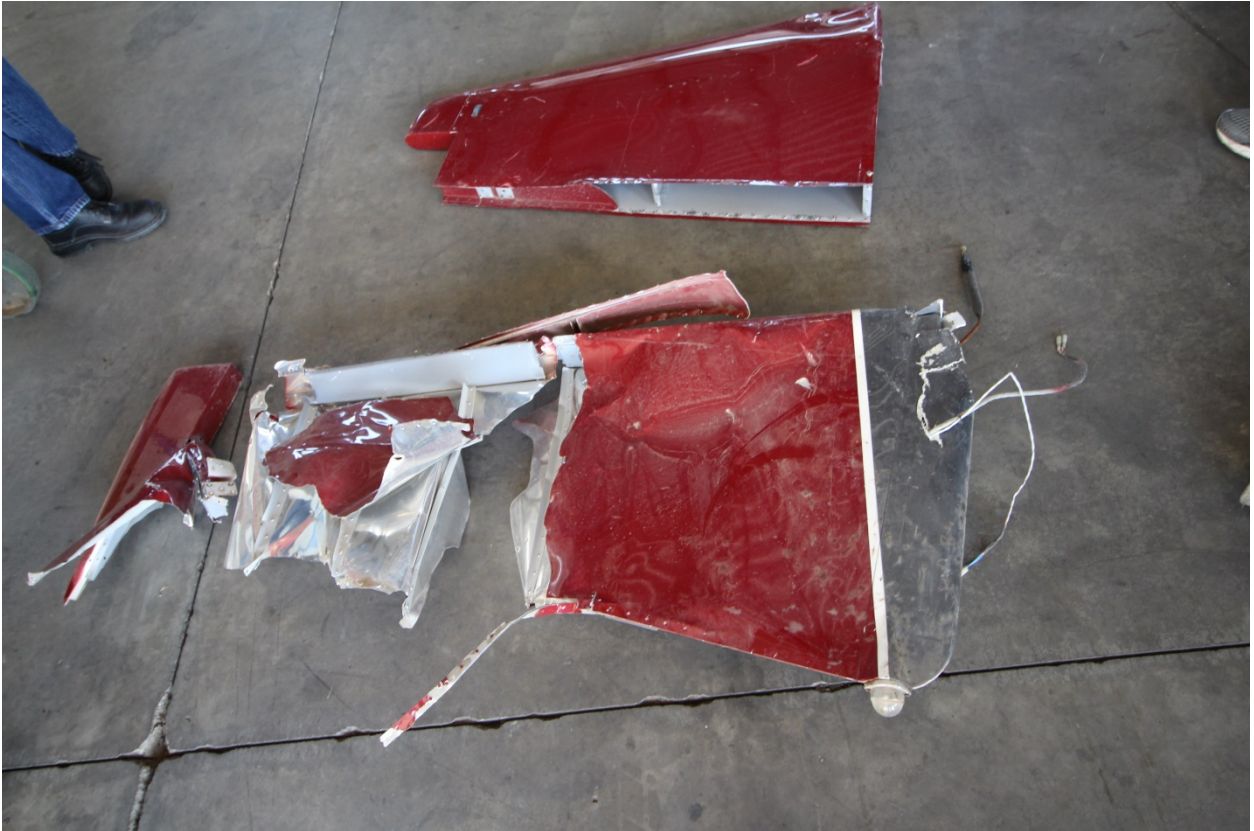
Figure 1: View of Empennage Section Found About 1.3 Miles from Main Wreckage.
