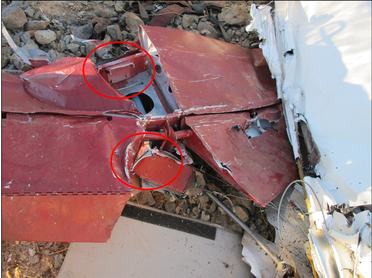
Figure 6-Horizontal Stabilizer and Elevators
