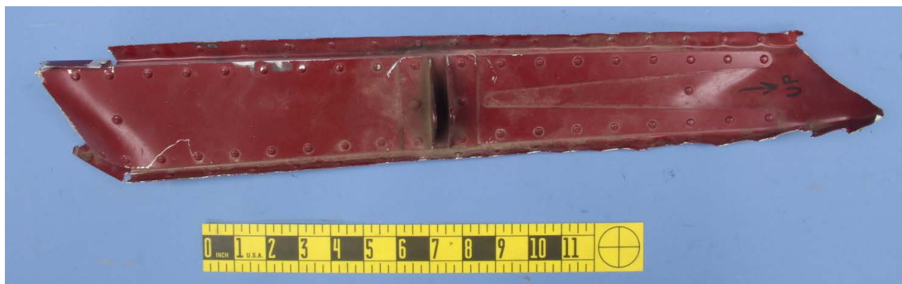
Figure 13 – The separated section of the aft vertical spar from the vertical stabilizer, viewed aft looking forward.
