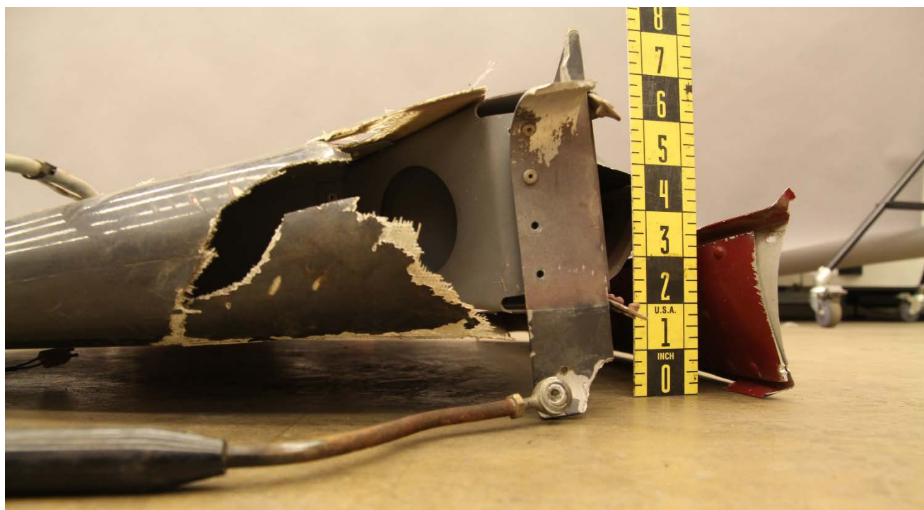
Figure 16 – Closer view of underside of the tail rudder, showing fracture to the composite skin, bending and tearing of the support plate and the fracture surface of aft vertical spar.
