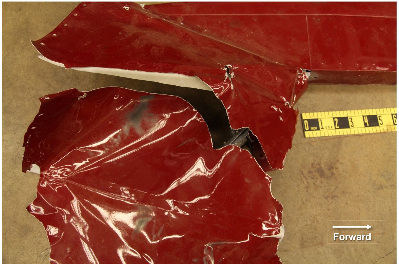
Figure 8 – Torn and fractured portion of the skins on the upper portion of the right side of the rudder.
