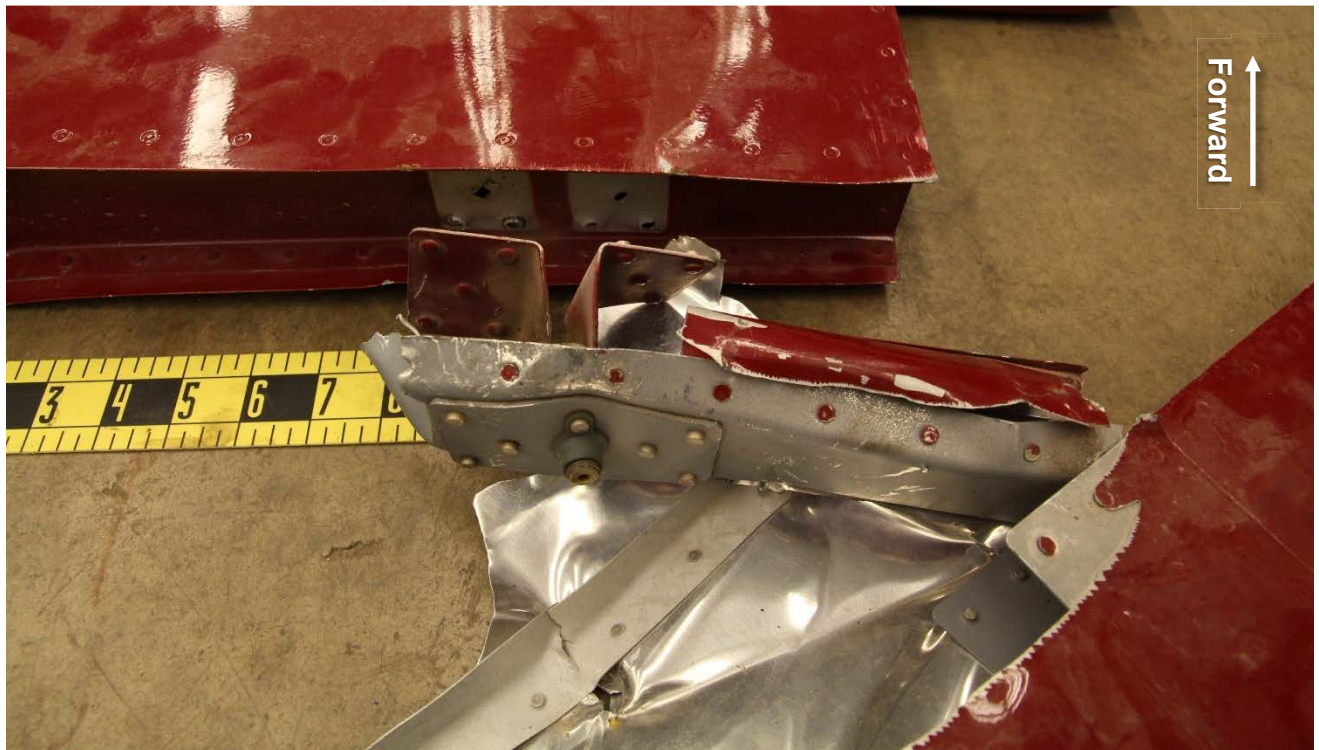
Figure 12 – Position of the upper portion face of the vertical stabilizer, showing rudder attachment flanges that had separated from the aft vertical spar.
