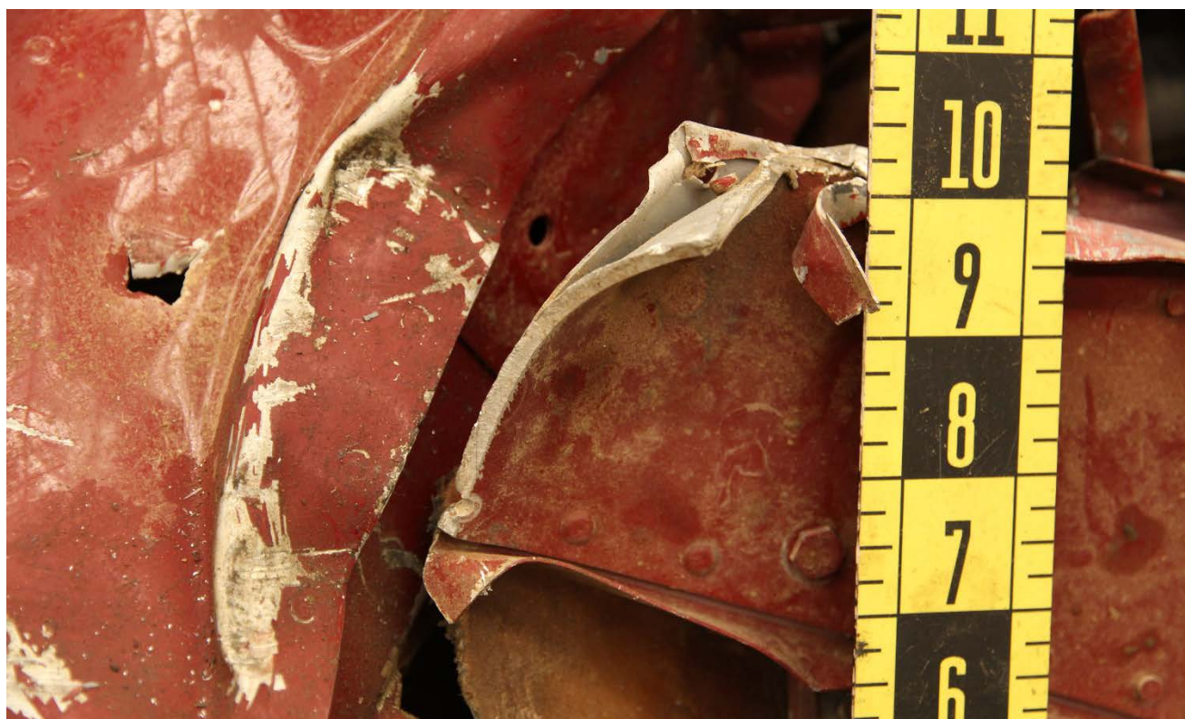
Figure 20 – The fracture surface of the lower section of the aft vertical spar from the vertical stabilizer, still affixed to the horizontal stabilizer assembly.
