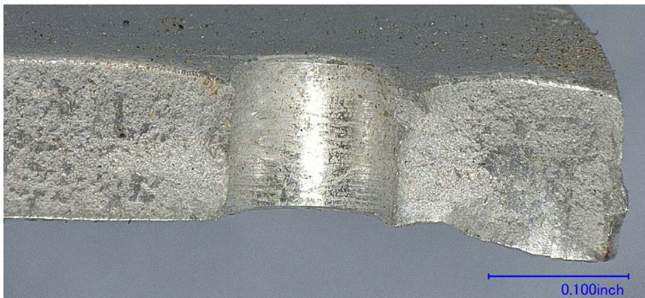
Figure 23 – Portion of the fracture about the rivet hole on the fracture surface in Figure 22.
