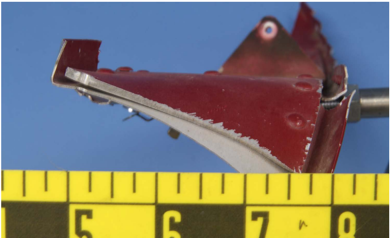
Figure 22 – The upper mating fracture surface of the separated section of the aft vertical spar from the vertical stabilizer, shown in Figure 16.
