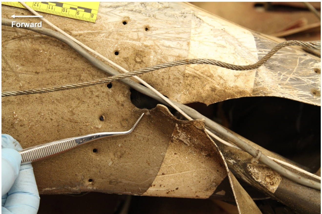
Figure 27 – An example of organic material, consistent with avian material, extracted from the underside of the empennage tailcone.
