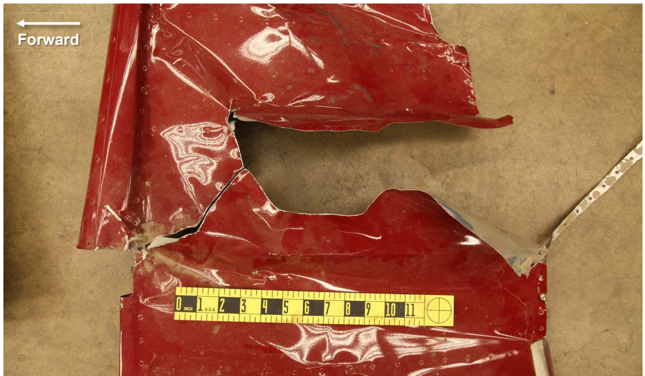
Figure 7 – Closer view of the fracture of the rudder skin on the left side.
