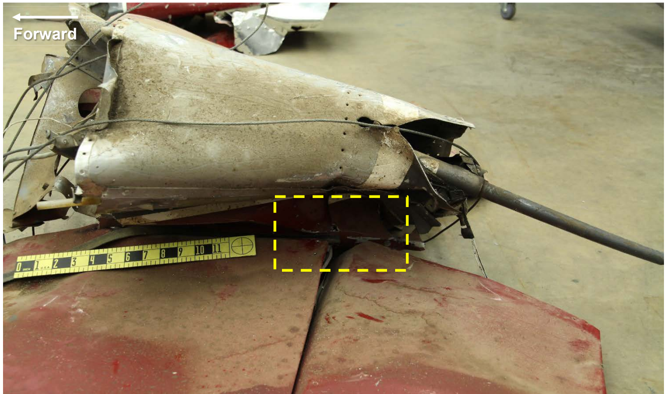
Figure 25 – A view of the underside of the horizontal stabilizer assembly, showing a impressed or dented region in the structure. The boxed area is shown in Figure 26.
