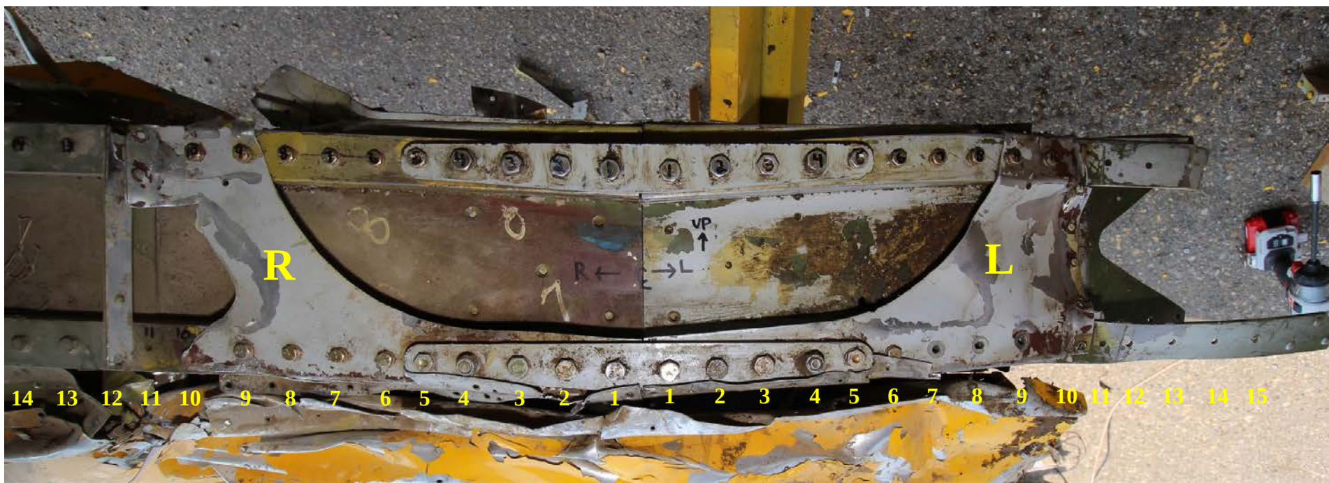
Figure 4 – Center portion of main wing spar, viewed looking aft
