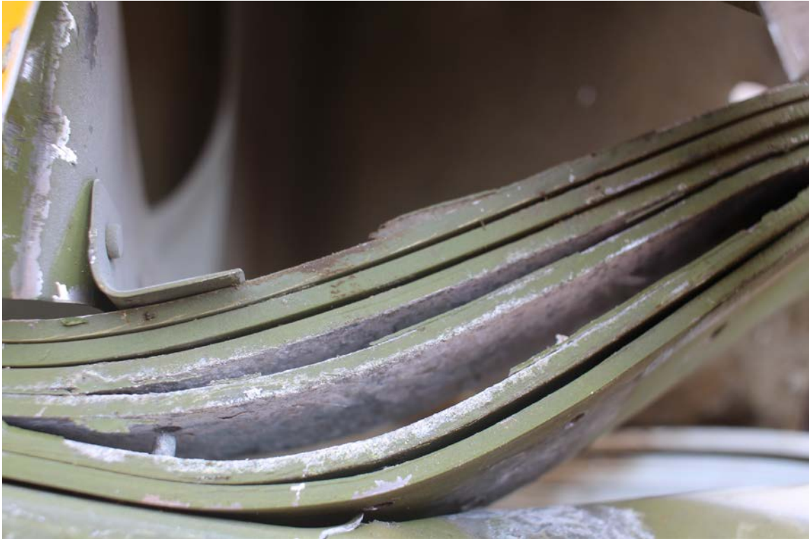
Figure 5 – Corrosion in left upper spar cap layers
