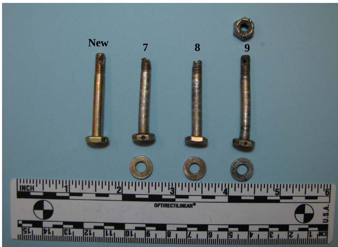
Figure 6 – New bolt and bolts removed from left lower spar cap
