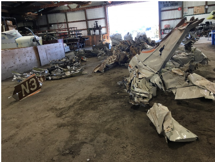
Photo 02 – Wreckage Layout (NTSB)
