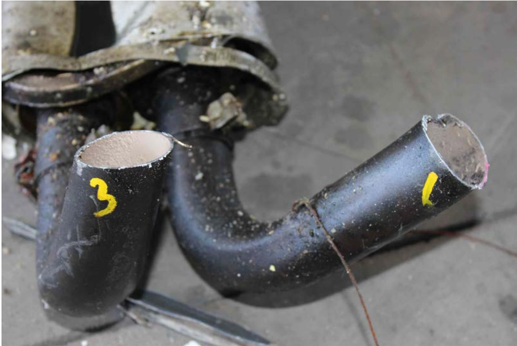
Photo 15 – Cylinder 1 and 3 Exhaust Pipes
