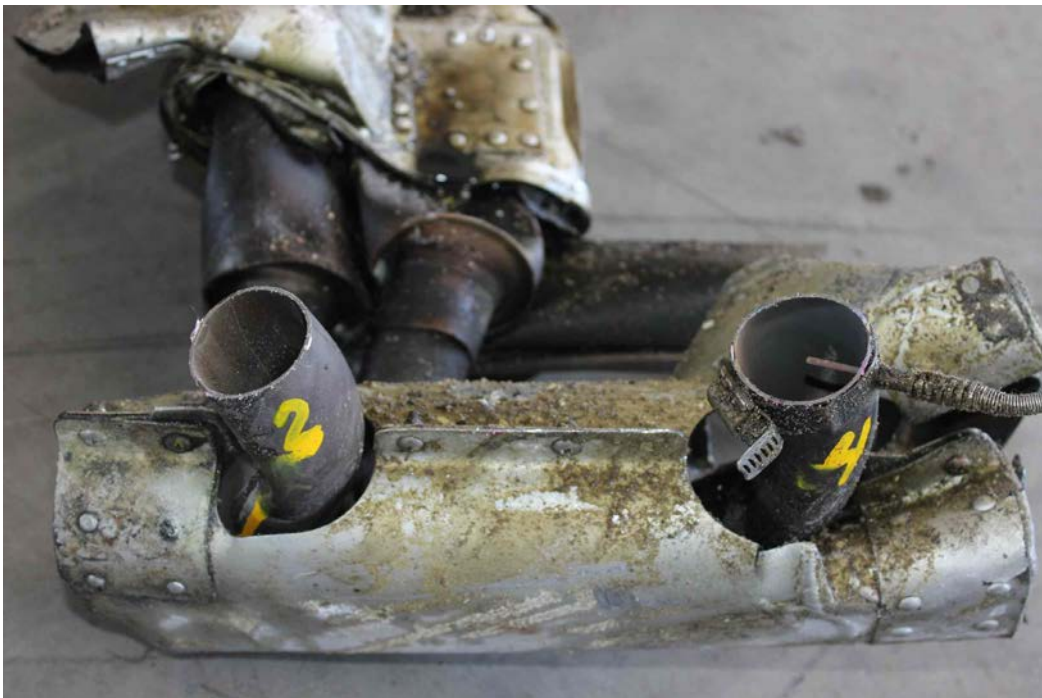
Photo 16 – Cylinder 2 and 4 Exhaust Pipes
