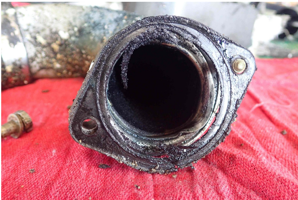
Photo 18 – Cylinder 3 Inlet Manifold Gasket
