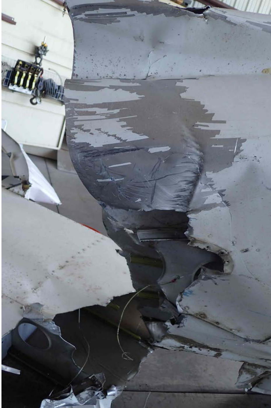
Photo 2 – Wire Striations on Right Wing
