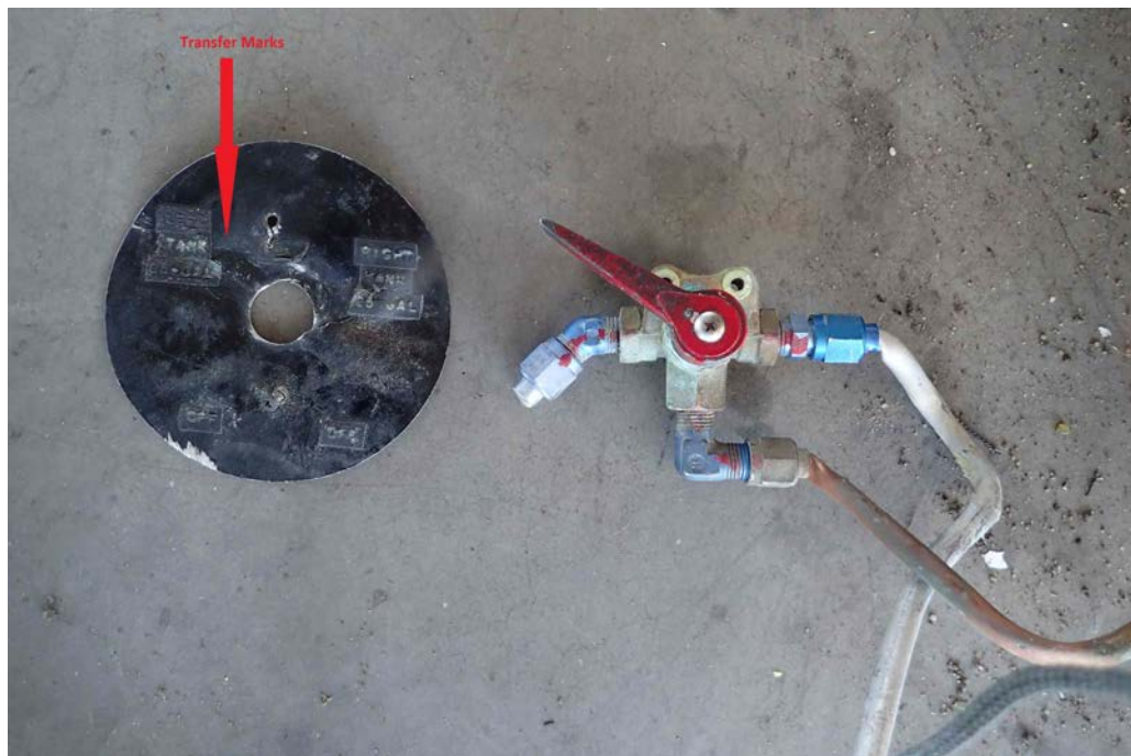
Photo 4 – Fuel Selector Valve and Backing Plate
