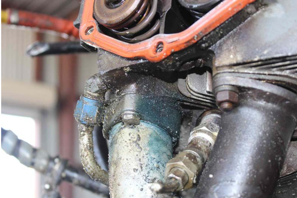
Photo 17 – Cylinder 3 Blue Staining at Inlet Manifold Pipe
