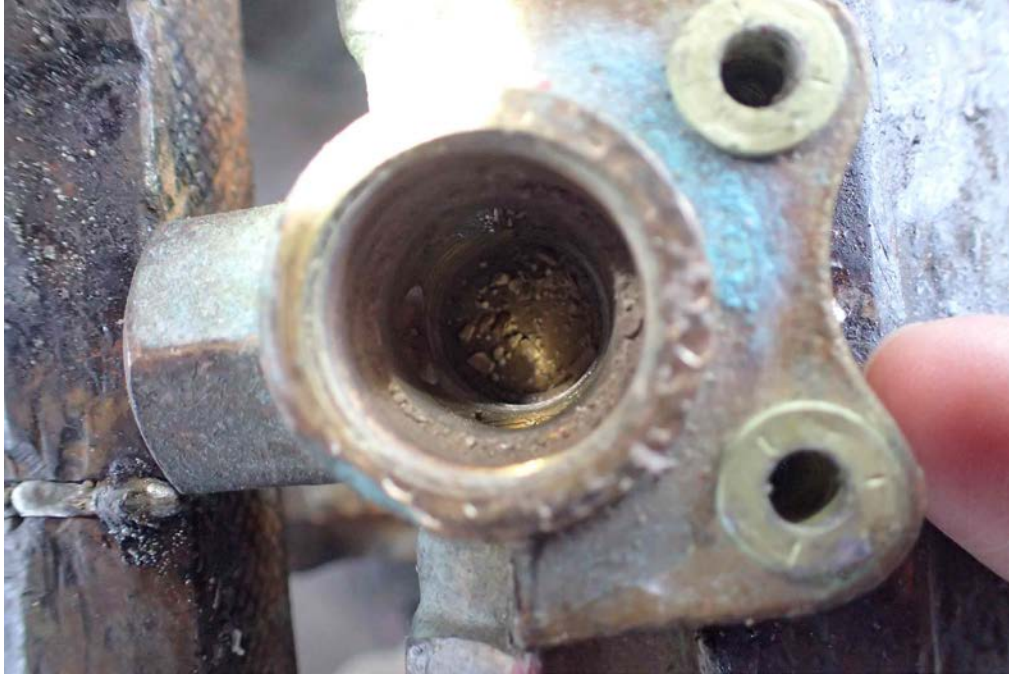
Photo 7 – Fuel Selector Valve Cavity
