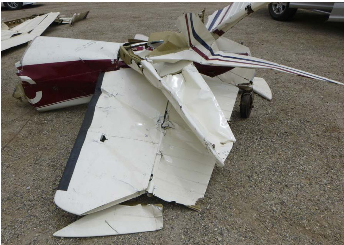
Figure 13 – Left side of empennage and left horizontal stabilizer
