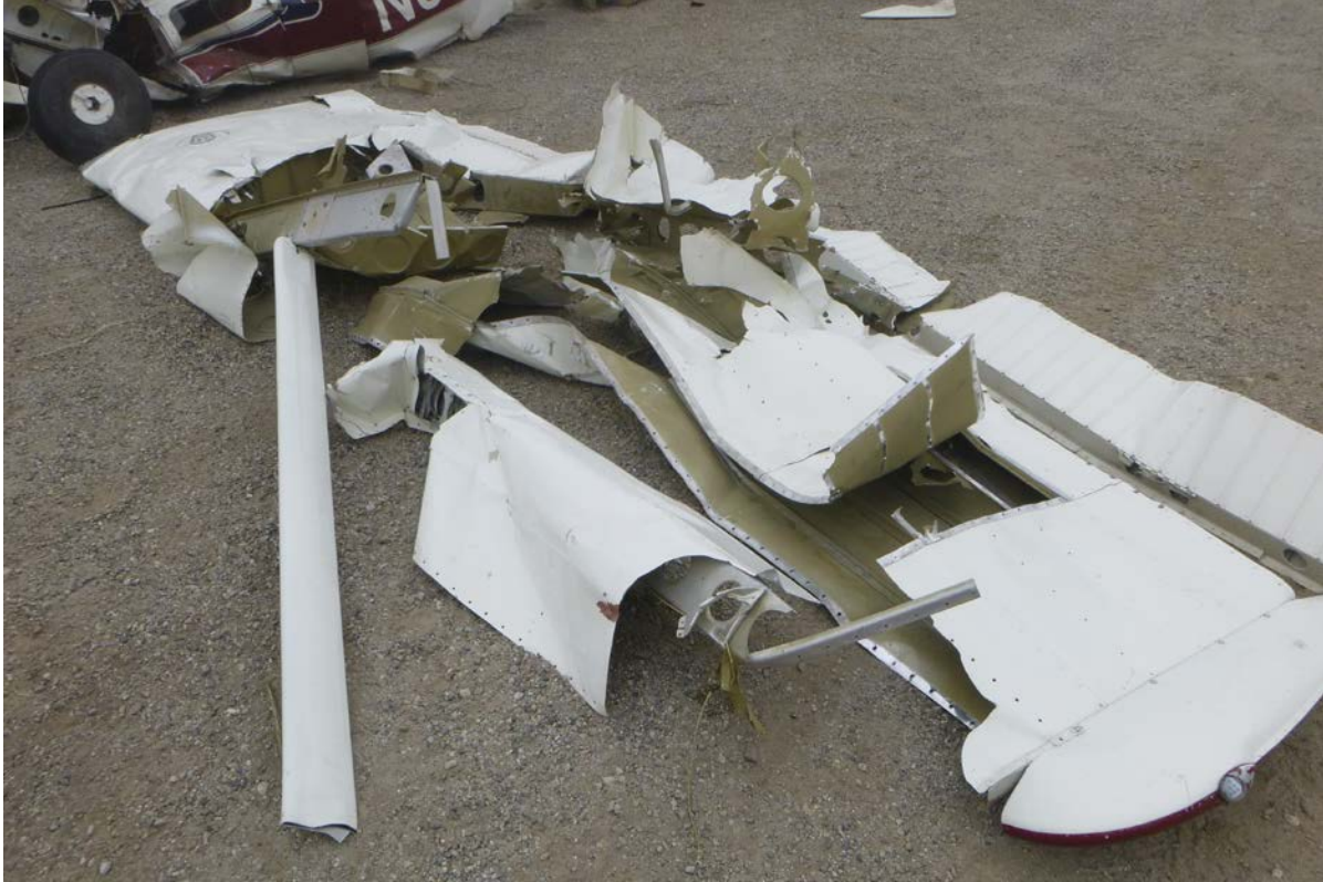
Figure 11 – Left wing wreckage
