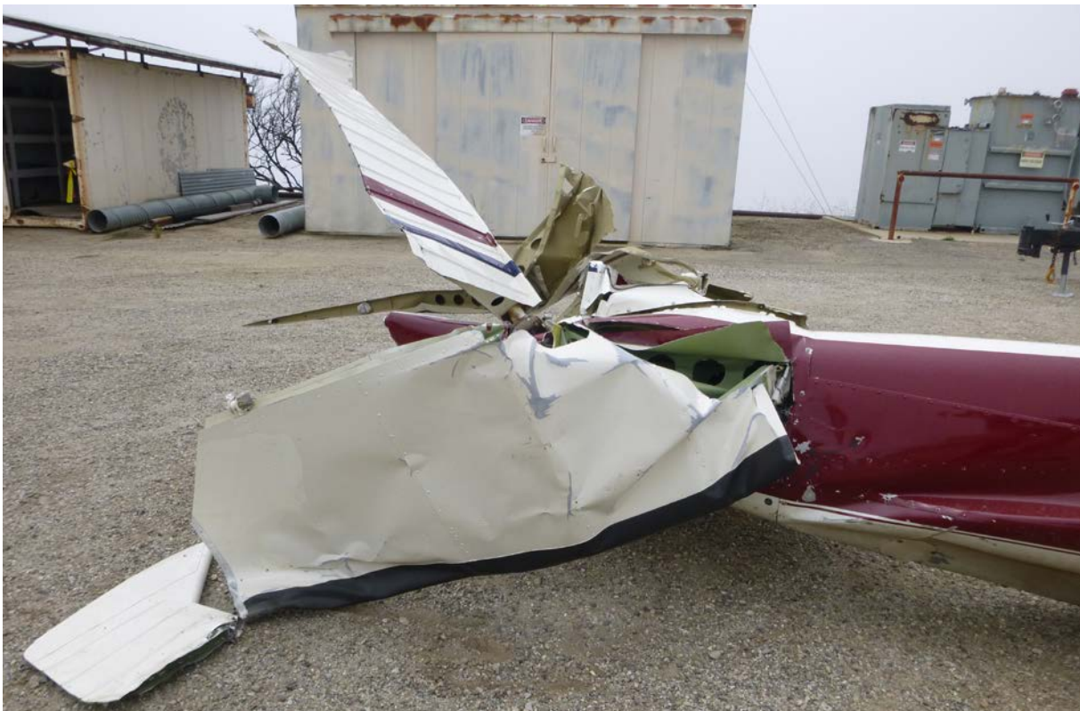
Figure 12 – Right side of empennage and right horizontal stabilizer
