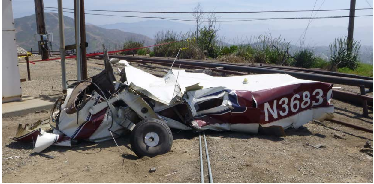
Figure 7 – Main fuselage wreckage
