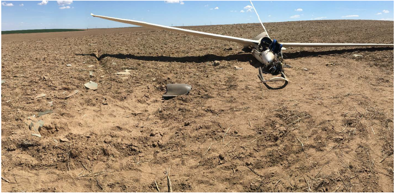
Figure 1: The First Identified Point of Impact in Relation to Glider
