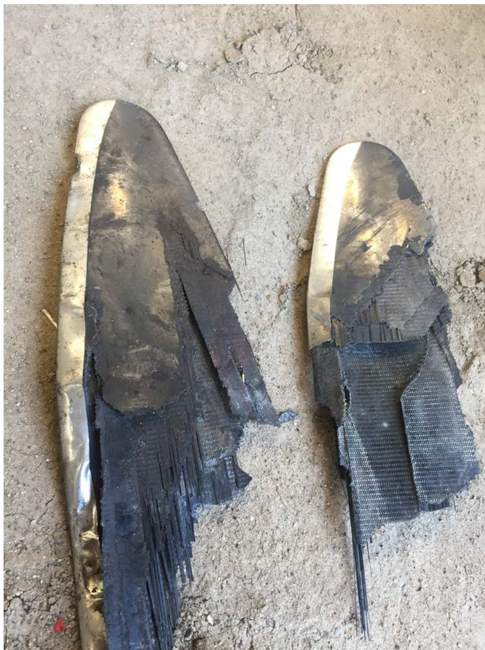
Photo 7 - Recovered propeller blades.
