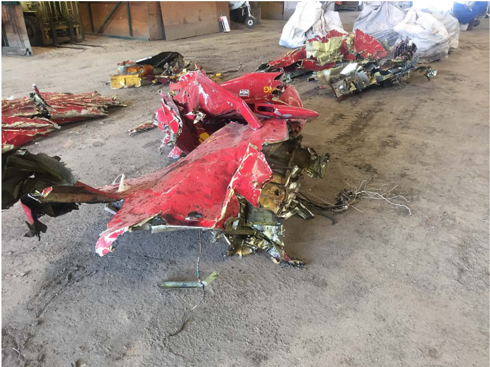
Photo 4 - View of the recovered wreckage / empennage.
