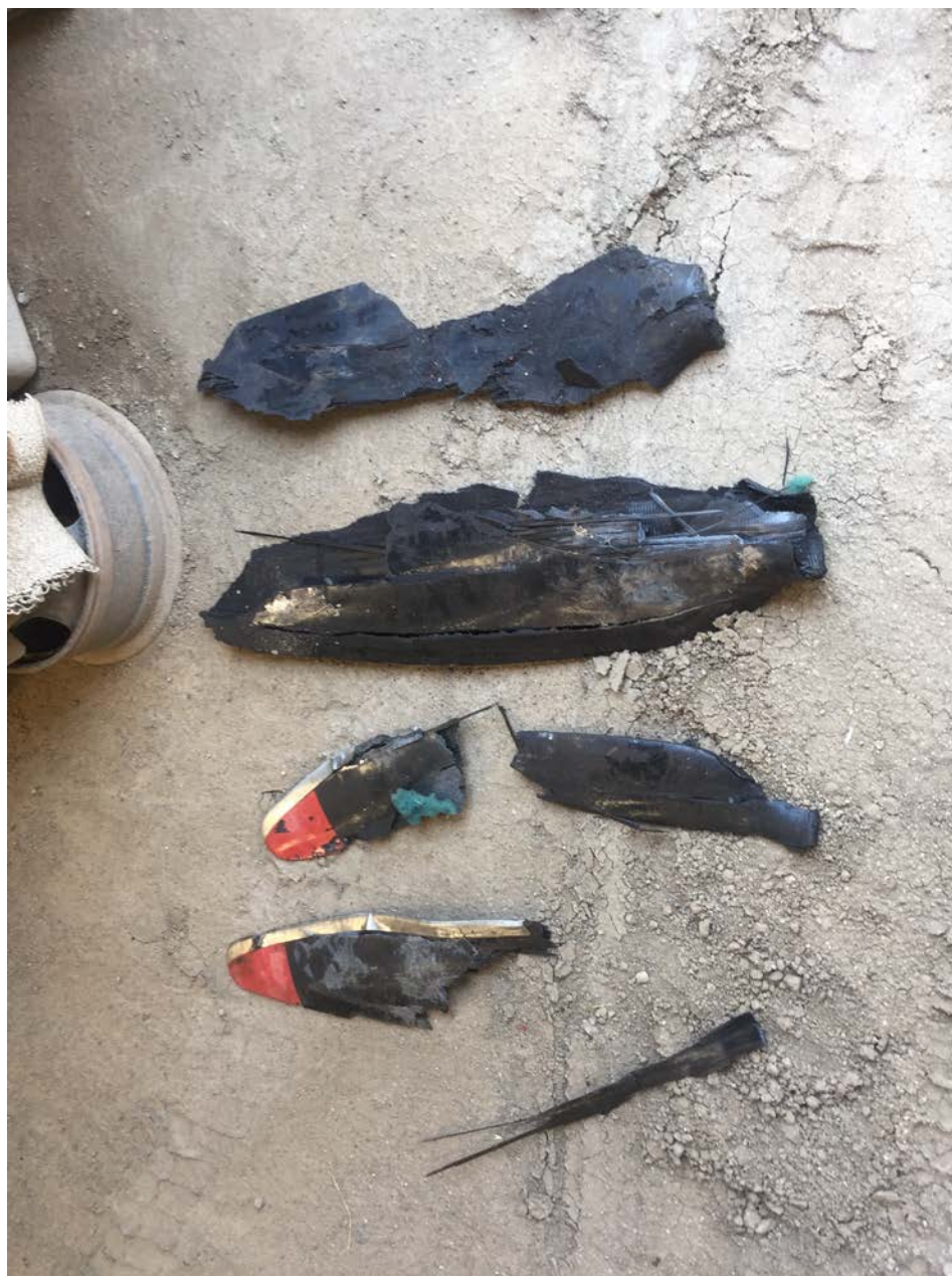
Photo 6 - Recovered propeller blades.
