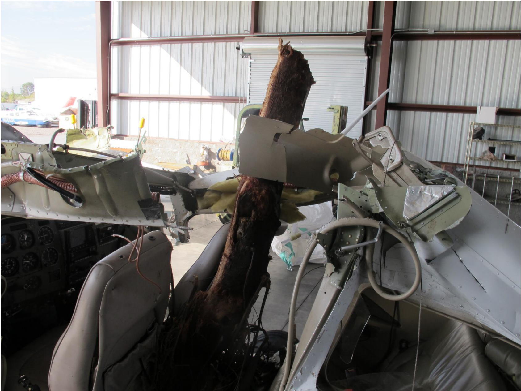
Photo 7 – Cabin Damage and Exit Point of Tree Limb
