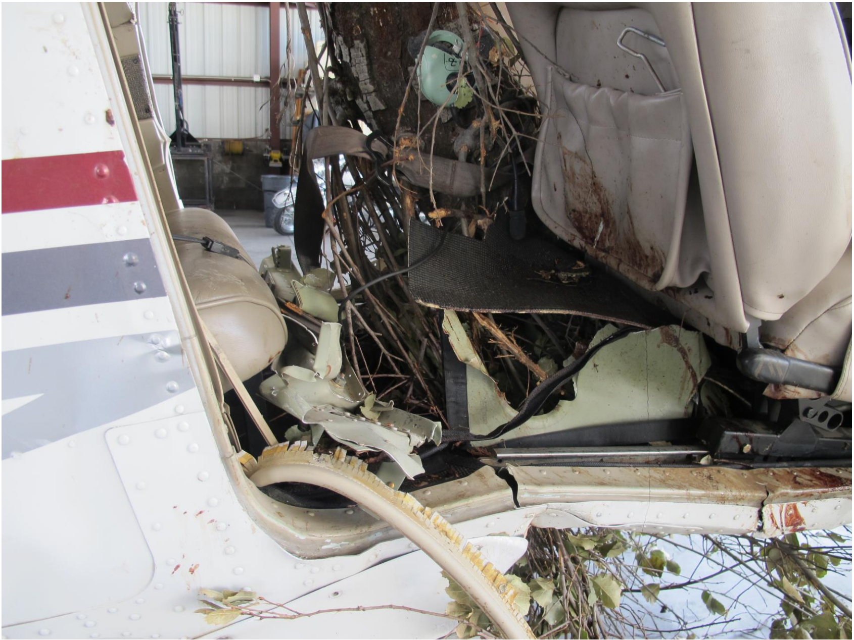
Photo 5 – Cabin Damage and Entry Point of Tree Limb
