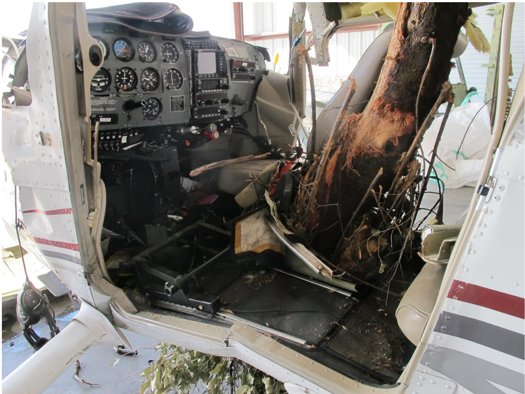
Photo 6 – Cabin Damage and Entry Point of Tree Limb
