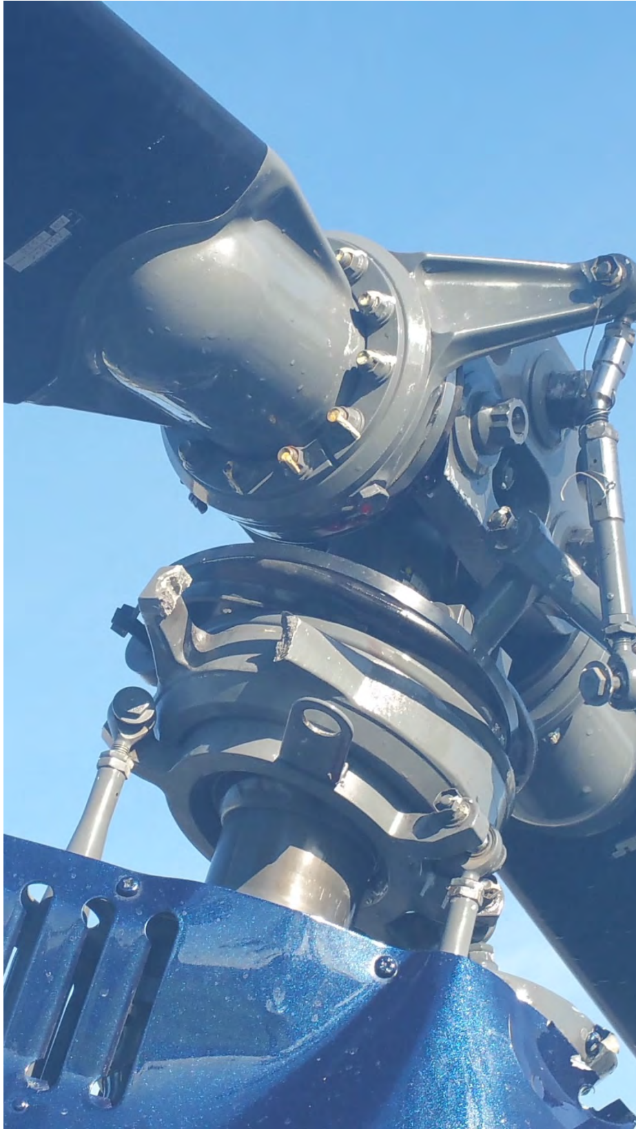
Photo 11 Main Rotor Hub
