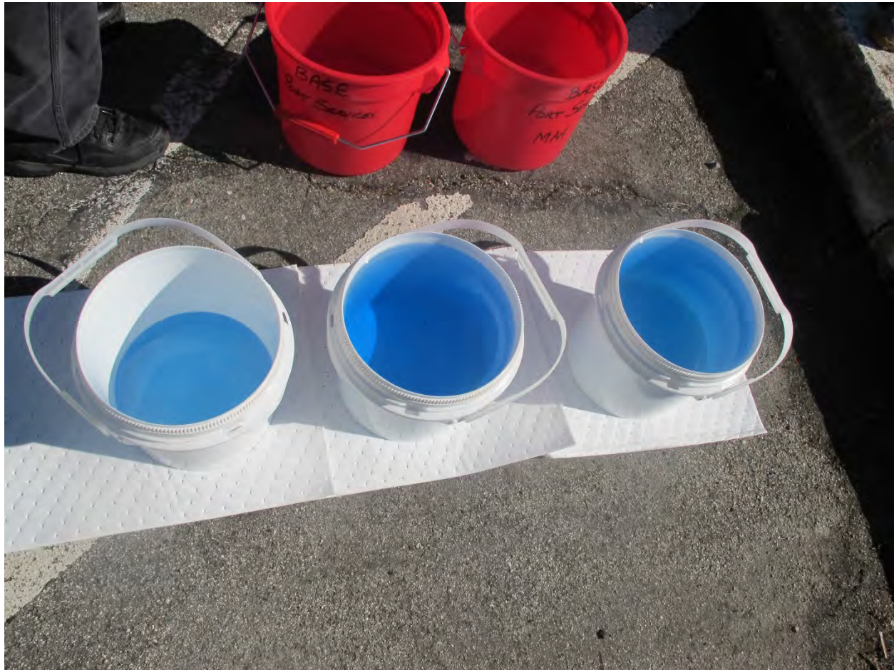
Photo 12 Drained Liquid from Fuel Tanks
