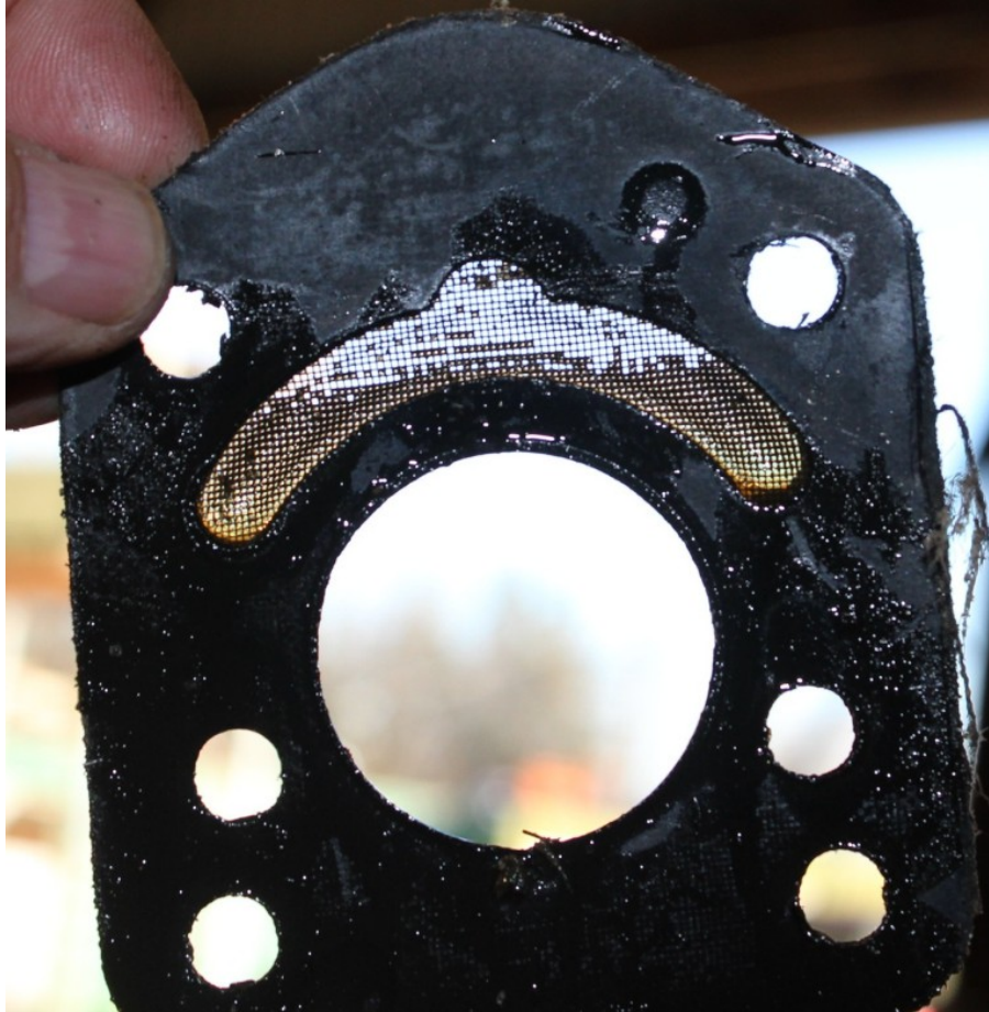
Figure 68 - Propeller Governor Screen
