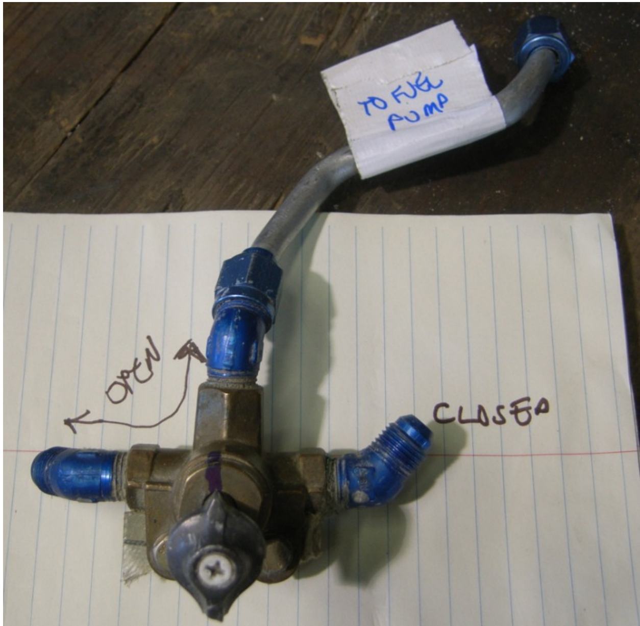
Figure 32 - Excised Fuel Selector Valve
