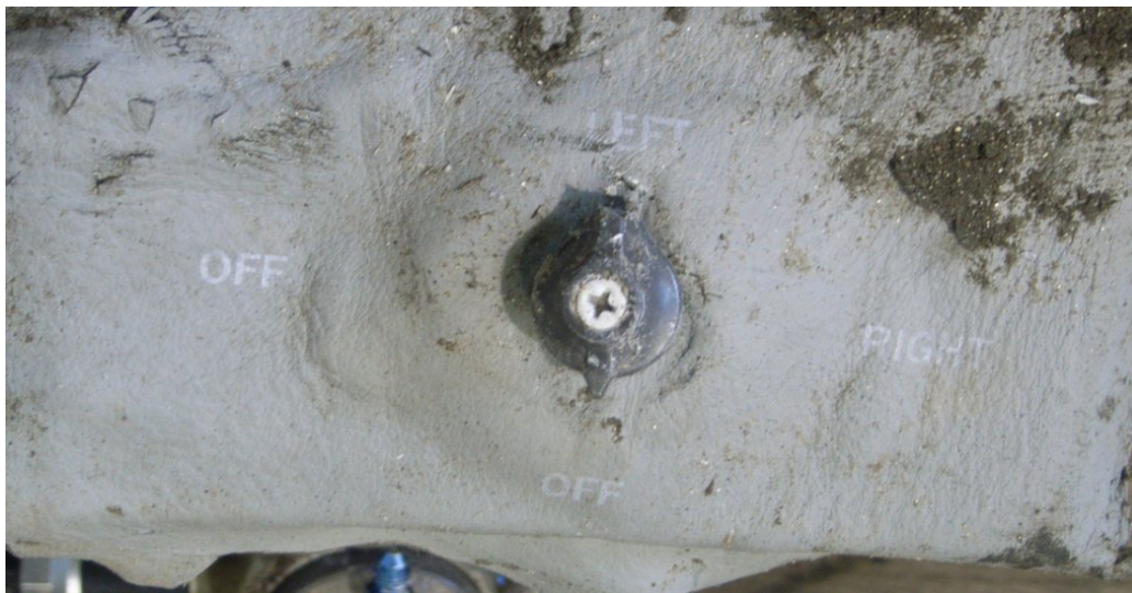
Figure 30 - Cockpit Fuel Selector Panel with Fractured Handle
