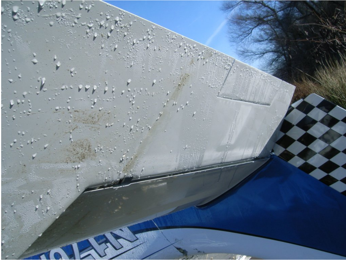
Figure 19 - Right Horizontal Stabilizer with Trim Tab
