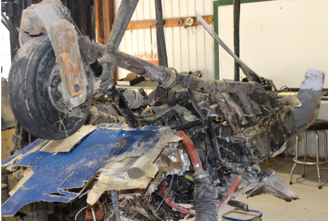
Figure 36 - Nose Gear Attached to Inverted Engine
