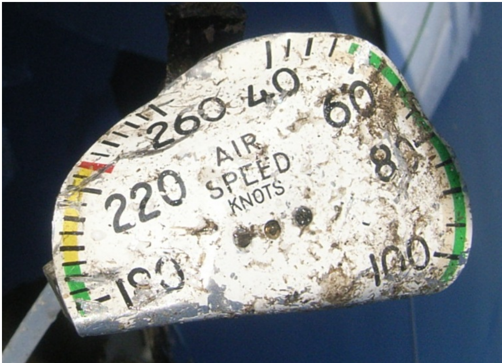
Figure 34 - Upper Face of Airspeed Indicator
