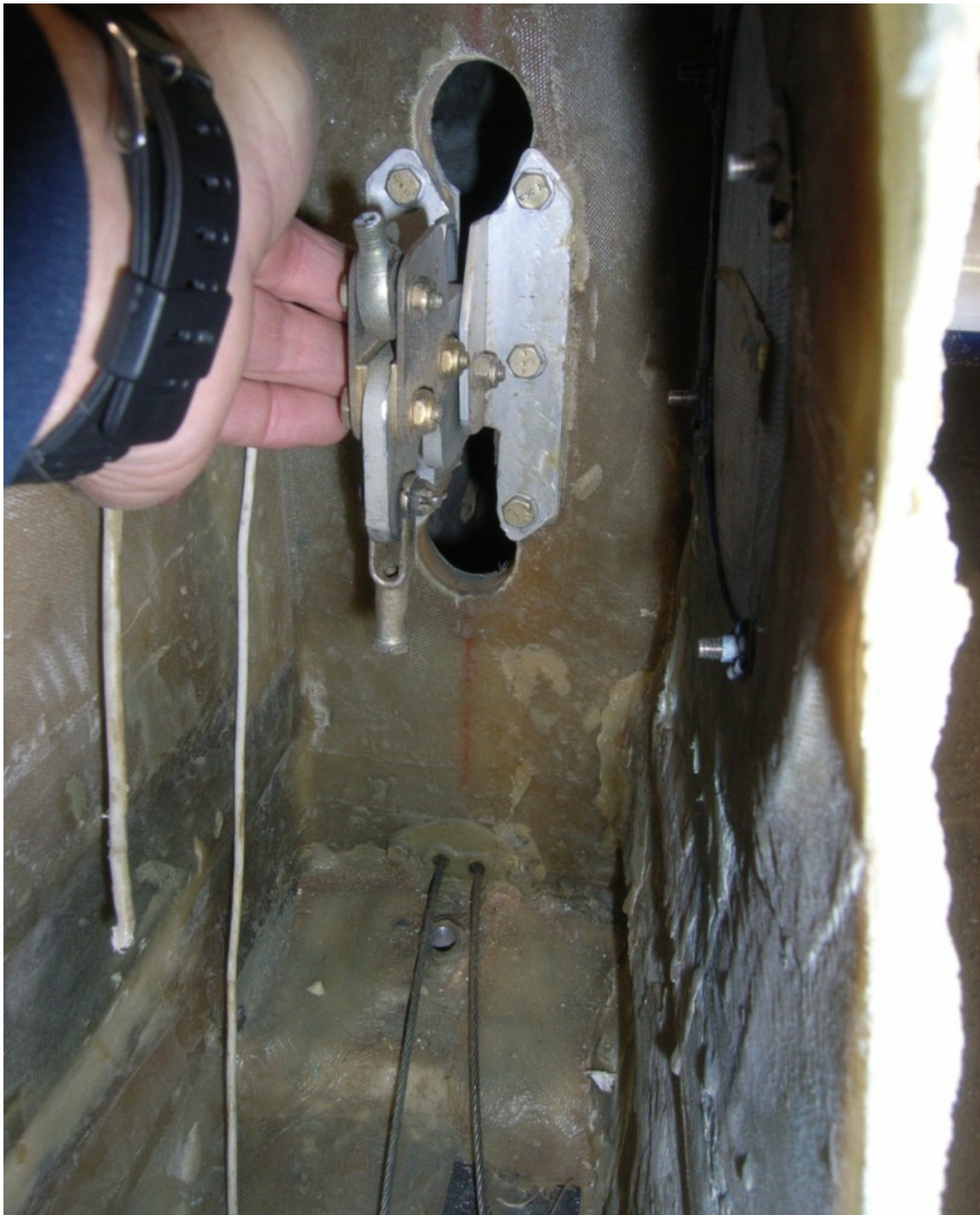
Figure 15 - Elevator Bellcrank Assembly
