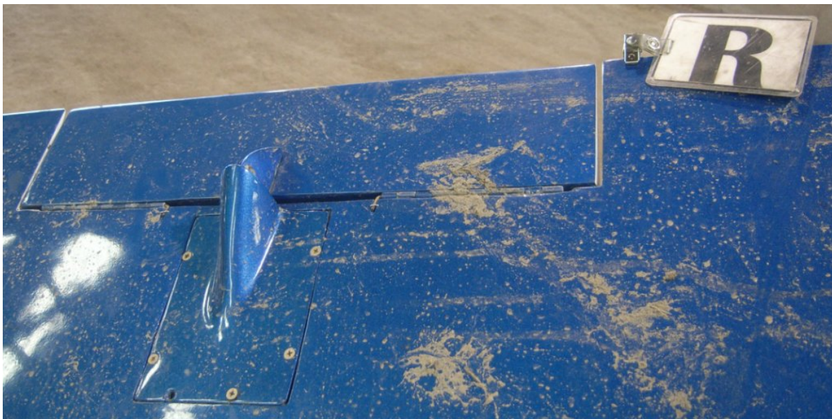
Figure 20 – Pitch Trim Tab with Actuator Fairing
