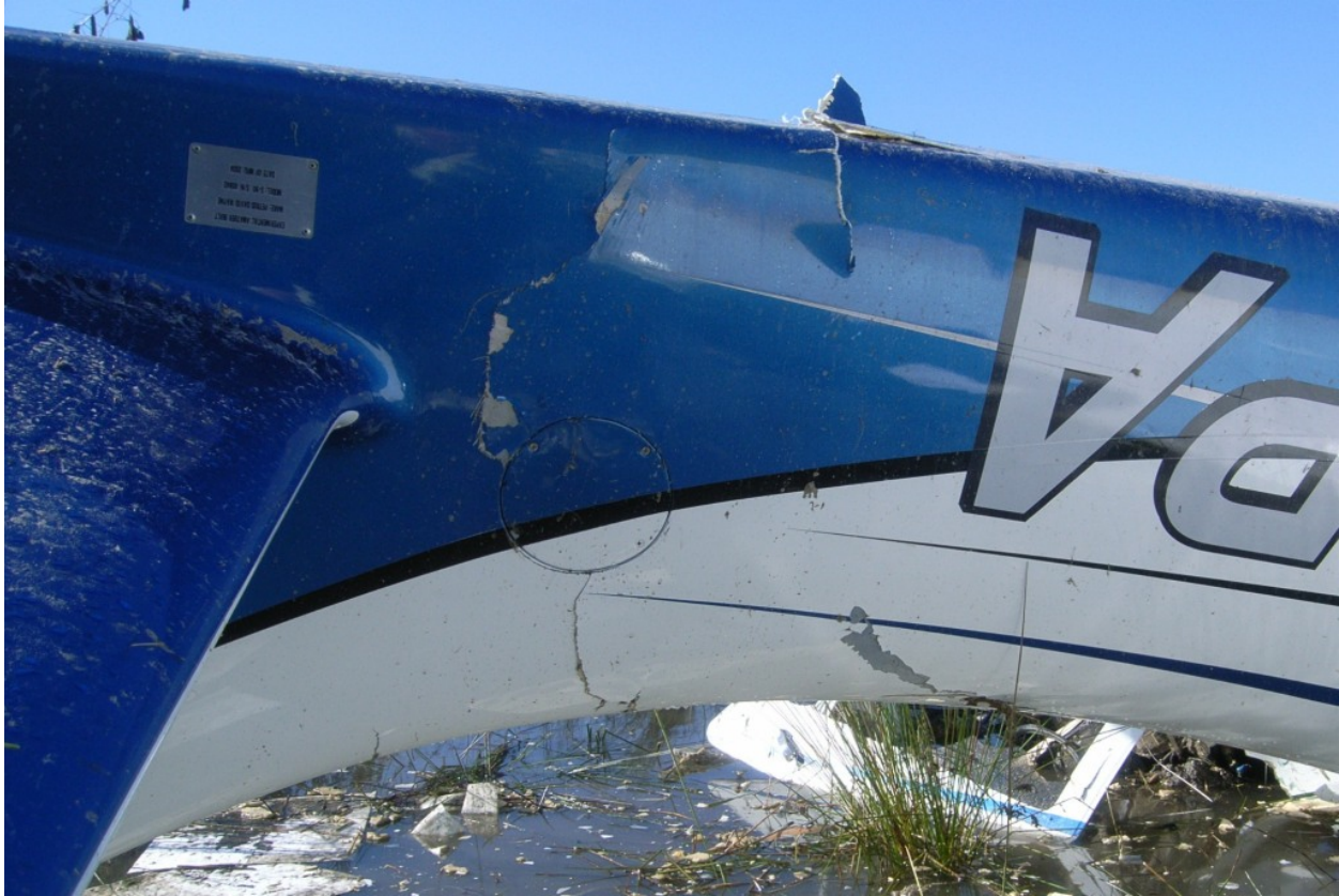
Figure 13 - Circumferential Crack on Aft Fuselage
