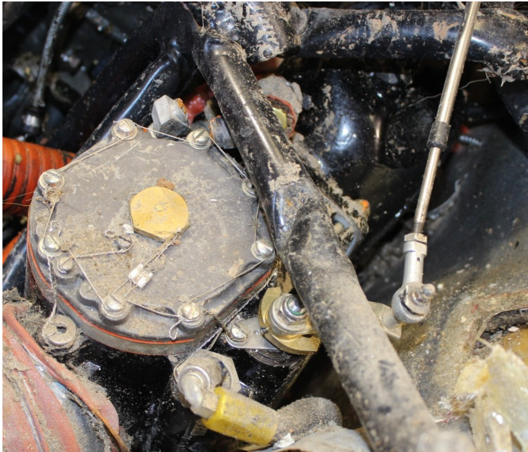
Figure 60 – Partially Attached Fuel Servo
