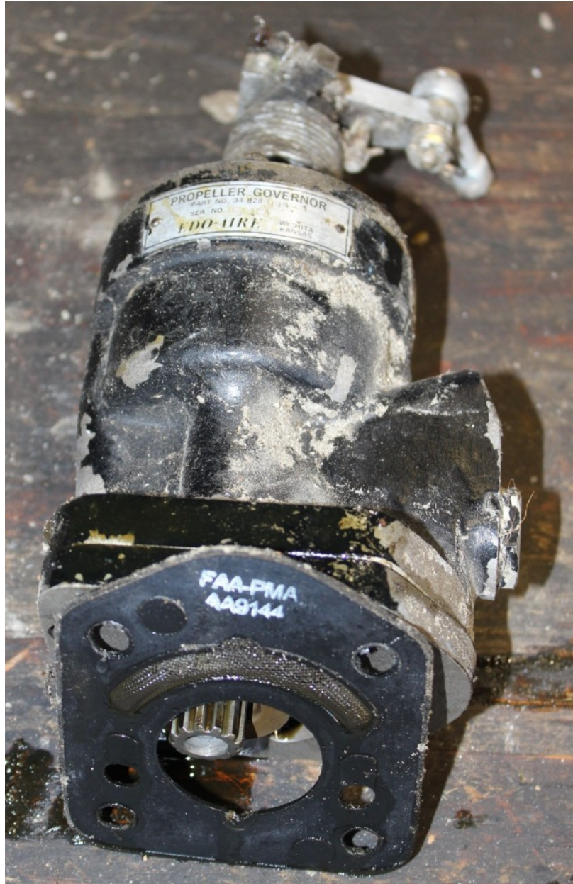
Figure 67 - Removed Propeller Governor
