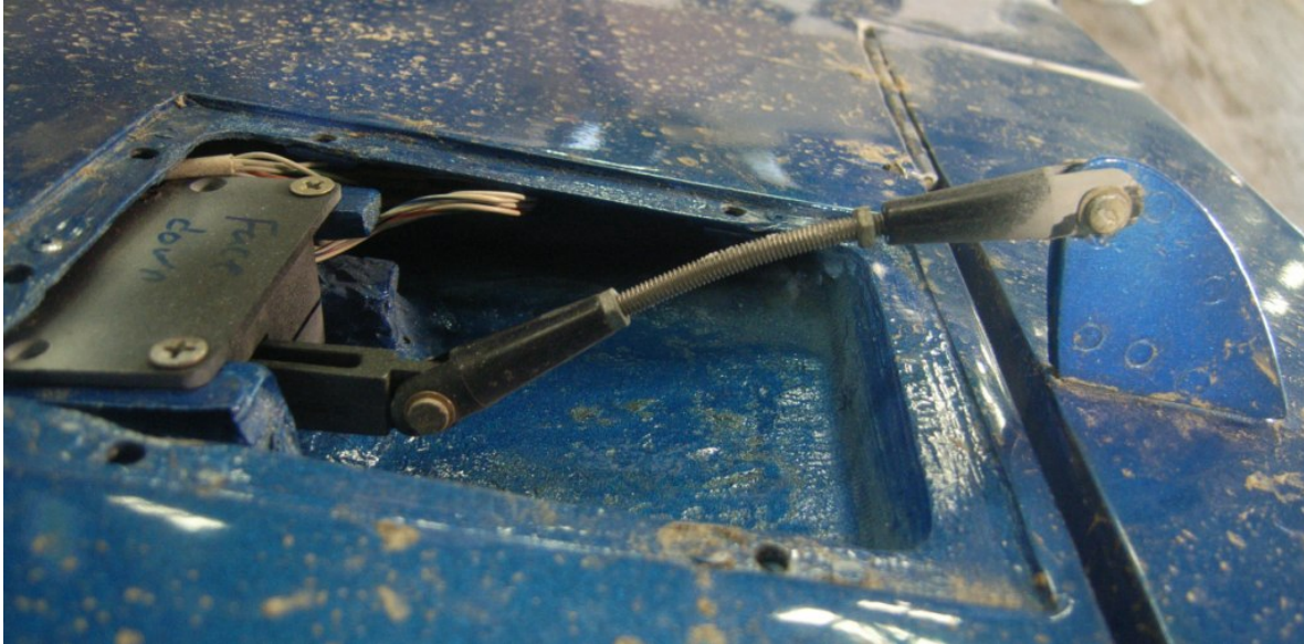
Figure 21 - Pitch Trim Tab and Actuator
