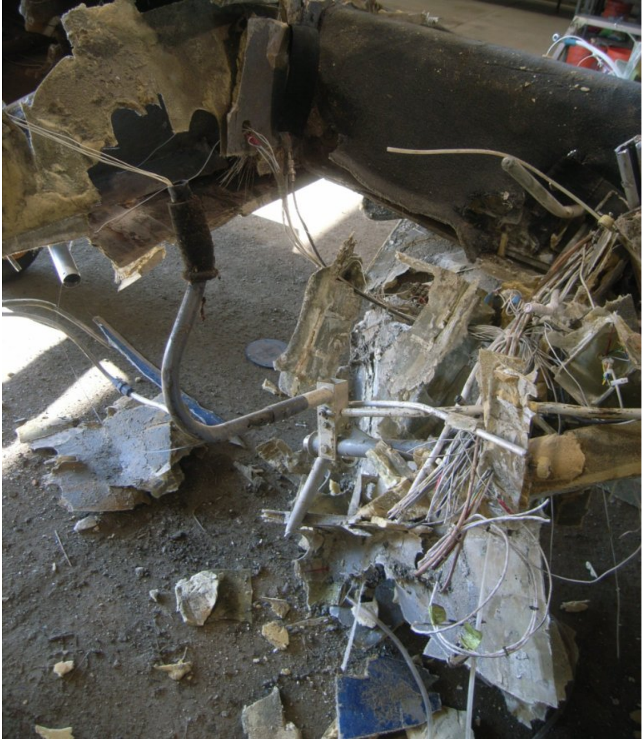
Figure 24 - Center Section with Flight Control Segments
