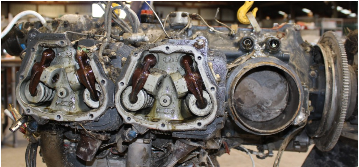
Figure 52 - Right Cylinder Bank Rocker Assemblies
