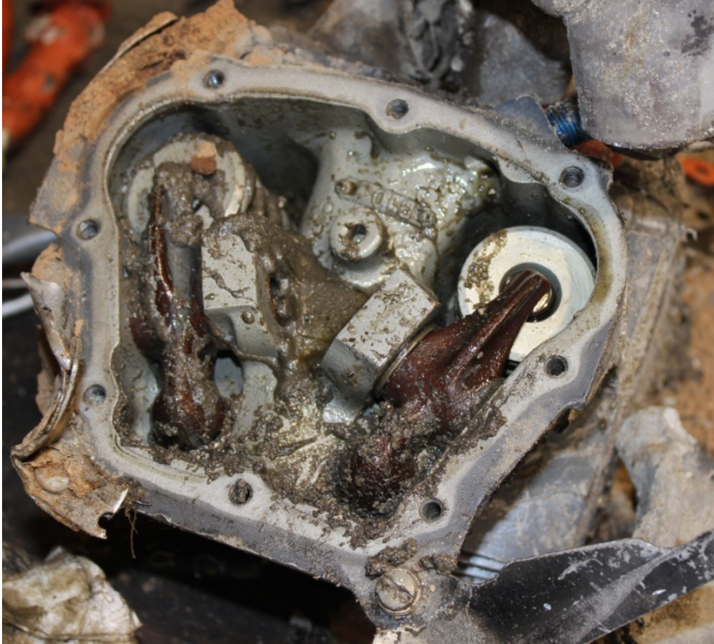
Figure 53 – No. 1 Cylinder Rocker Assembly
