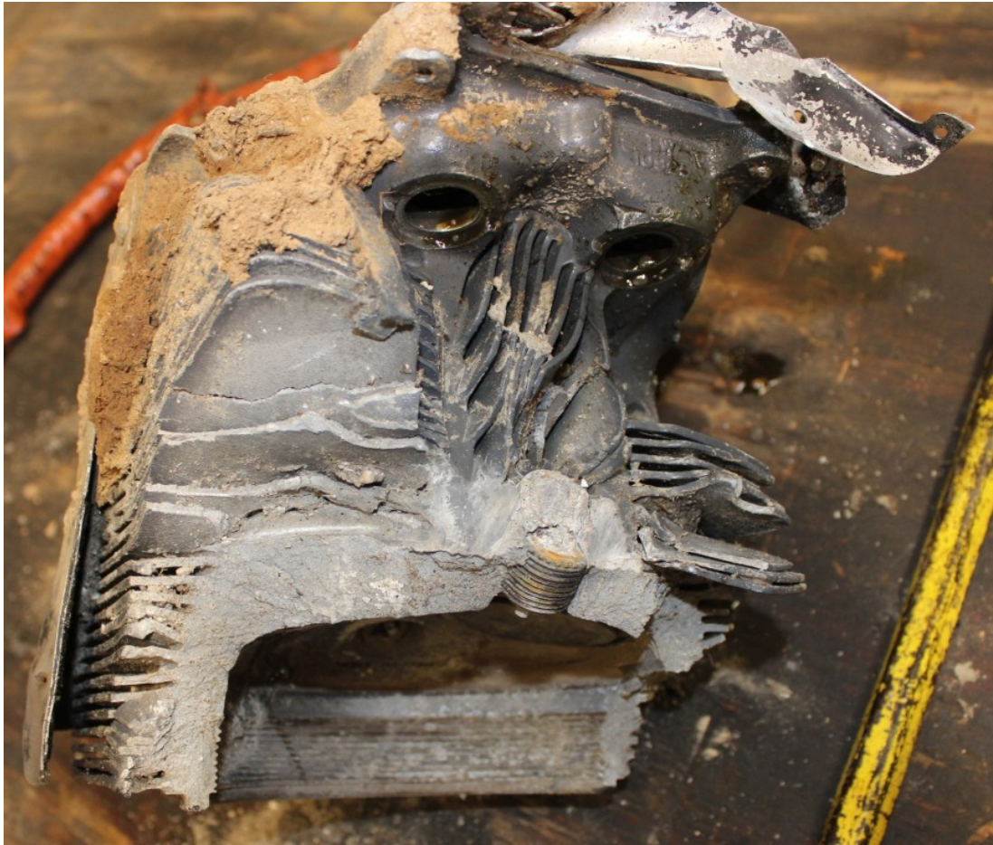
Figure 50 - Propeller-Separated Portion of No 1 Cylinder
