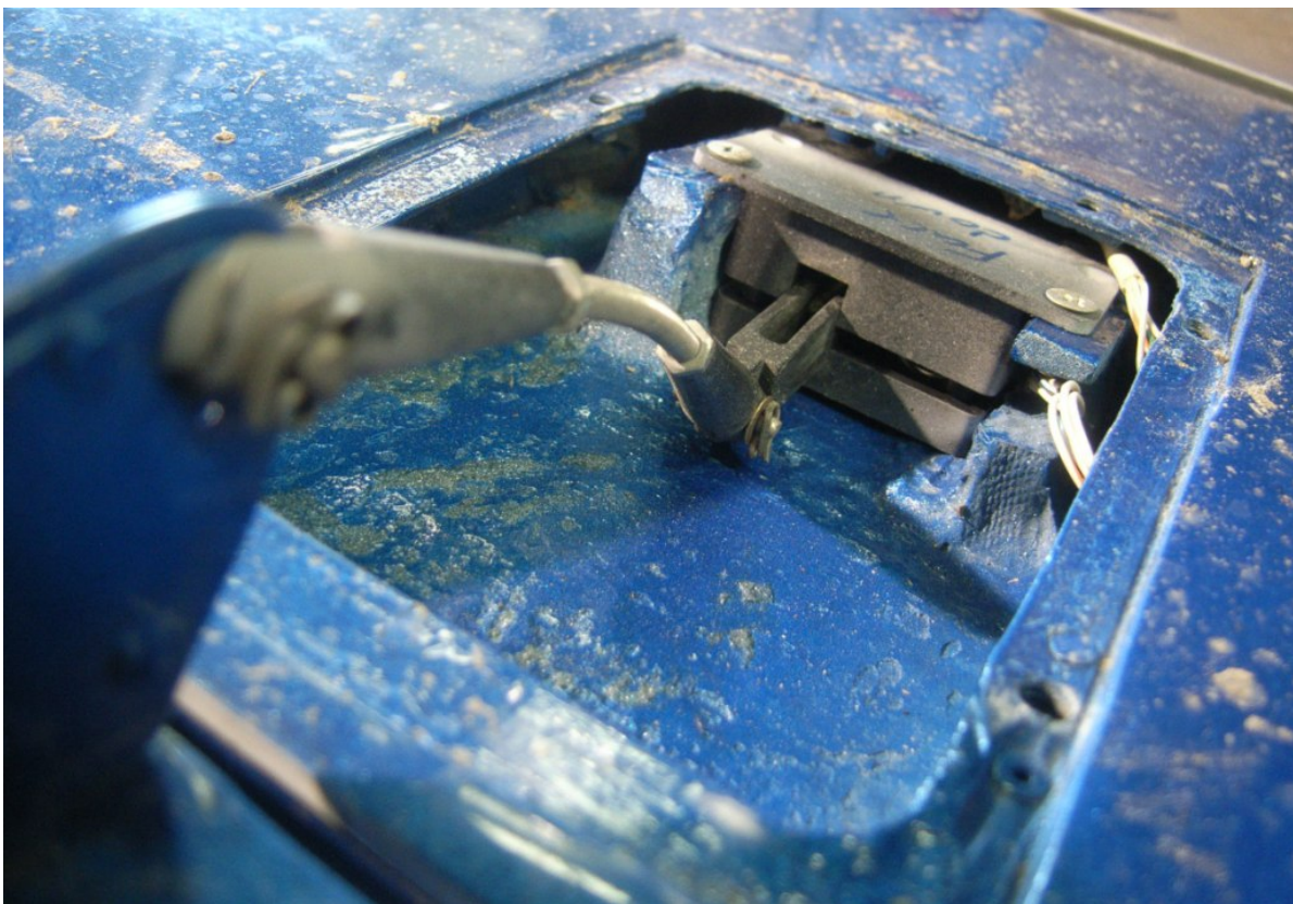
Figure 22 - Pitch Trim Actuator and Rod
