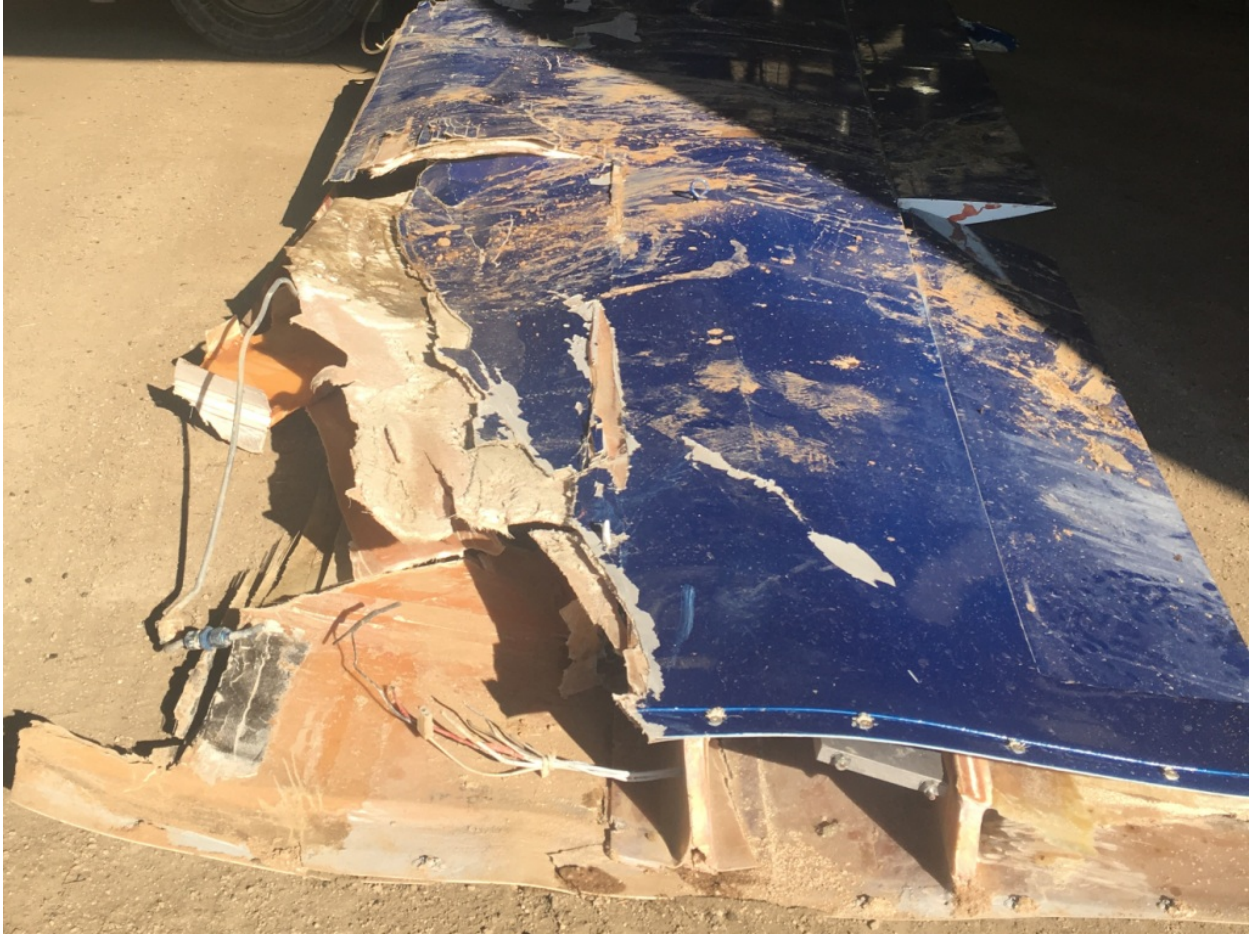
Figure 12 - Non-Displaced Right Aileron Weights (wing inverted)
