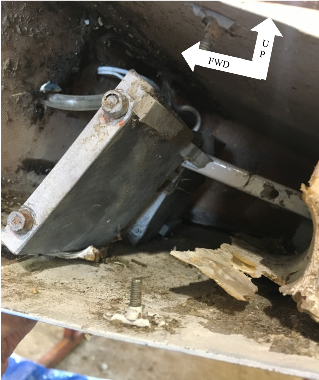
Figure 11 - Displaced Left Aileron Weights (looking inbd)
