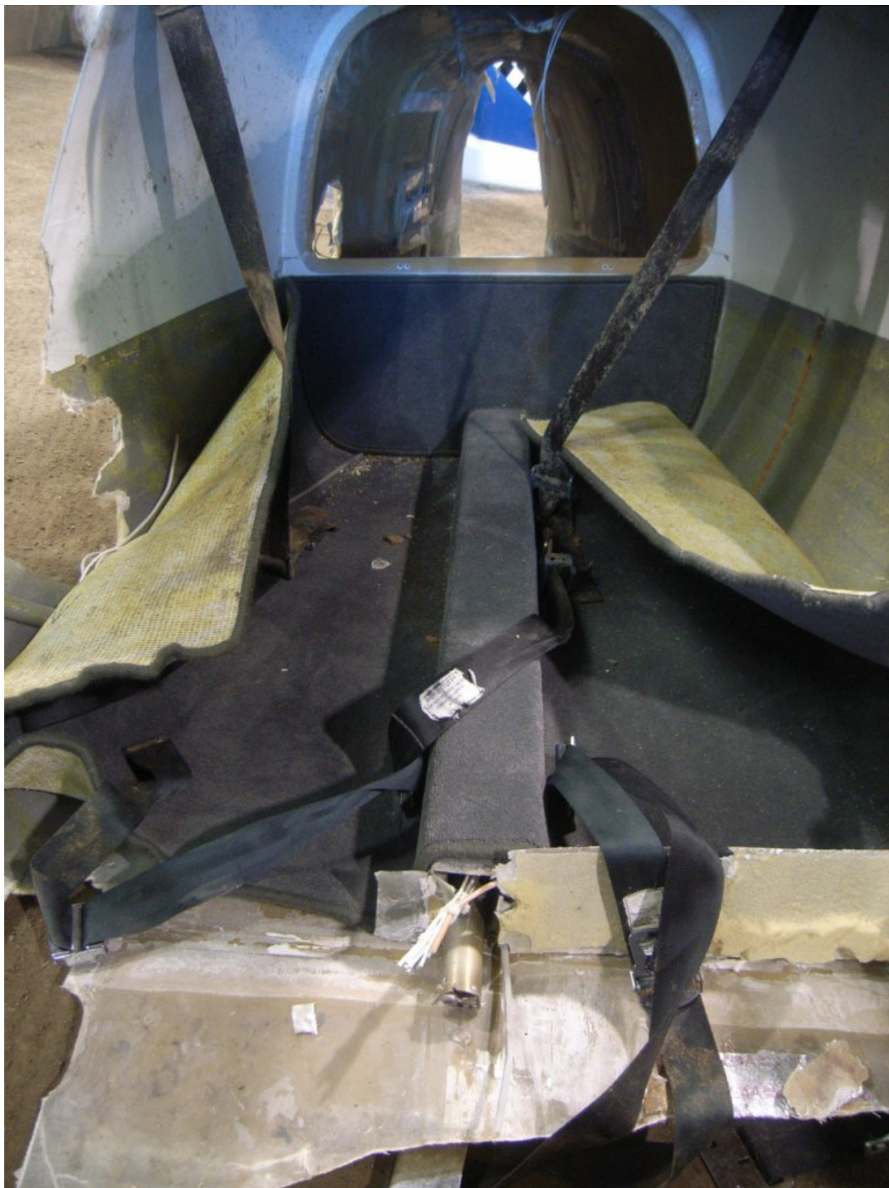
Figure 16 - Aft Fuselage with Elevator Control Rod
