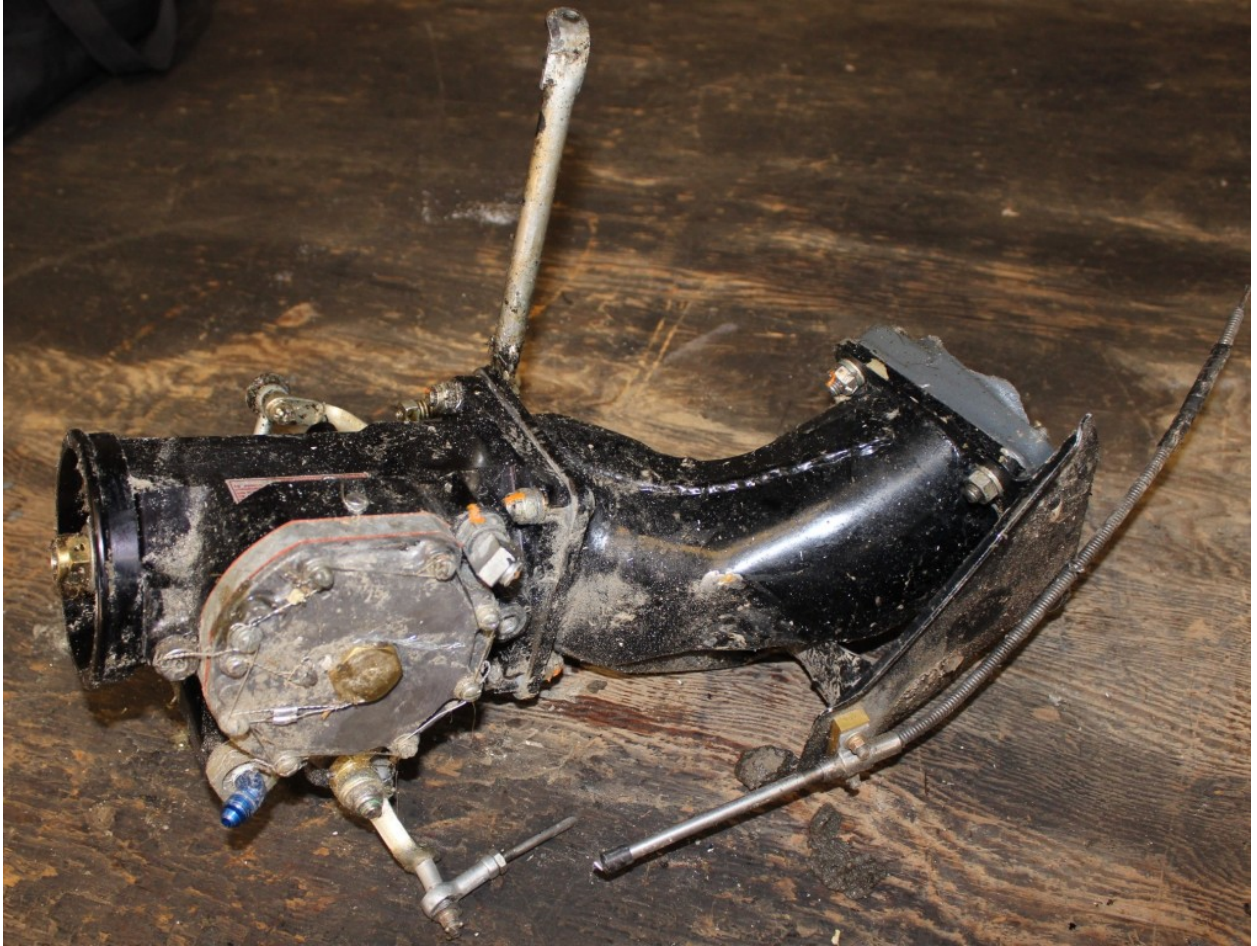
Figure 61 - Removed Fuel Servo
