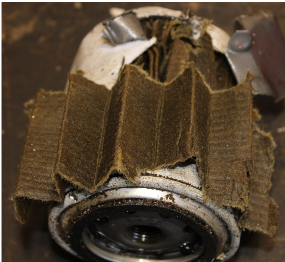
Figure 55 - External Oil Filter Internal Filter Element
