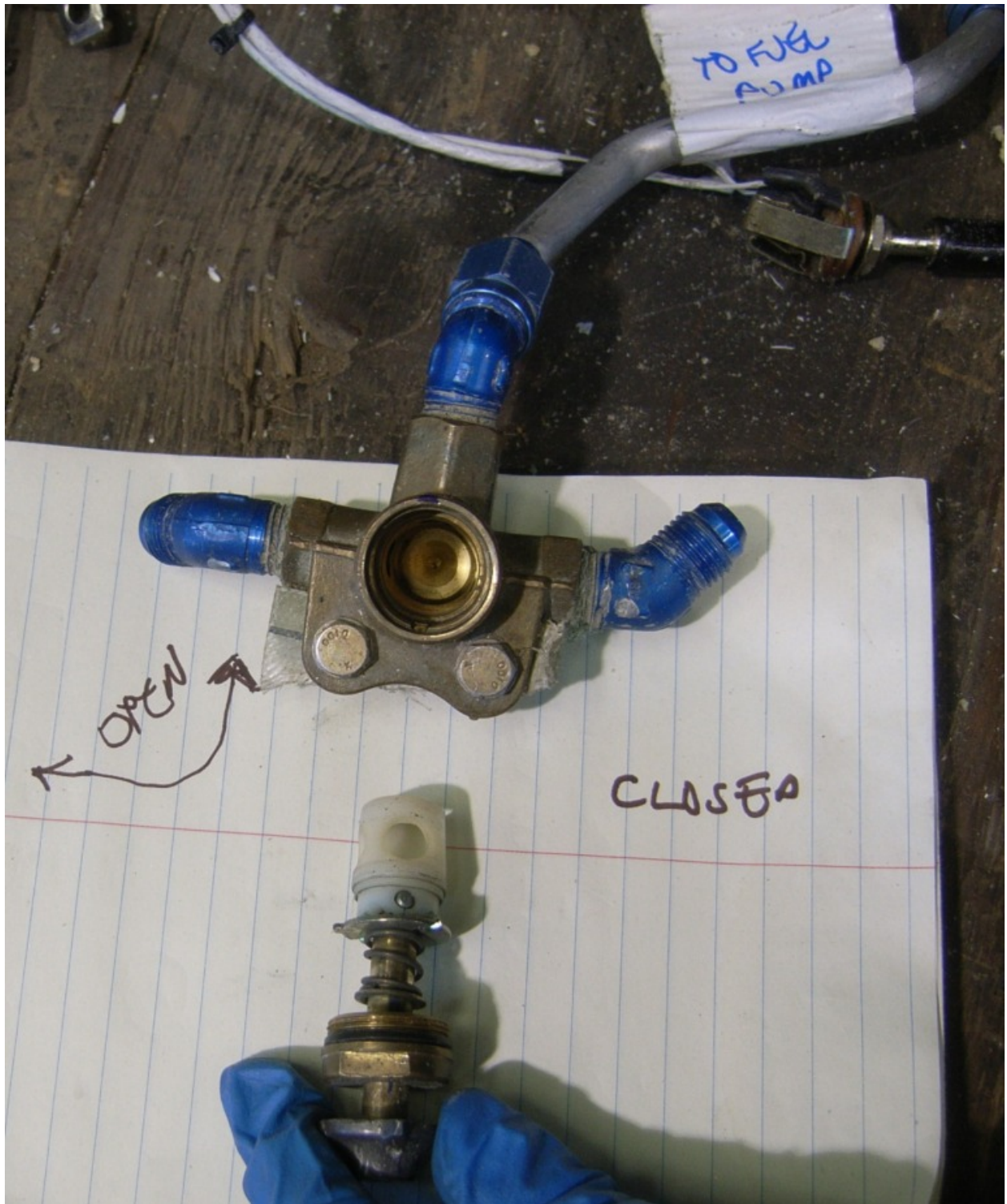
Figure 33 - Fuel Selector Valve Internals
