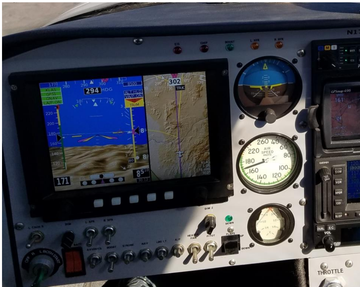
Figure 1 - PFD/EFIS and Pneumatic ASI Comparison
