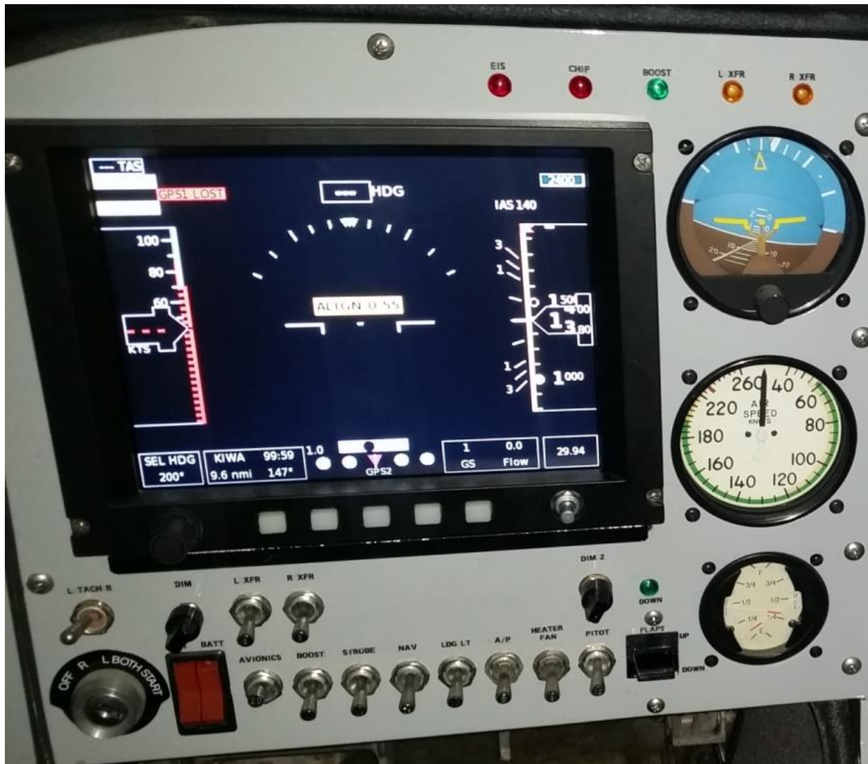
Figure 2 – PFD/EFIS ASI Bar with White Flap Range
