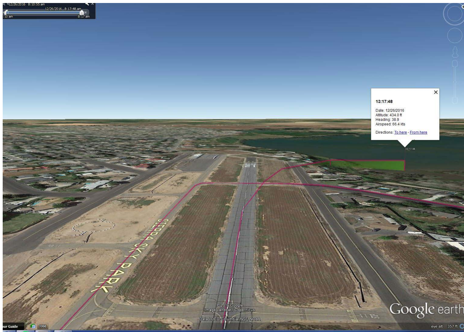
Figure 2. Google Earth overlay showing last 20 seconds of accident flight
