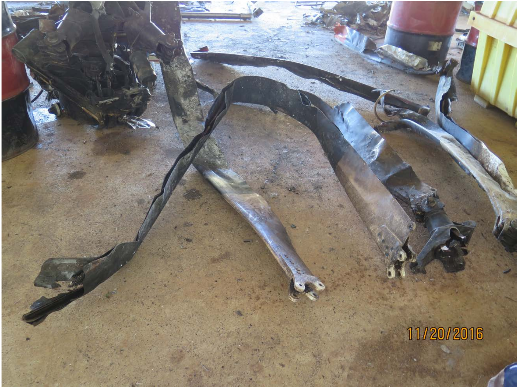
Photo 10 - Five recovered main rotor blades
