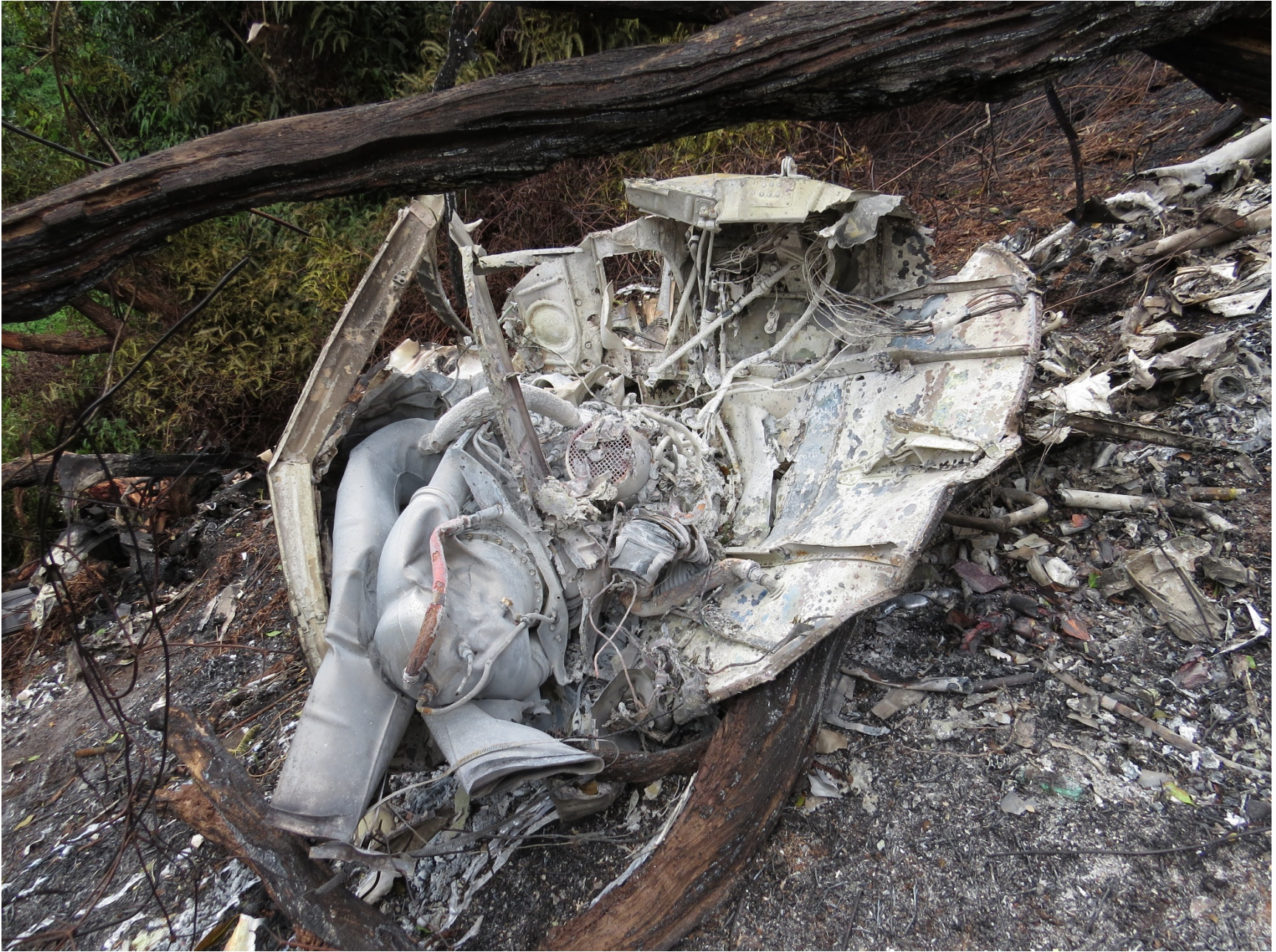
Photo 4 - Rolls Royce (Allison) 250-C20B engine at accident site
