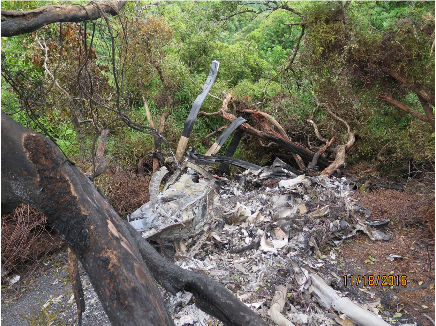
Photo 3 - Main rotor and transmission assembly
