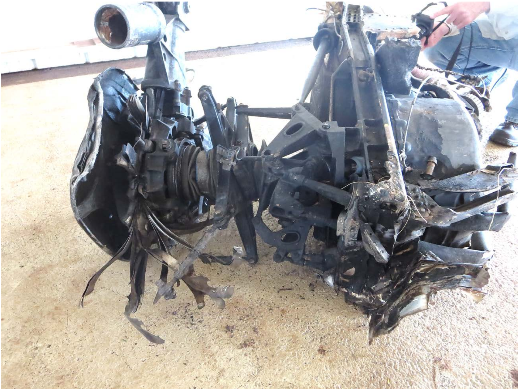
Photo 8 - Main rotor head and transmission
