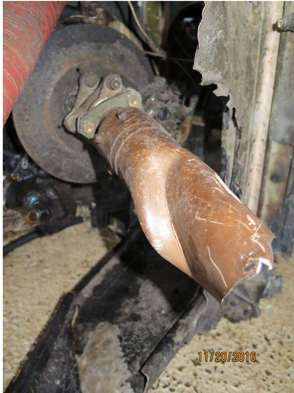
Photo 6 - Tail rotor drive shaft with fracture and torsional deformation
