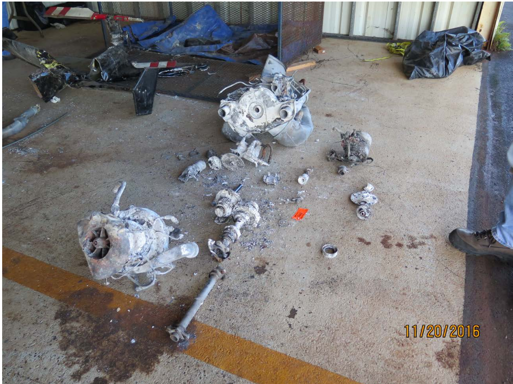
Photo 9 - Rolls Royce 250-C20B engine with drive shafts, pinion gear and couplings
