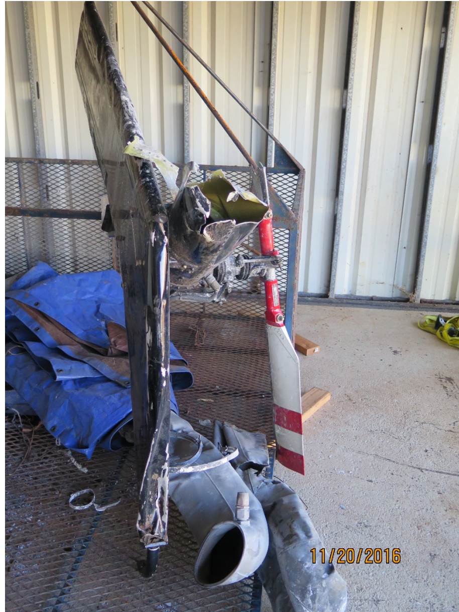
Photo 11-Tail rotor and vertical stabilizer assembly
