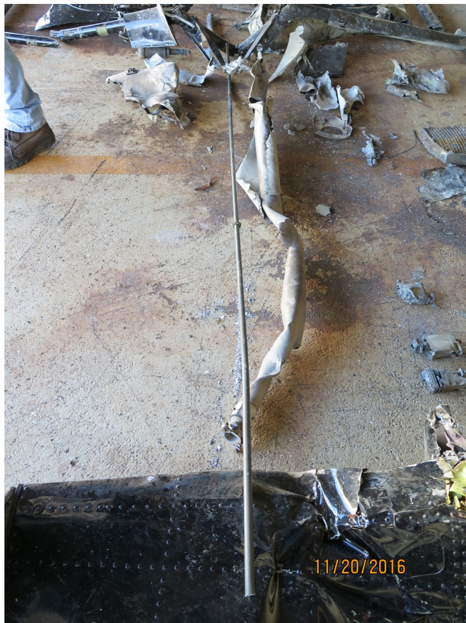
Photo 7 - Fractured and twisted tail rotor drive shaft
