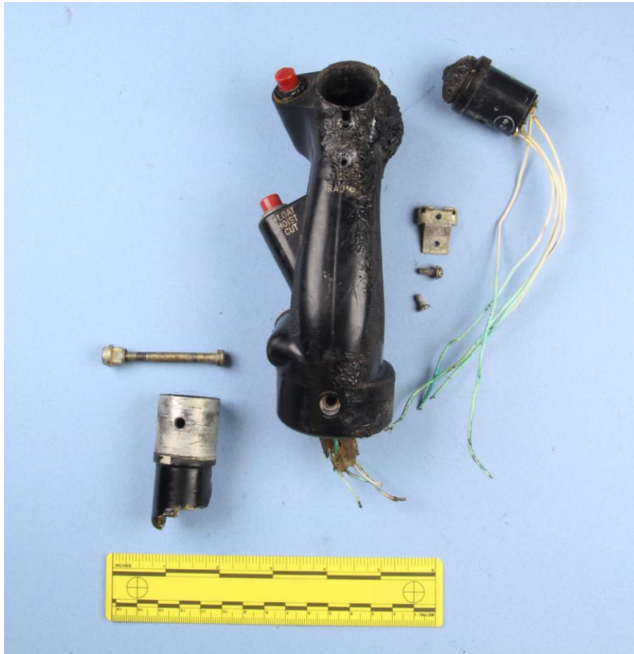
Figure 2: Cyclic grip after partial disassembly to remove the trim switch.
