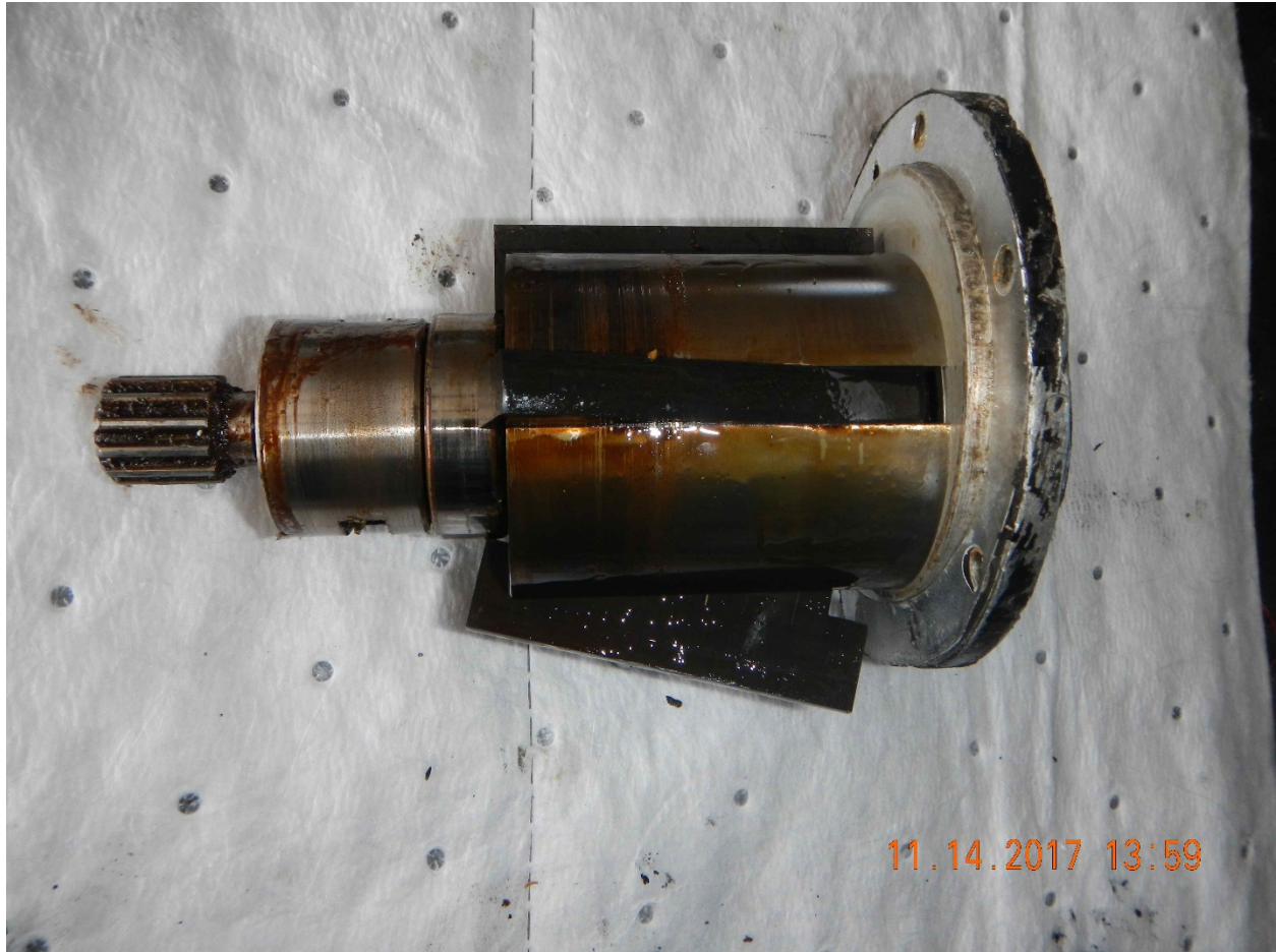
Photo 13 – Vacuum Pump Rotor
