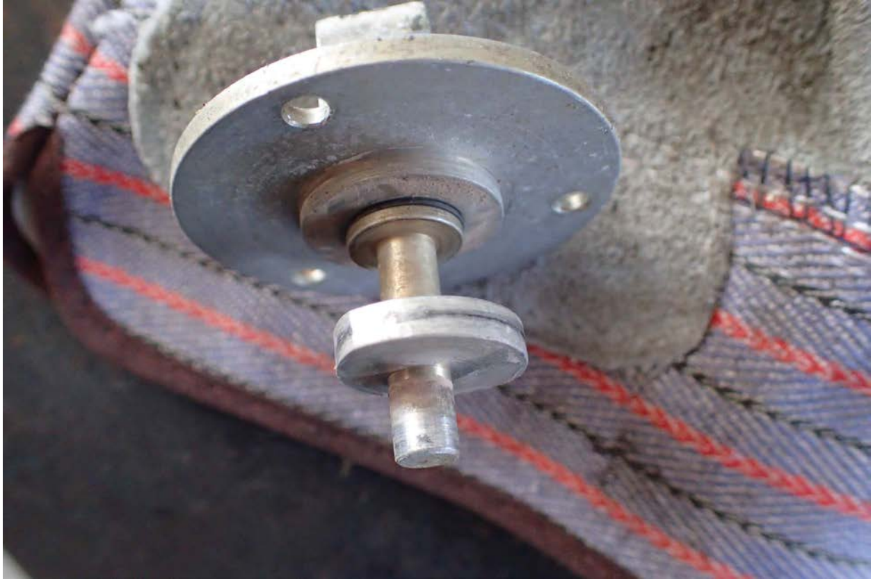
Photo 6 – Fuel Selector Valve Cam
