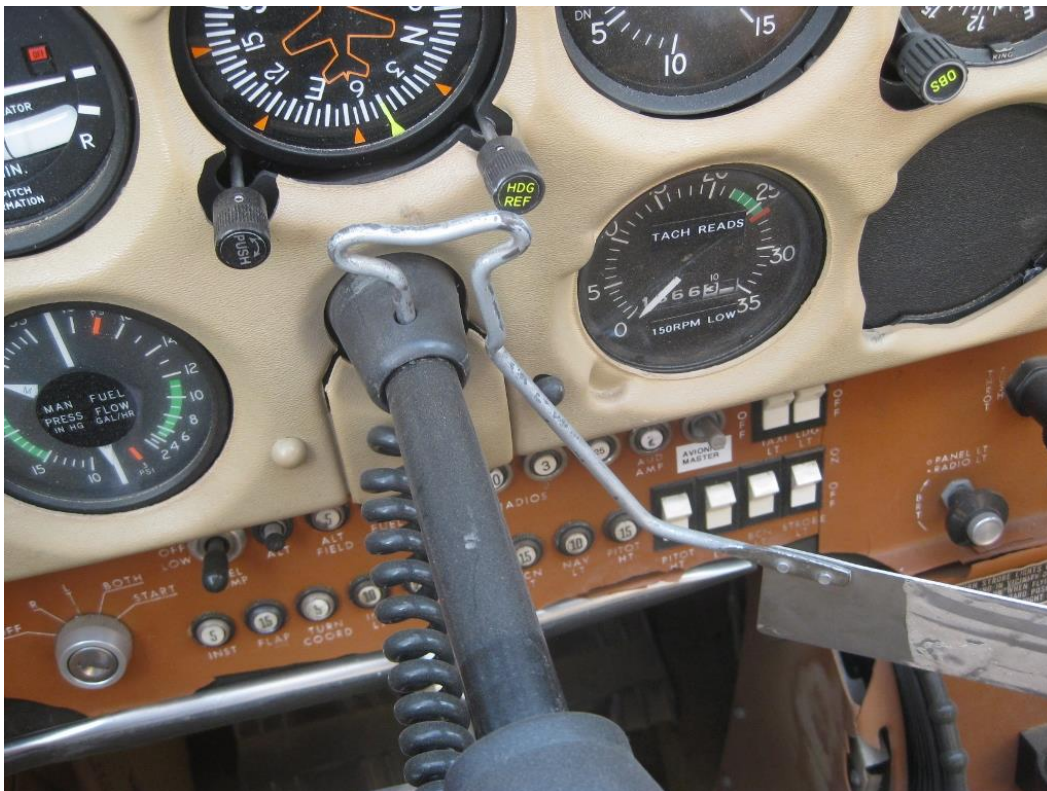
Figure 4 - Control Lock as Found (reversed installation)
