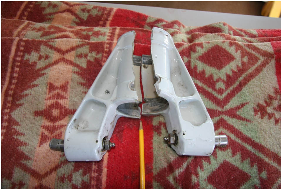
Figure 4: Left Landing Gear Upper Trunnion
