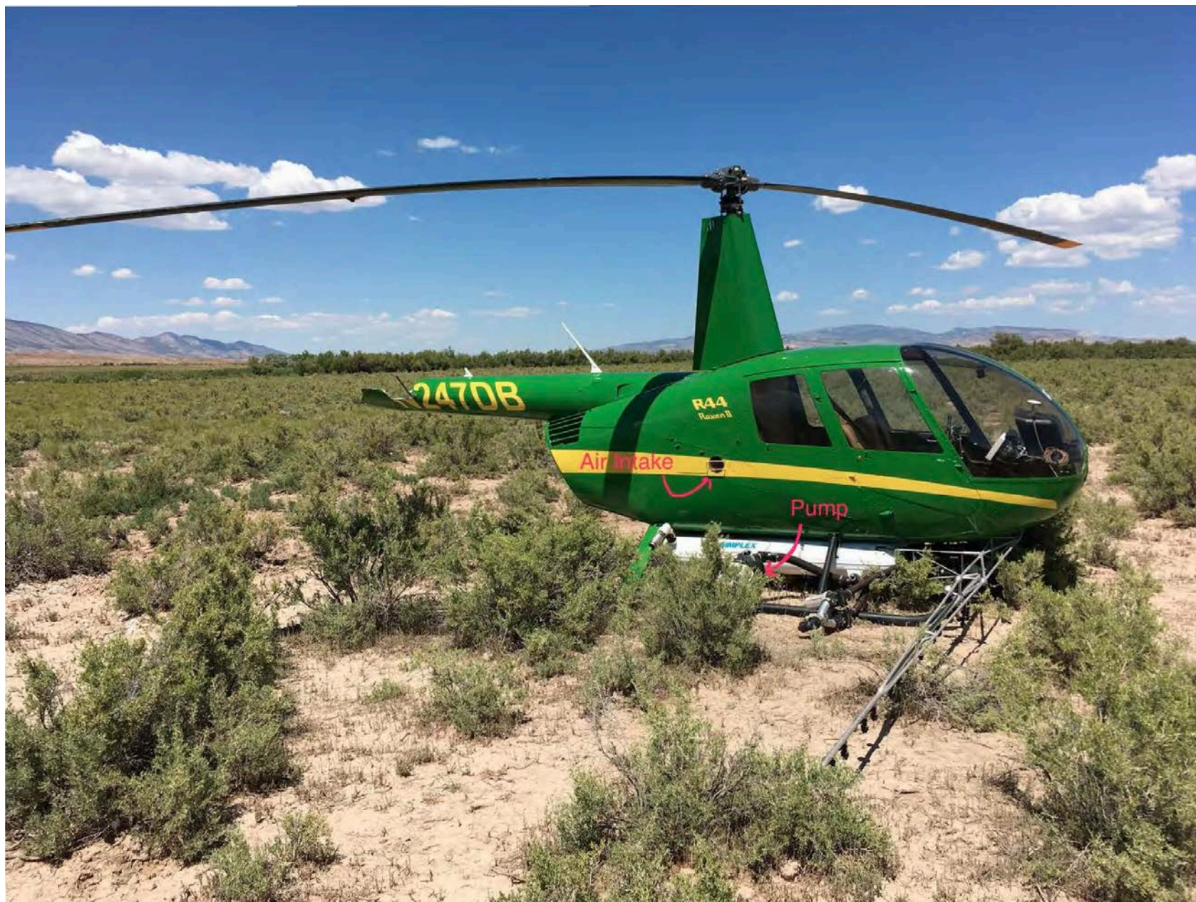
Photo 3 – View of pump location to air intake.
