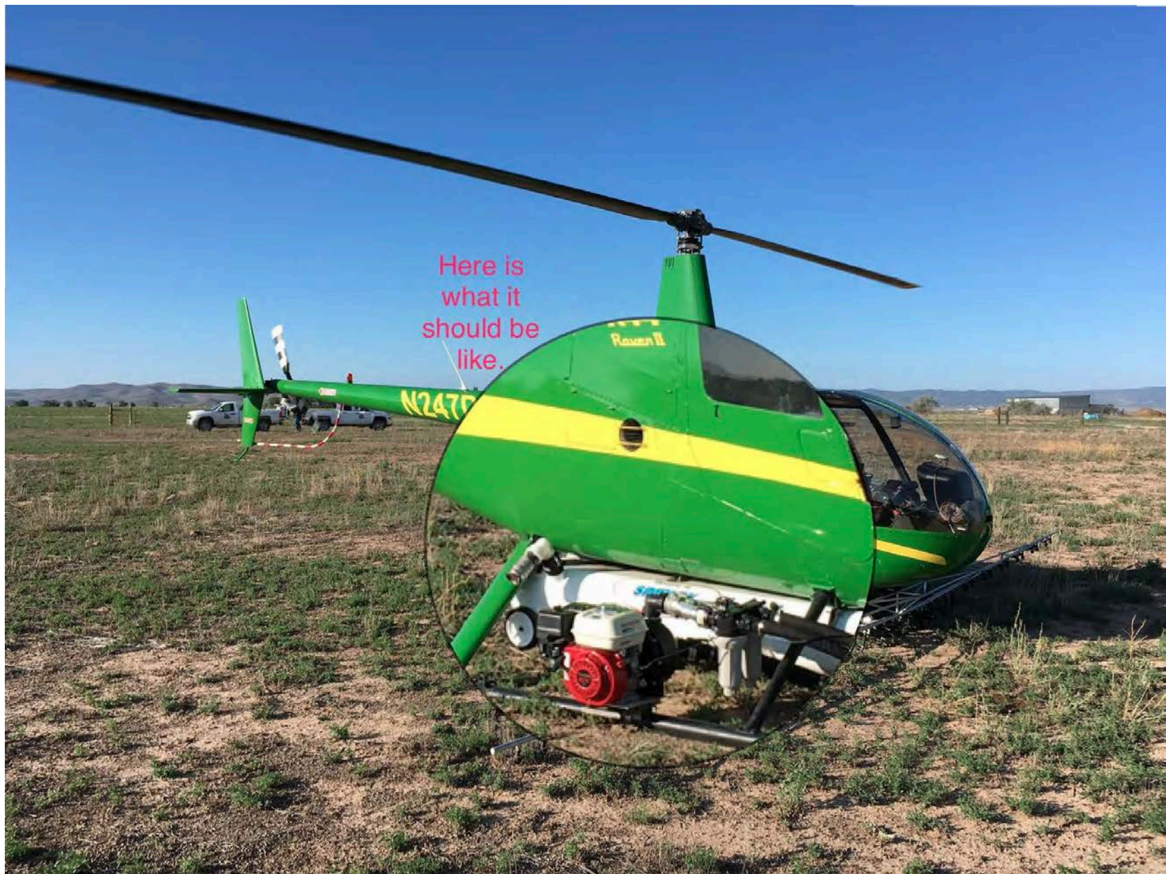
Photo 2 – Close up of intact Simplex pump system.
