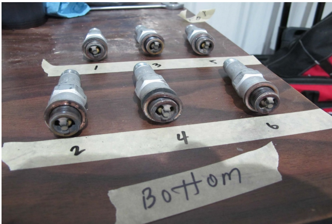
Figure 4 Bottom Spark Plugs
