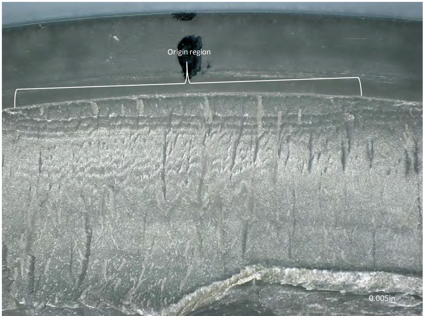
Figure 12 Digital microscope image of the origin region as identified in Figure 10.
