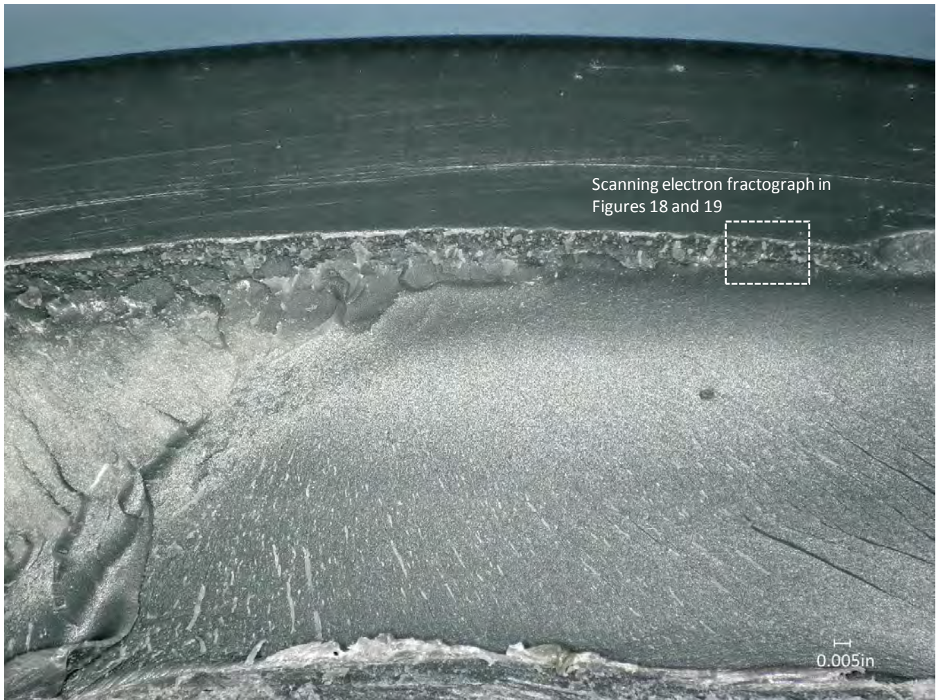
Figure 13 Digital microscope image of a region with incipient craze fracture features as identified in Figure 10
