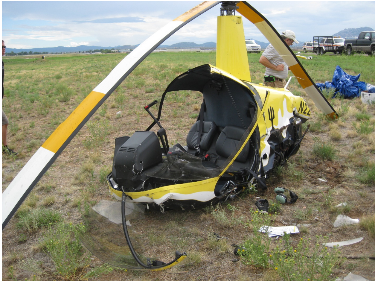
Figure 3 Front view of helicopter with damaged main rotor blades
