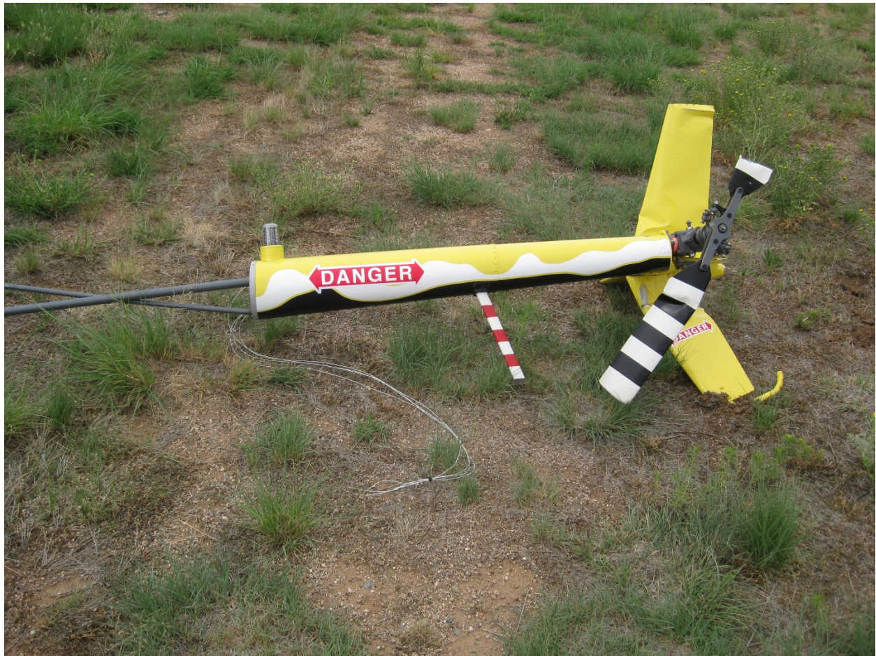
Figure 2 Severed tail boom
