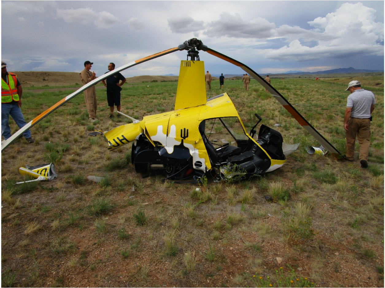
Figure 1 Side view of structural frame damage to helicopter
